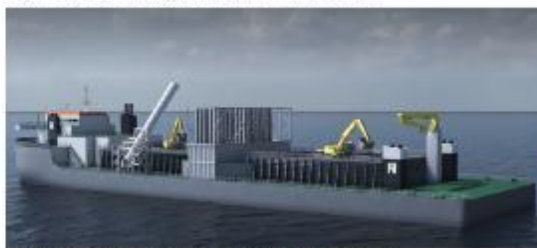
Figure 2 Placement of rock for pipe and cable crossings
