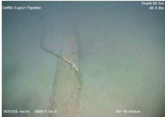
Image 1. Partially buried section of the GEP
