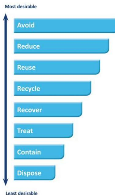
**Figure 11-2: Waste management hierarchy from the Project Waste Management Plan**
