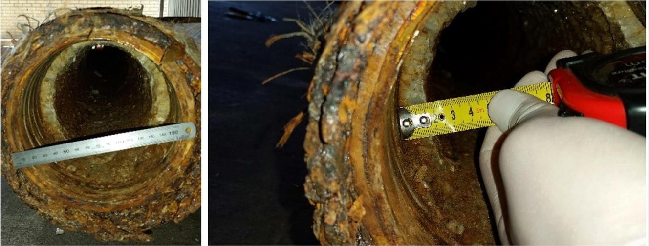
**Figure 3-8: Griffin 4 Flowline with Scale Built-up**
