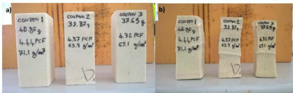
Figure 3-6: Images of 71 kg/m<sup>3</sup> foam coupons (a) before and (b) after small scale hydrostatic testing
