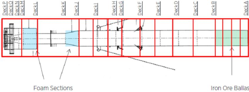
The diagram shows a longitudinal section of the RTM structure, divided into 15 vertical sections labeled Deck P through Deck A from left to right. Two sections, Deck L and Deck K, are highlighted in light blue and labeled 'Foam Sections'. A section at the far right, Deck A, is highlighted in light green and labeled 'Iron Ore Ballast'. Arrows point from the labels below to the corresponding sections in the diagram.
