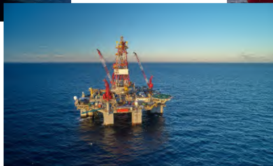
Semi-Submersible 50-1000+m Water Depth
