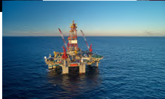
Semi-Submersible 50-1000+m Water Depth
