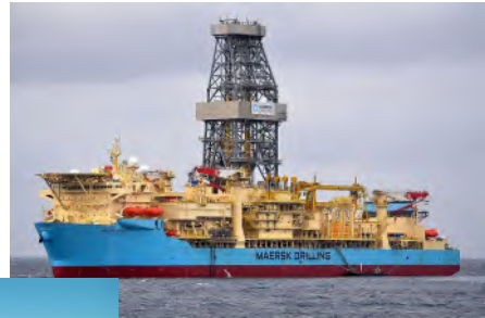
Drill Ship 600-3000+m Water Depth
