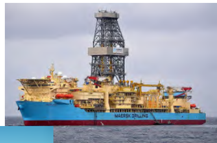
Drill Ship 600-3000+m Water Depth
