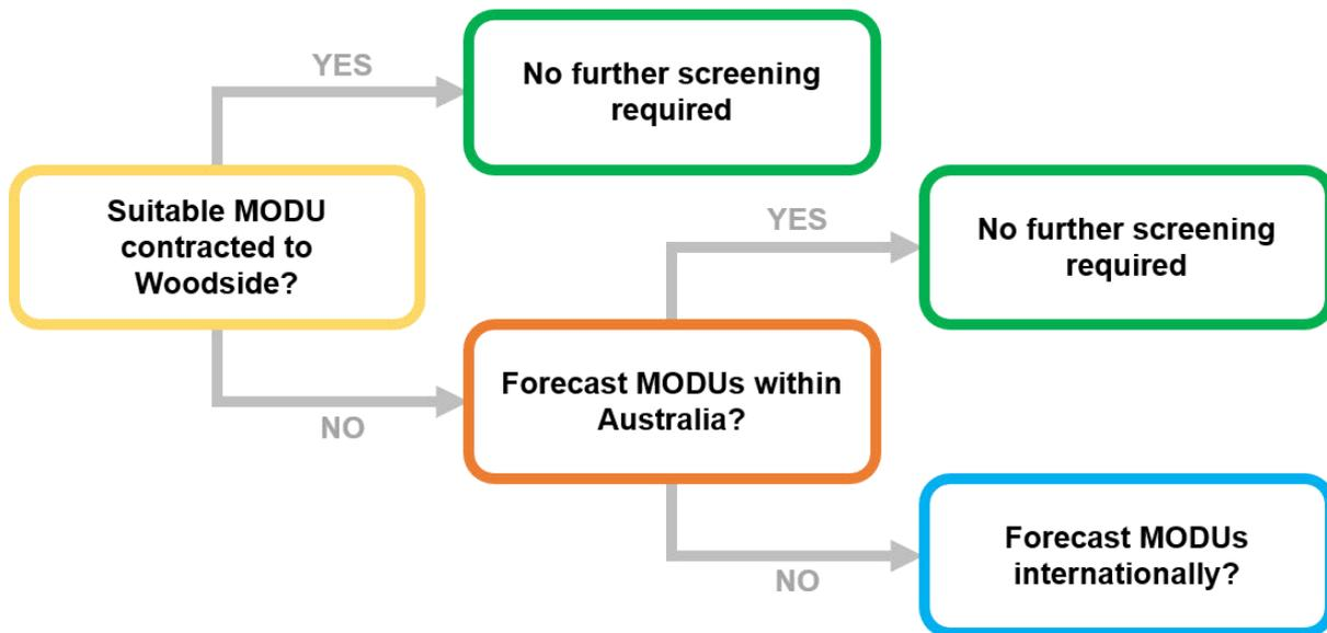
**Figure 6-1: PLA08 process for sourcing relief well MODU**
