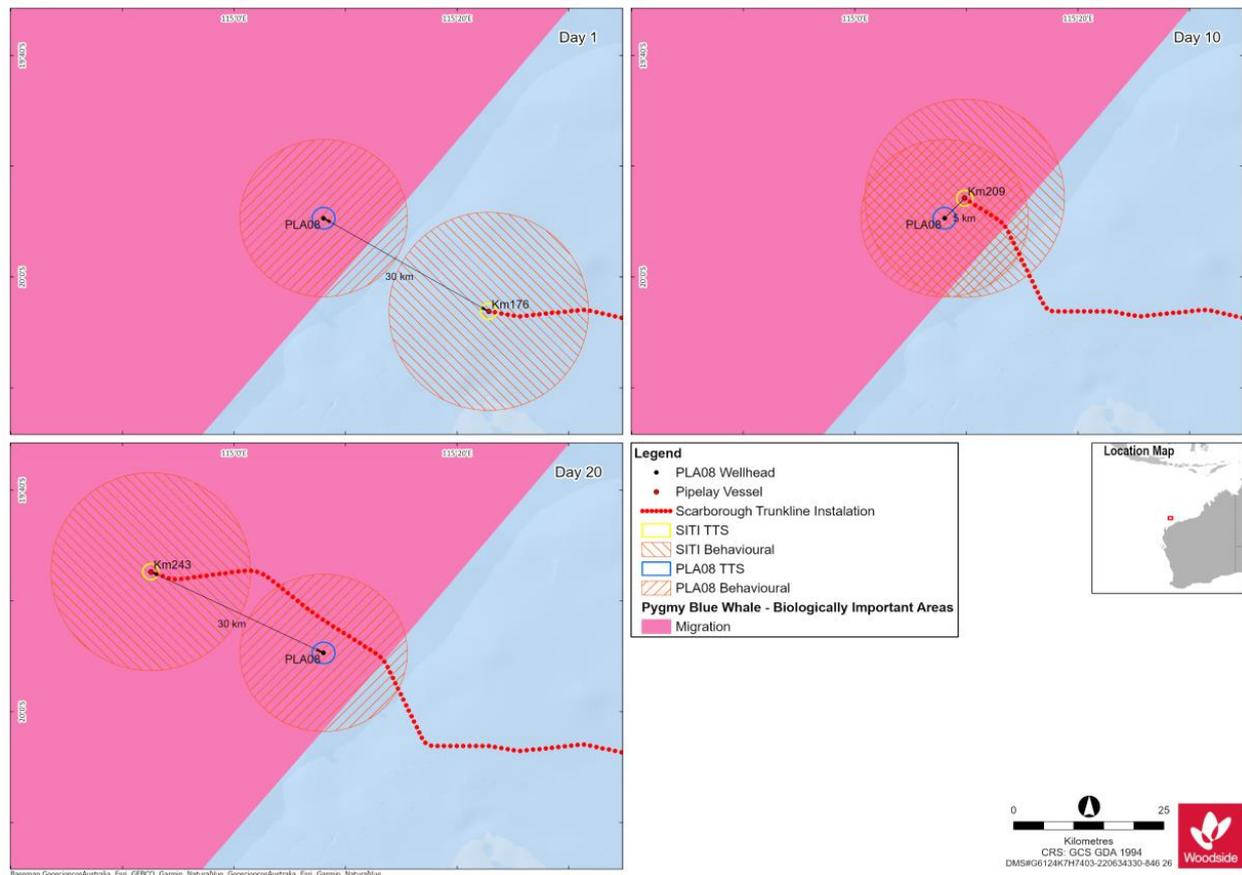
**Figure 6-1:** Illustrative figure showing overlap in sound fields between a dP MODU drilling at PLA08 Drilling while the Scarborough Trunkline Installation activities pass in close proximity.
