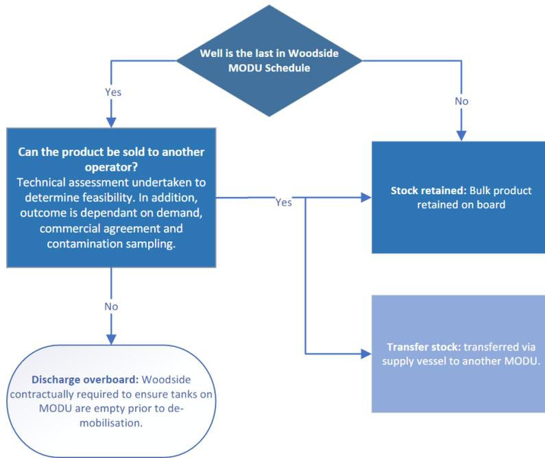
**Figure 6-2 Management process for excess bulk product**
