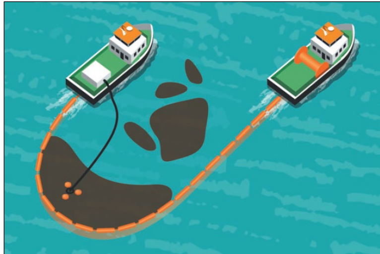
Figure 11-1: 'J' Configuration for Containment & Recovery Operations; 1 x Containment and Recovery Unit (IPIECA-IOGP, 2016a)
