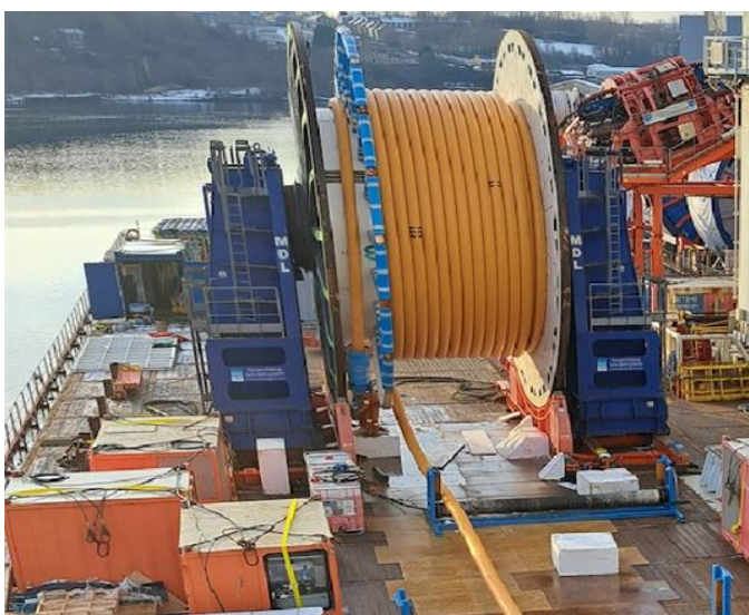
Figure 3-5: Flowline reel with reel hub drive system engaged
