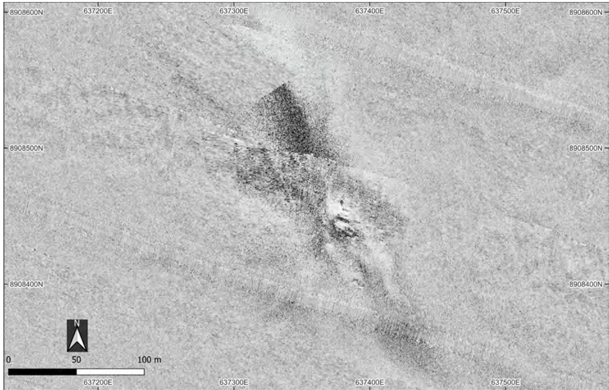
Figure 12: Example of SSS data collected by DOF Subsea in 2018 survey. Note, image on SSS is believed to be location of exploratory well drilling, therefore it is not a listed target.
