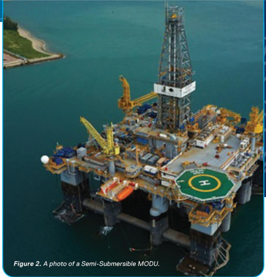
Figure 2. A photo of a Semi-Submersible MODU.
