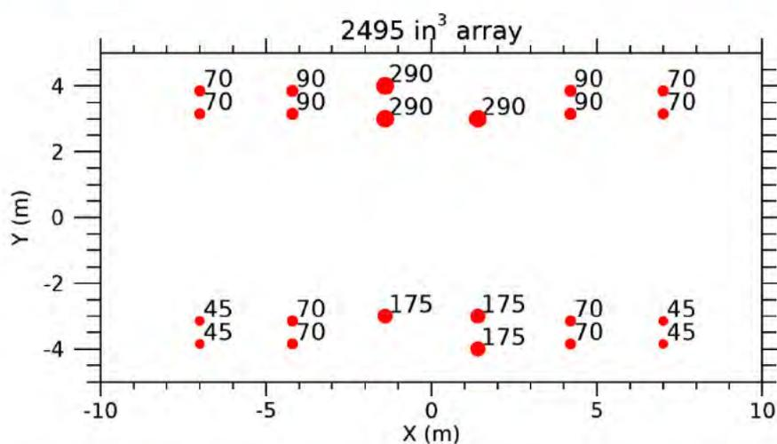
Figure B-1. Layout of the modelled 2495 in<sup>3</sup> array. Tow depth is 6 m. The labels indicate the firing volume (in cubic inches) for each airgun. Also see Table B-1.
