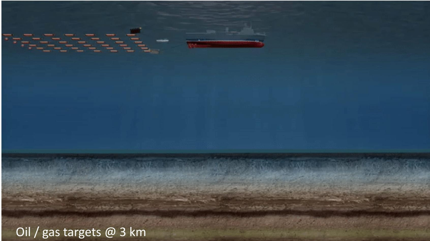
Sound waves (air) sent into earth by towed source, reflect off rock layers and reflections measured back at surface by “hydrophones” towed at shallow depths of < 10 metres by boat
