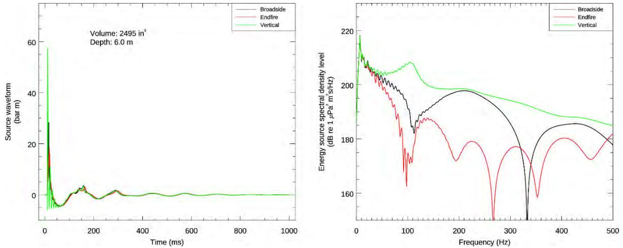
Figure B-2. Predicted source level details for the 2495 in<sup>3</sup> seismic source with a 6 m towed depth. (Left) the overpressure signature and (right) the power spectrum for in-plane horizontal (broadside), perpendicular (endfire), and vertical directions (no surface ghost).
