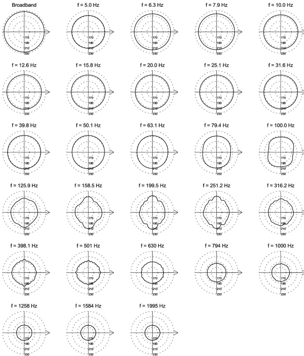
Figure B-3. Directionality of the predicted horizontal source levels for the 2495 in<sup>3</sup> seismic source, 5 Hz to 2 kHz. Source levels (in dB re 1  $\mu\text{Pa}^2\cdot\text{s}^2$ ) are shown as a function of azimuth for the centre frequencies of the decade bands modelled; frequencies are shown above the plots. The perpendicular direction to the frame is to the right. Tow depth is 6 m.
