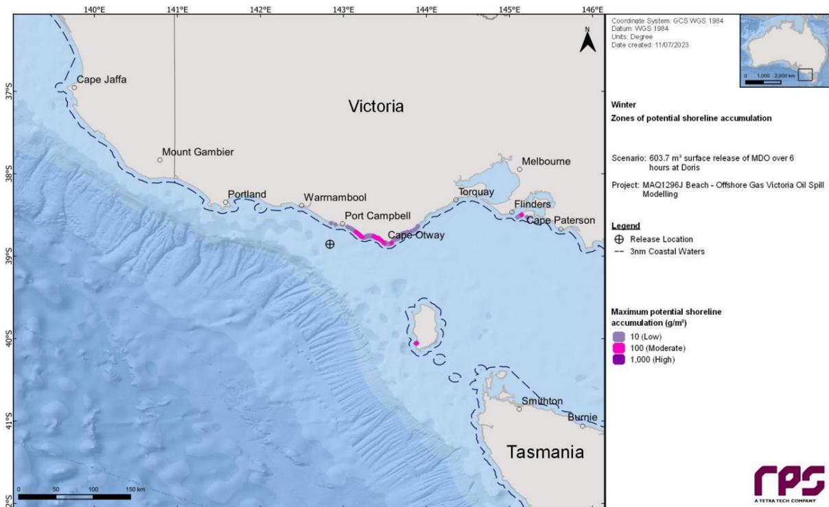
Figure 4-8: 603.7 m<sup>3</sup> Vessel spill (MDO) Actionable Response Areas Otway Basin (Doris Field) Winter (RPS APASA 2023)
