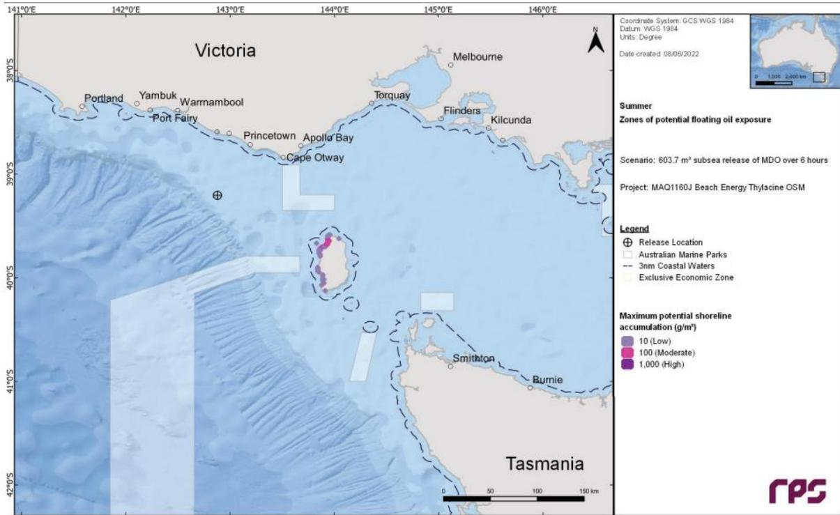
Figure 4-3: 603.7 m<sup>3</sup> Vessel spill (MDO) Actionable Response Areas Otway Basin (Thylacine Field) Summer (RPS APASA, 2022)
