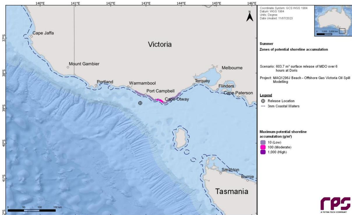
Figure 4-7: 603.7 m<sup>3</sup> Vessel spill (MDO) Actionable Response Areas Otway Basin (Doris Field) Summer (RPS APASA 2023)
