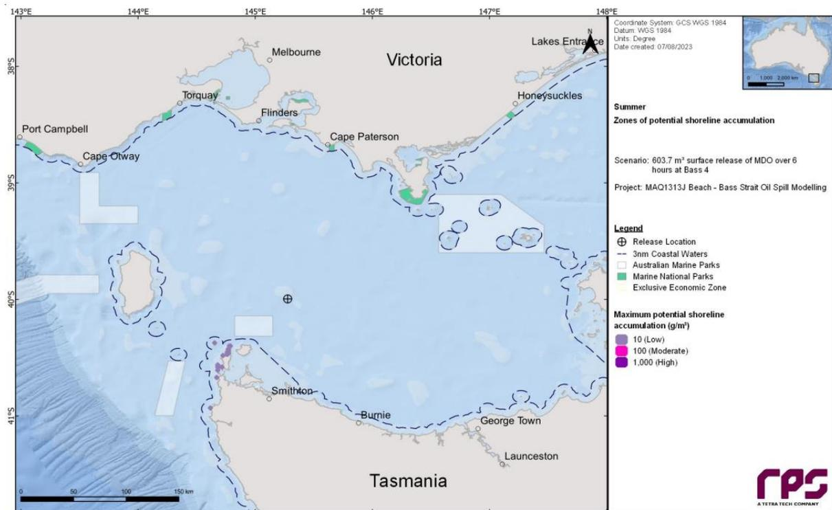
Figure 4-17: 603.7 m<sup>3</sup> Vessel Spill (MDO) Actionable Response Areas Bass Basin Summer (RPS, 2023)
