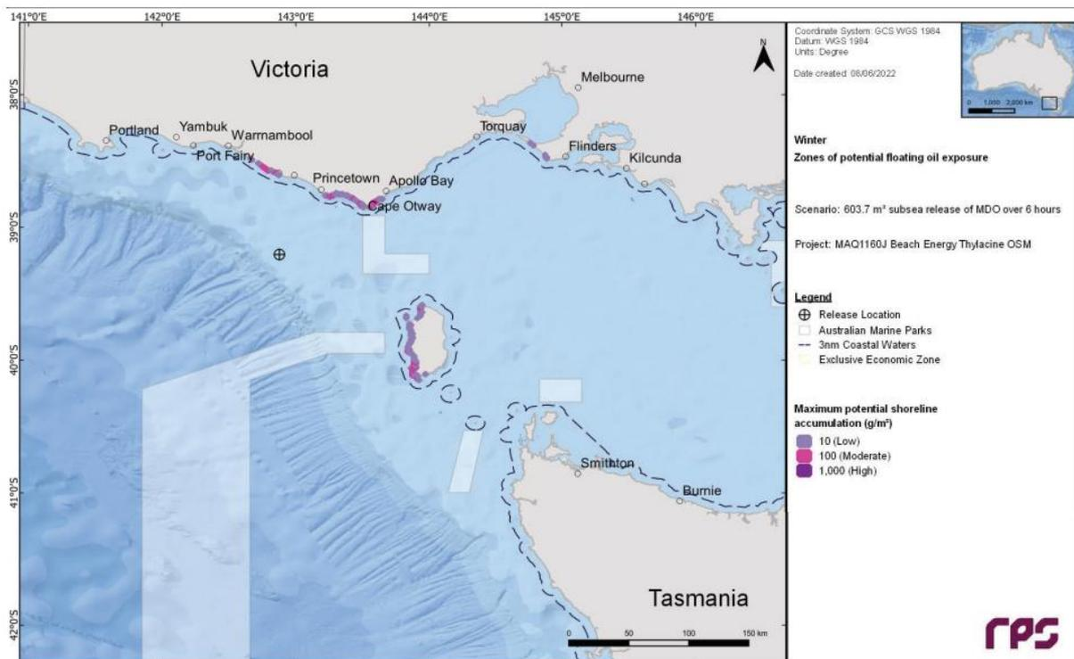
Figure 4-4: 603.7 m<sup>3</sup> Vessel spill (MDO) Actionable Response Areas Otway Basin (Thylacine Field) Winter (RPS APASA, 2022)
