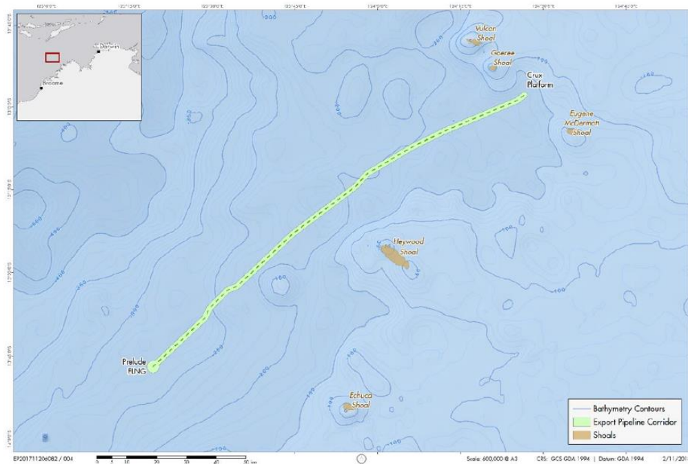
Figure 7-29: Crux pipeline corridor
