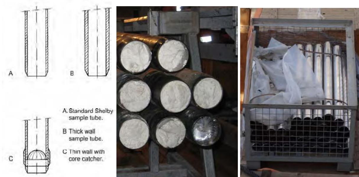
Figure 3-9: Examples of a geotechnical piston core sample tubes
