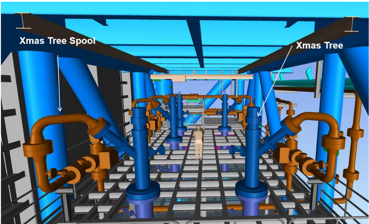
Figure 6-31: Dry Xmas Tree and Tie-in Spool Example
