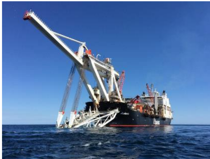
Figure 6-2: Indicative Pipelay Vessel (Audacia)
