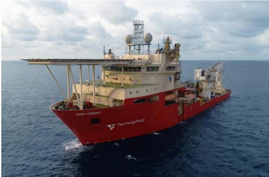
Figure 6-7: Indicative Flexible Pipelay Vessel (Deep Orient)
