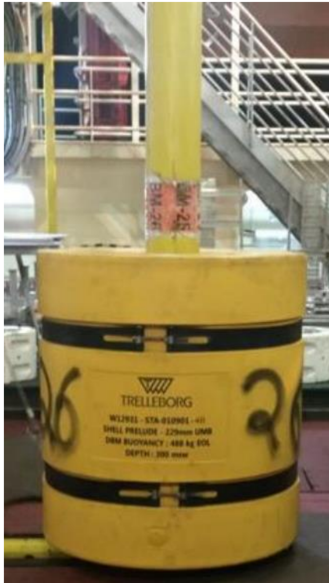
Figure 6-12: Example of a Buoyancy Module
