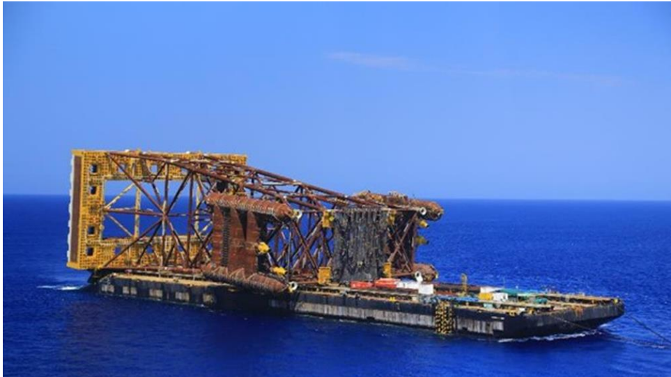
Figure 6-5: Indicative Substructure Transportation Barge (I650)
