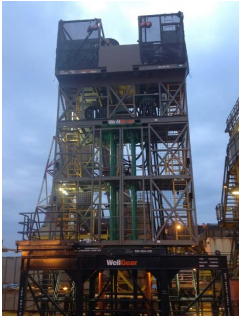
Figure 6-29: Indicative Hydraulic Workover Unit
