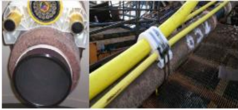
Figure 1. Minerva Pipeline Bundle Arrangement
