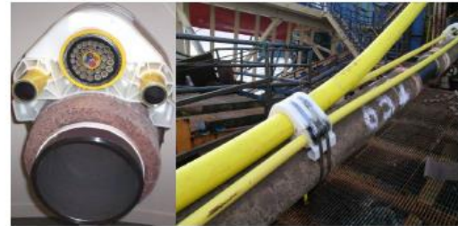
Figure 2. Minerva Pipeline Bundle Arrangement
