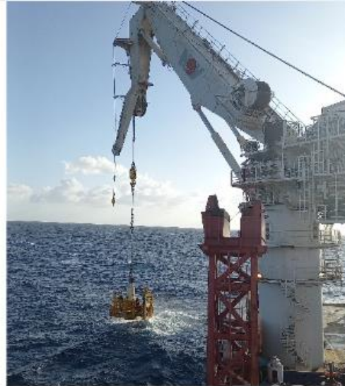
Figure 3. Typical Subsea Equipment Recovery Activity
