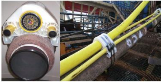
Figure 1. Minerva Pipeline Bundle Arrangement
