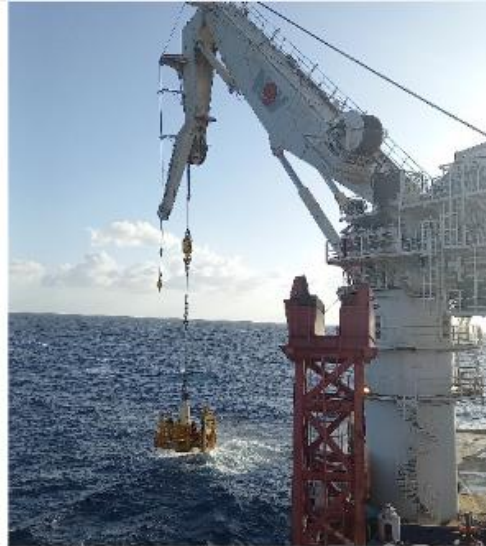
Figure 3. Typical Subsea Equipment Recovery Activity
