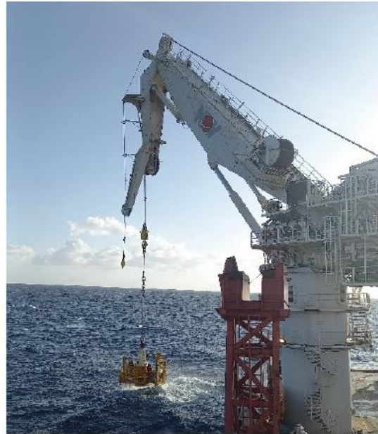
Figure 3. Typical Subsea Equipment Recovery Activity
