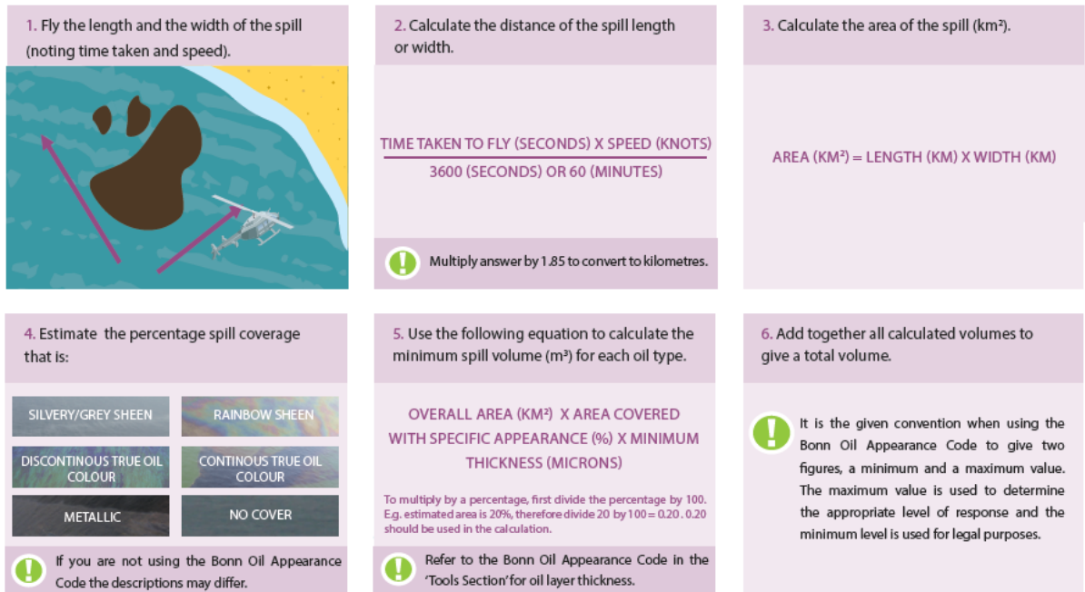
Figure 4.2: Spill quantification procedure (OSRL, 2016)
