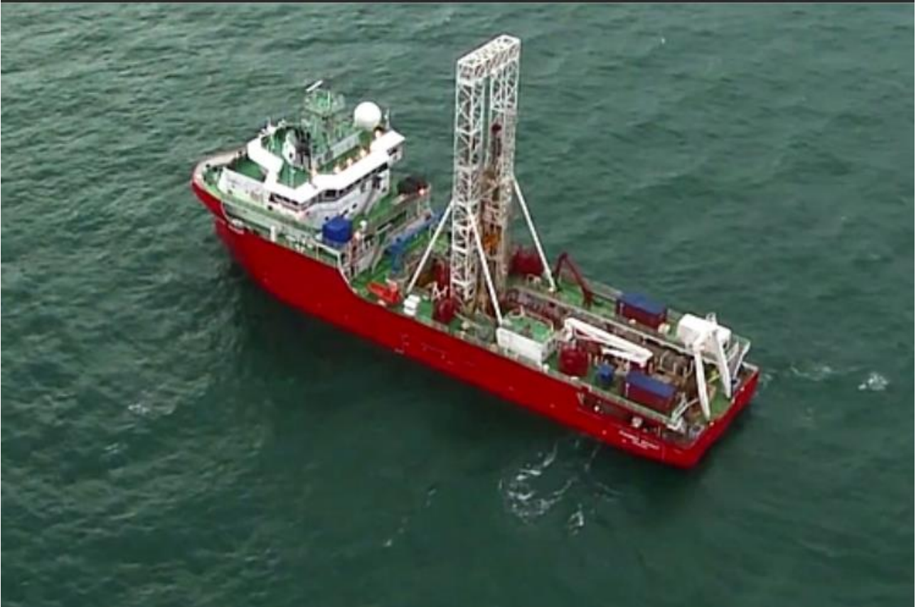
Figure 3-2: Typical geotechnical investigation vessel
