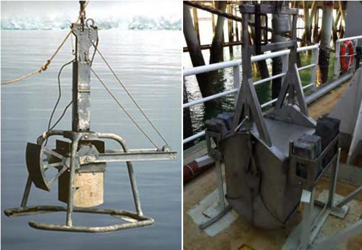
Figure 3-10: Examples of box core samplers
