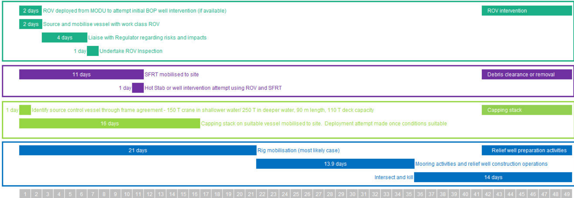
Figure 6-2: Source control and well intervention response strategy deployment timeframes for J85 Development Well
