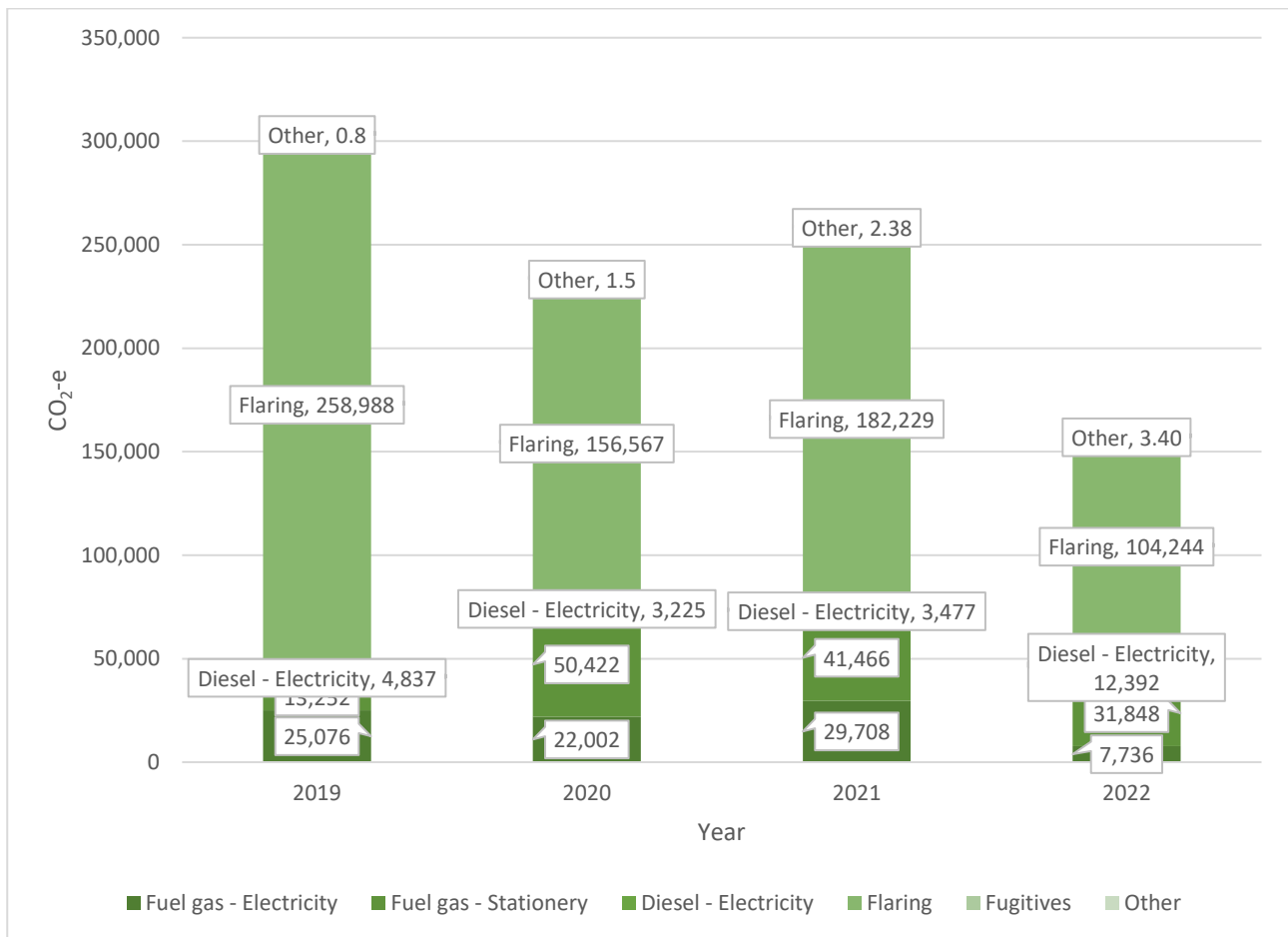
Figure 7-1: GHG emissions due to combustion sources at Montara Facility in 2019–2022 (CO 2 -e)
