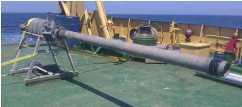
**Photo 2-12 Typical gravity corer**
