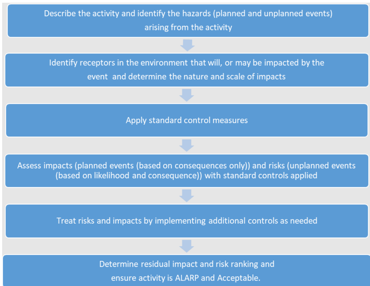
Figure 5-1: Hazard identification and assessment guideline
