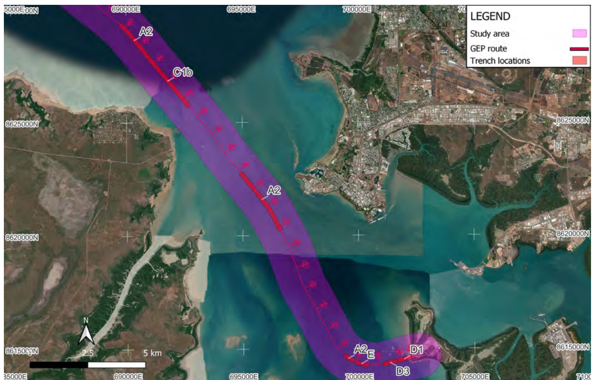
Figure 102: Map of proposed trenching locations with trench type labelled. (Polygons for trench locations are indicative of location only, not to scale by width).
