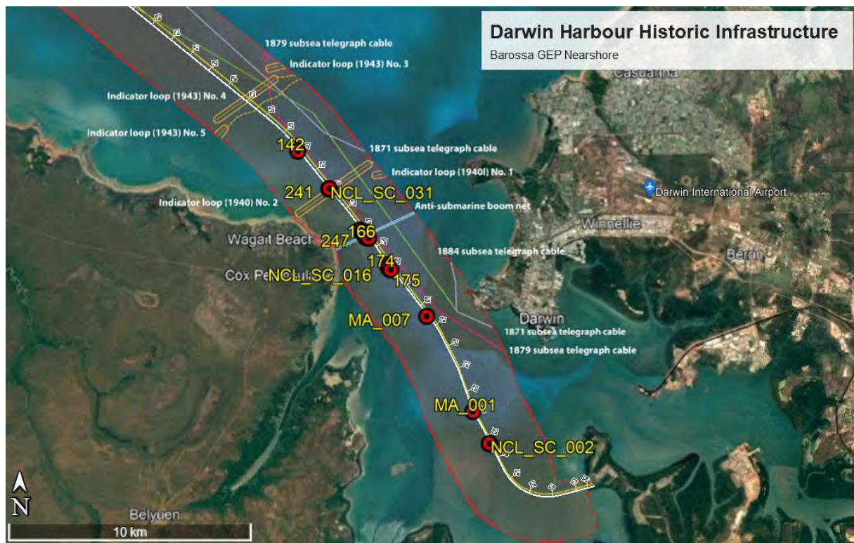
Figure 70: ROV survey shortlisted target locations overlaid on map of known historic maritime infrastructure in Darwin Harbour.
