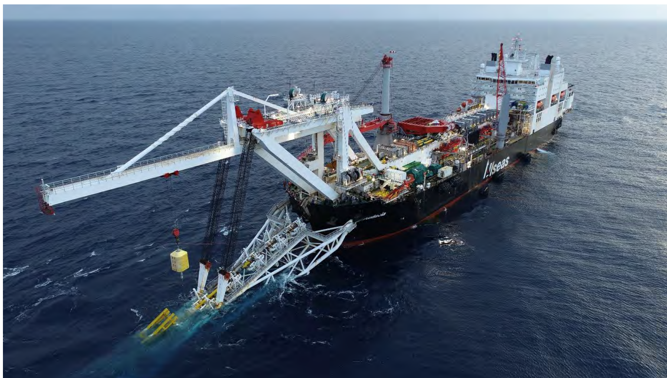
Figure 2-3: Indicative pipelay vessel ( Audacia )
