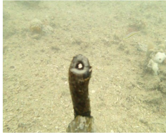
Figure 52: Cross section of broken communication cable. (Source: CA 2012).
