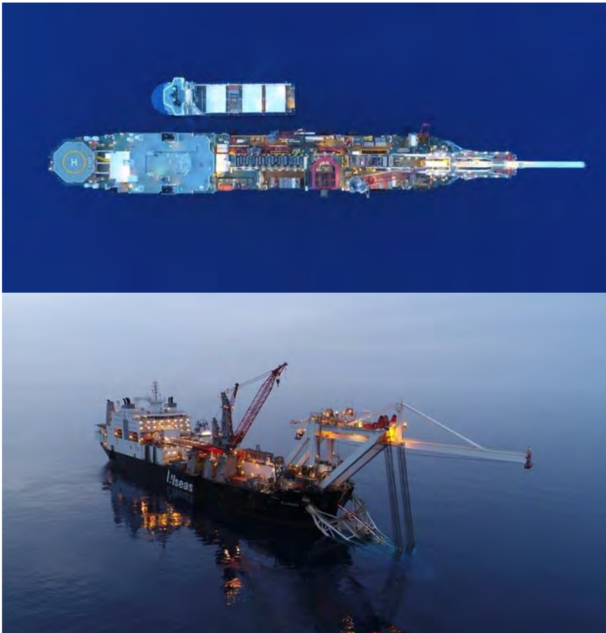
Figure 6-1: Photographs of a typical pipelay vessel at dusk
