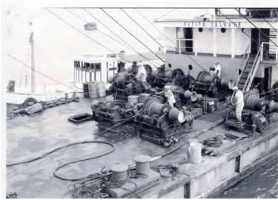
Figure 92: "Winches on the deck of Fujita Salvage Boat." Note bollard at bottom of picture. 116
