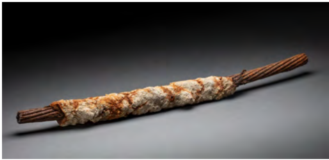
Figure 27: Section of the 1871 Darwin to Java subsea telegraph cable recovered from Timor Sea in 2016. 76
