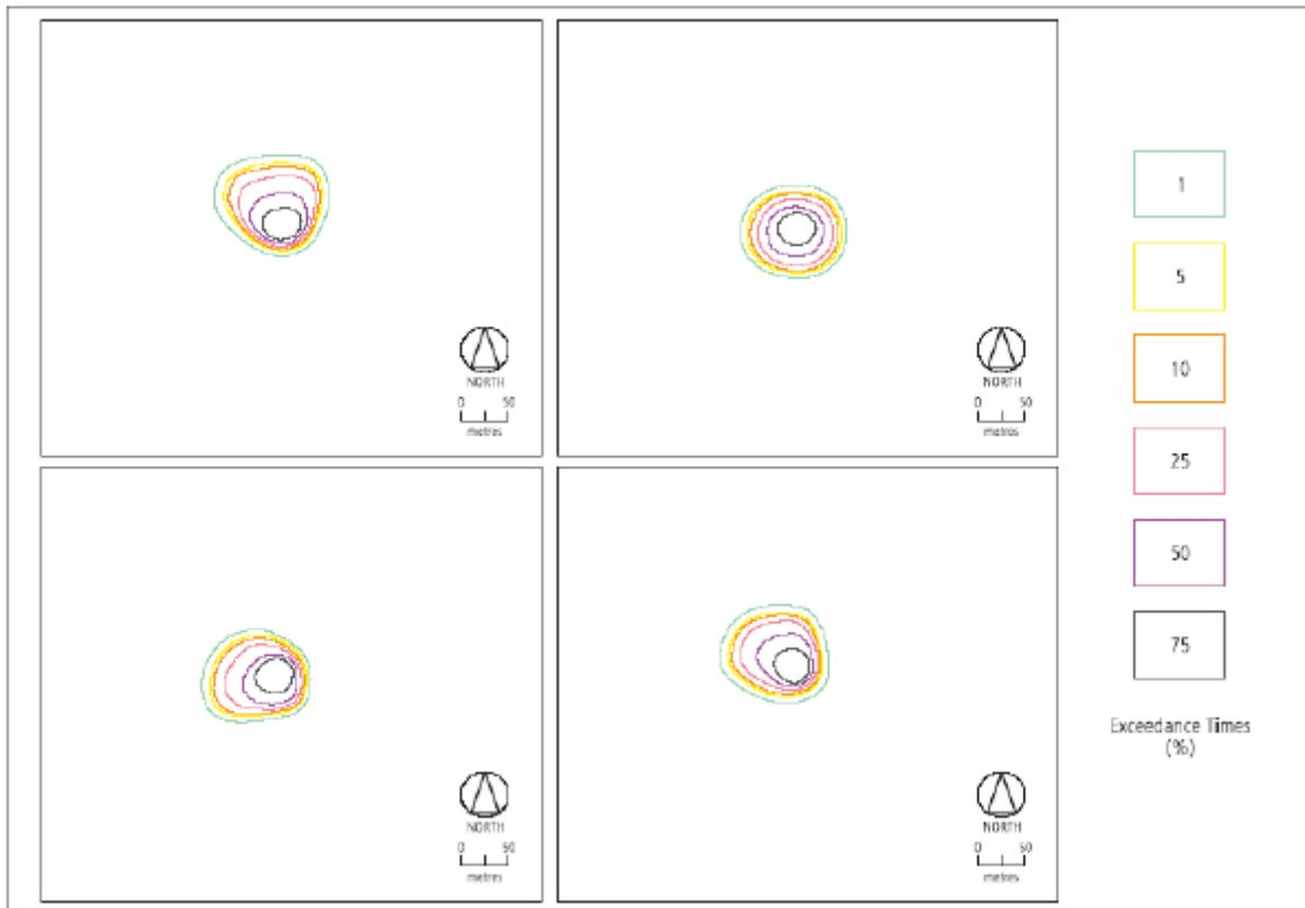
**Figure 6-5 Predicted dispersion and temperature of cooling water discharge (trajectory and dispersion of cooling water modelled for a nominal discharge of 100,000 m<sup>3</sup> at a water temperature of 25°C above surrounding seawater.**
