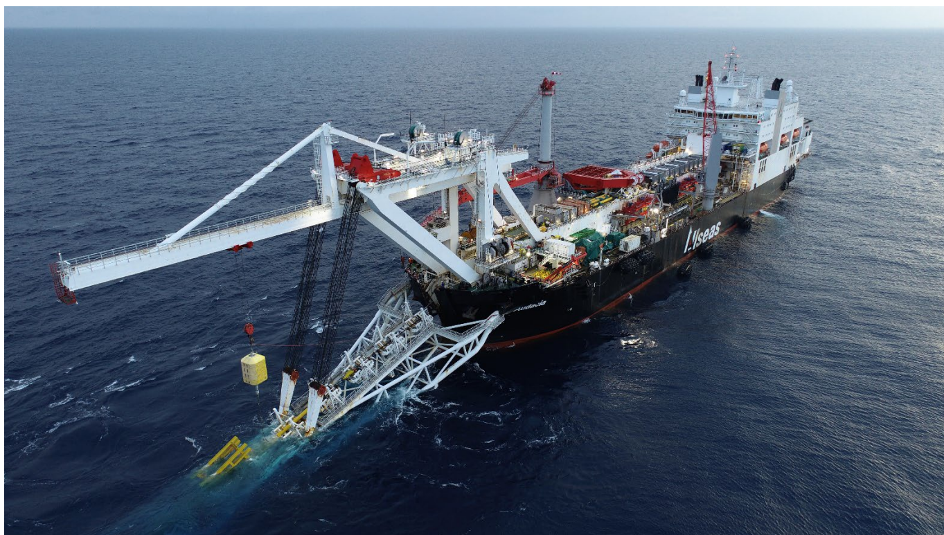
Figure 2-3: Indicative pipelay vessel ( Audacia )
