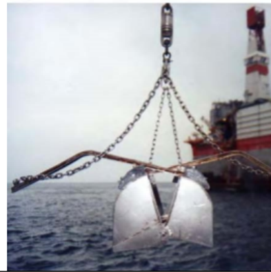
Figure M.9.1 Deployment of Spring-loaded Grab Sampler (Photo: Sakhalin Energy Investment Company)
