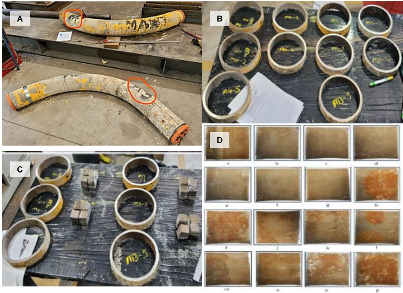
Figure 3-3: 8” production spool pieces (A), rings cut from spool pieces (B and C) and coupons cut from rings (D)
