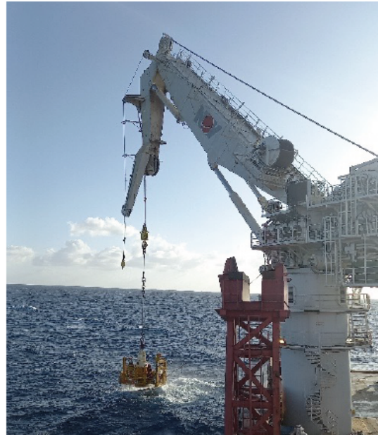
Figure 3. Typical Subsea Equipment Recovery Activity
