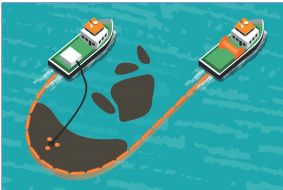
Figure 11-1: 'J' Configuration for containment and recovery operations; 1 containment and recovery unit (IPIECA-IOGP, 2016a)
