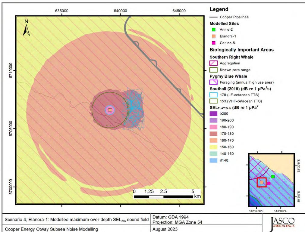
Figure 31. Scenario 4, Drilling and standby OSV, Elanora-1, accumulated SEL<sub>24h</sub>: Sound level contour map showing weighted maximum-over-depth SEL<sub>24h</sub> results, along with isopleths for TTS in low and very-high-frequency cetaceans. Thresholds omitted here were not reached or not long enough to display graphically.
