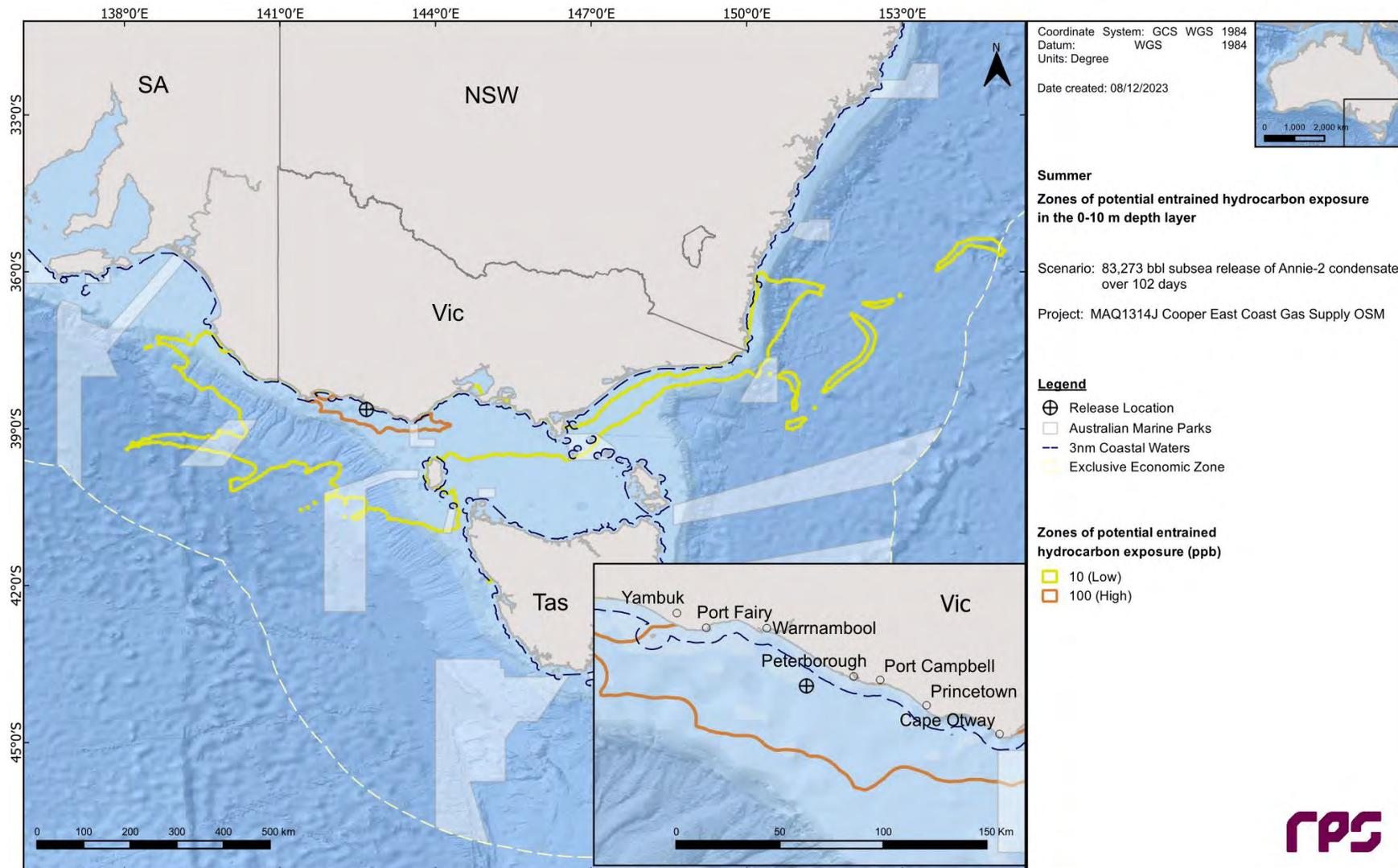
**Figure 12.13** Zones of potential entrained hydrocarbon exposure at 0-10 m below the sea surface in the event of an 83,273 bbl subsurface release from a loss of well control at Pecten East-2 over 102 days. The results were calculated from 100 spill simulations during summer conditions.
