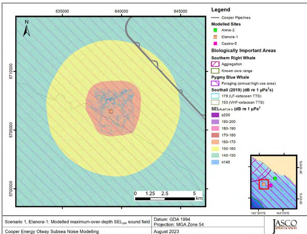
Figure 25. Scenario 1, Drilling Prelays, Elanora-1, accumulated SEL<sub>24h</sub>: Sound level contour map showing weighted maximum-over-depth SEL<sub>24h</sub> results, along with isopleths for TTS in low and very-high-frequency cetaceans. Thresholds omitted here were not reached or not long enough to display graphically.
