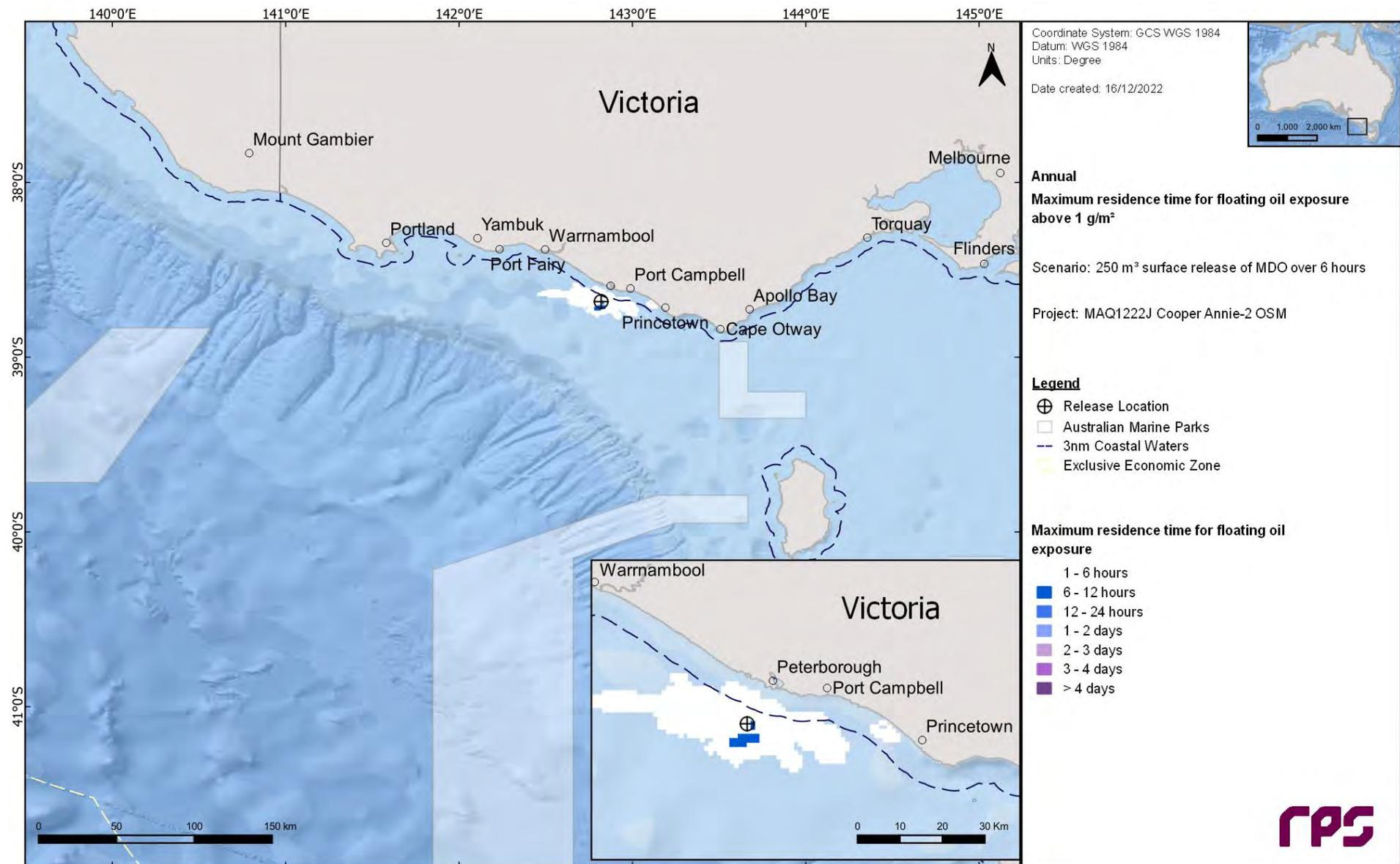
**Figure 10.3** Maximum residence time of floating oil exposure above 1 g/m<sup>2</sup>, in the event of a 250 m<sup>3</sup> of MDO containment loss over 6 hours tracked for 30 days. The results were calculated from 100 spill simulations.
