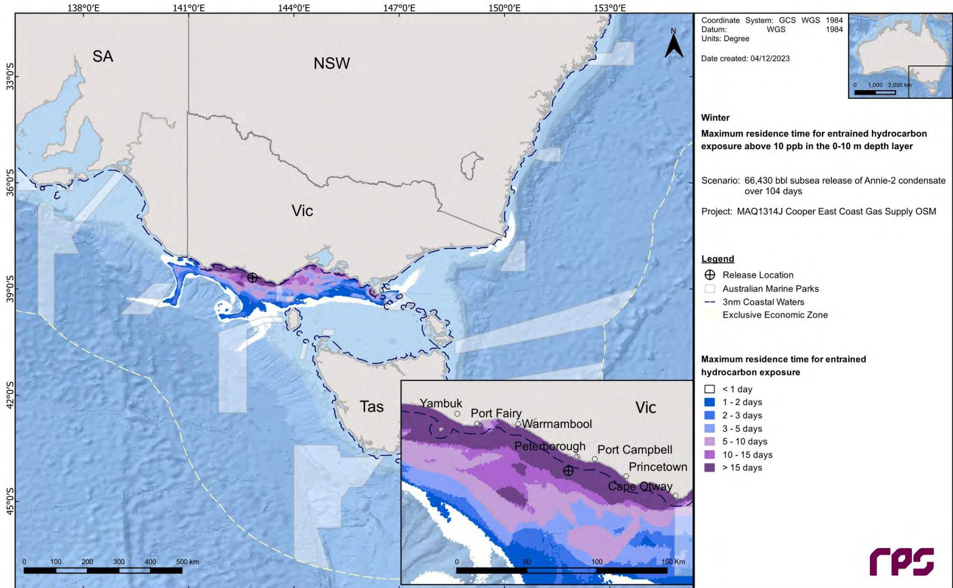
**Figure 13.16** Maximum residence time for entrained hydrocarbon exposure above 10 ppb, at 0-10 m below the sea in the event of a 66,430 bbl subsurface release from a loss of well control at Annie-2 over 104 days. The results were calculated from 100 spill simulations during winter conditions.
