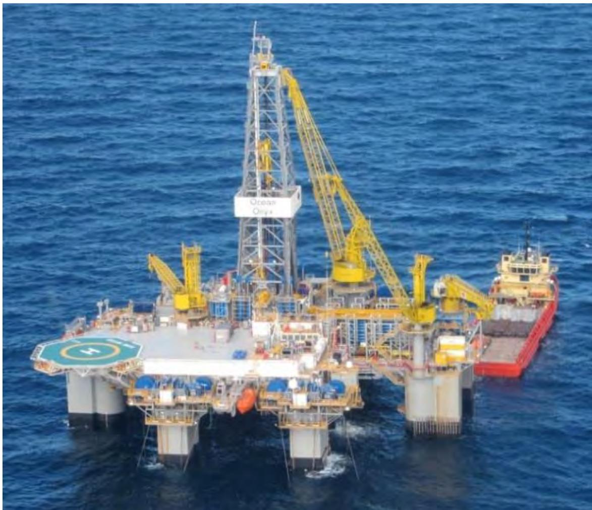
Figure 3. *Ocean Onyx* semi-submersible platform.
