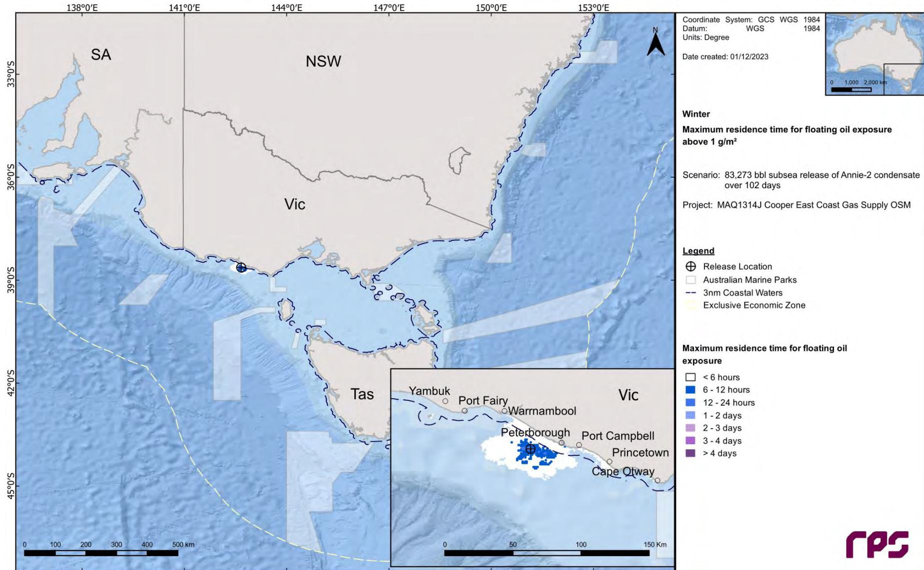
Figure 12.4 Maximum residence time of floating oil exposure above 1 g/m<sup>2</sup>, in the event of an 83,273 bbl subsurface release from a loss of well control at Pecten East-2 over 102 days. The results were calculated from 100 spill simulations during winter conditions.
