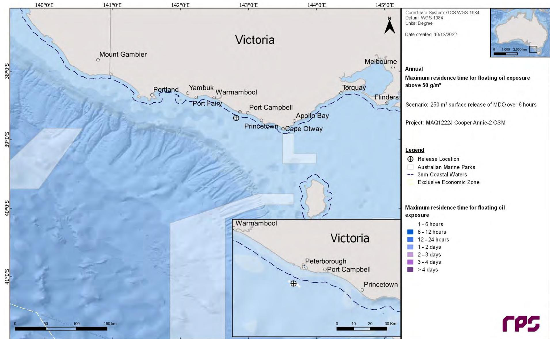
**Figure 10.5** Maximum residence time of floating oil exposure above 50 g/m<sup>2</sup>, in the event of a 250 m<sup>3</sup> of MDO containment loss over 6 hours tracked for 30 days. The results were calculated from 100 spill simulations.
