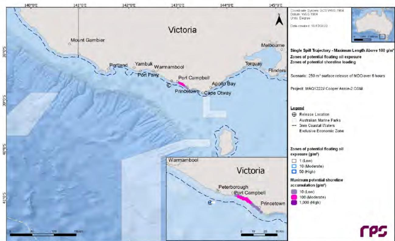
**Figure 10.19 Zones of potential floating oil exposure and shoreline accumulation, for the trajectory with the largest volume ashore and longest length of shoreline with accumulation above 100 g/m<sup>2</sup>. Results are based on a 250 m<sup>3</sup> surface release of MDO over 6 hours, tracked for 30 days.**
