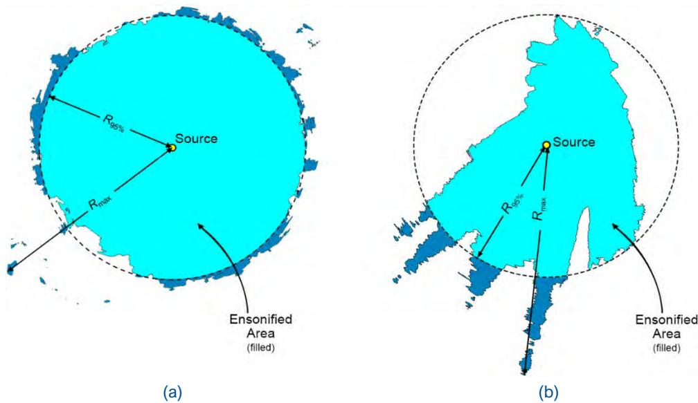
Figure B-5. Sample areas ensonified to an arbitrary sound level with  $R_{\max}$  and  $R_{95\%}$  ranges shown for two different scenarios. (a) Largely symmetric sound level contour with small protrusions. (b) Strongly asymmetric sound level contour with long protrusions. Light blue indicates the ensonified areas bounded by  $R_{95\%}$ ; darker blue indicates the areas outside this boundary which determine  $R_{\max}$ .
