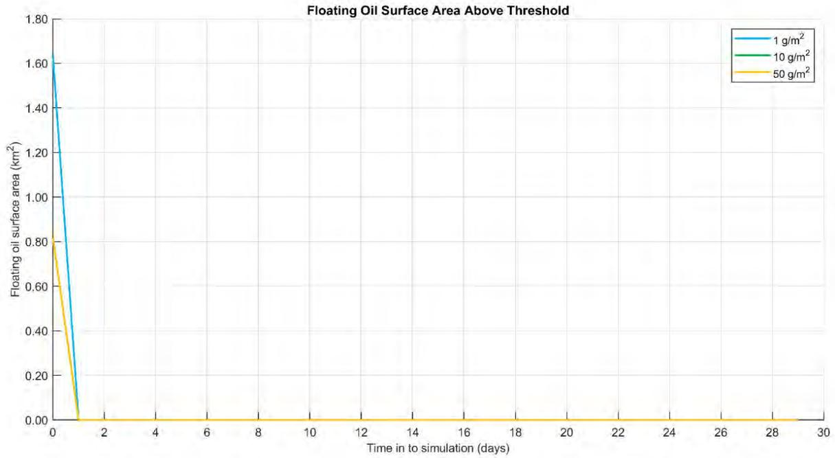
**Figure 10.17** Time series of the sea surface exposure above each threshold for the trajectory with the largest swept area of floating oil above 50 g/m<sup>2</sup>. Results are based on a 250 m<sup>3</sup> surface release of MDO over 6 hours, tracked for 30 days.
