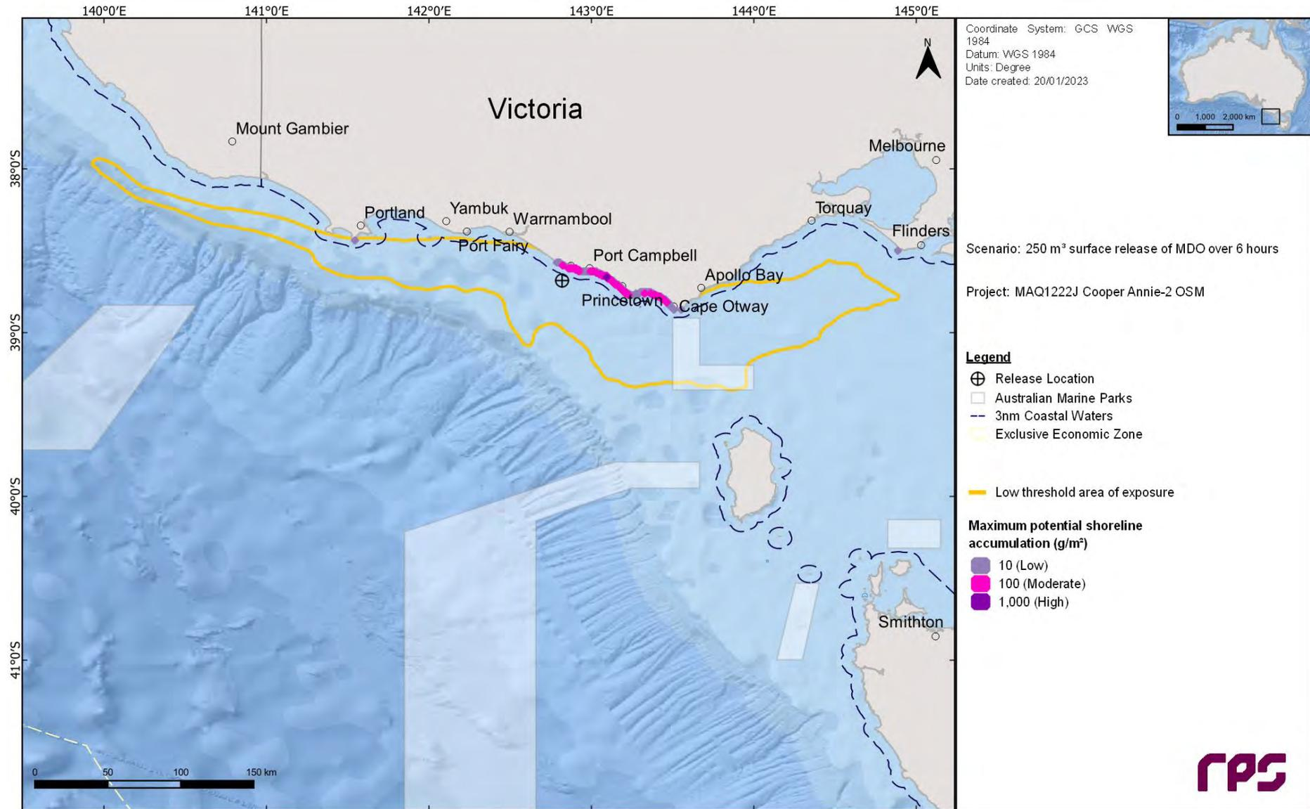
Figure 10.1 Predicted area of exposure for low thresholds produced by overlaying the results from 100 simulations of a 250 m<sup>3</sup> surface release of MDO over 6 hours.
