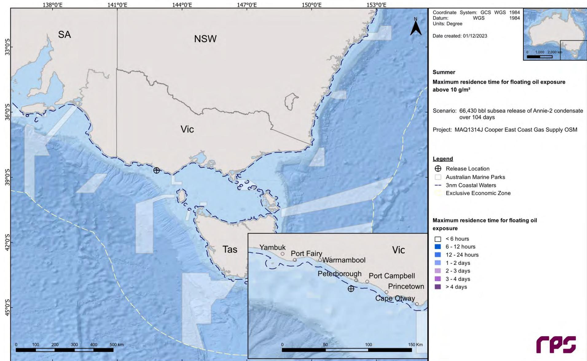
Figure 13.5 Maximum residence time of floating oil exposure above 10 g/m<sup>2</sup>, in the event of a 66,430 bbl subsurface release from a loss of well control at Annie-2 over 104 days. The results were calculated from 100 spill simulations during summer conditions.
