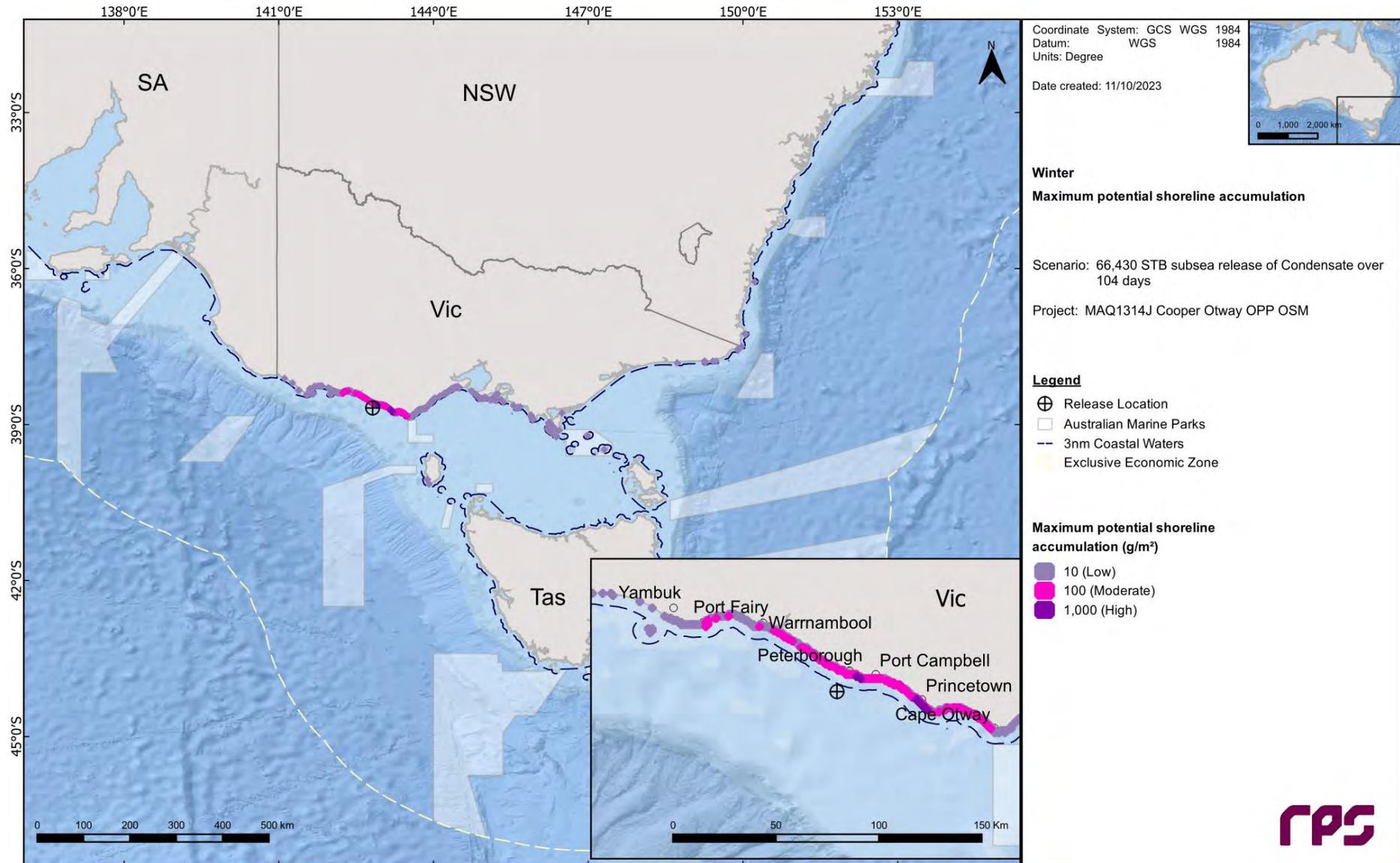
**Figure 13.8** Maximum potential shoreline accumulation in the event of a 66,430 bbl subsurface release from a loss of well control at Annie-2 over 104 days. The results were calculated from 100 spill simulations during winter conditions.
