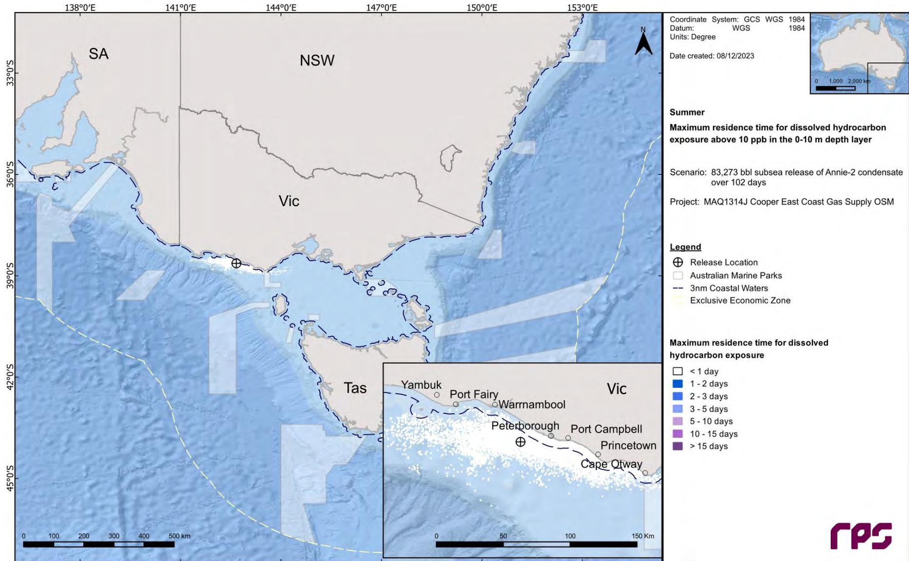
**Figure 12.11 Maximum residence time for dissolved hydrocarbon exposure above 10 ppb, at 0-10 m below the sea surface in the event of an 83,273 bbl subsurface release from a loss of well control at Pecten East-2 over 102 days. The results were calculated from 100 spill simulations during summer conditions.**
