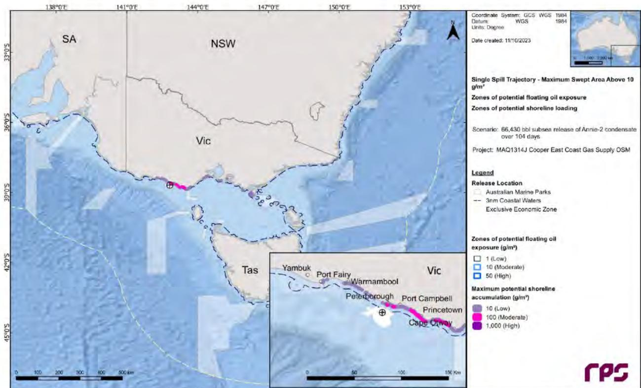
**Figure 13.19 Zones of potential floating oil exposure and shoreline accumulation, for the trajectory with the largest swept area of floating oil above 10 g/m<sup>2</sup>.**
