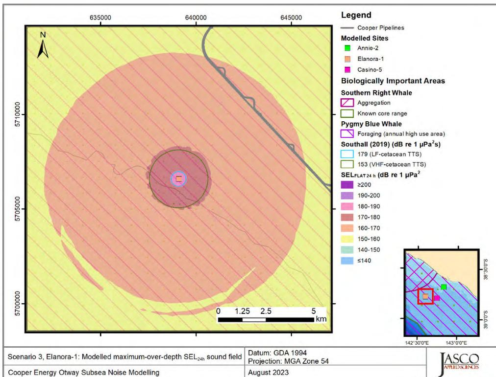
Figure 29. Scenario 3, MODU Drilling, Elanora-1, accumulated SEL<sub>24h</sub>: Sound level contour map showing weighted maximum-over-depth SEL<sub>24h</sub> results, along with isopleths for TTS in low and very-high-frequency cetaceans. Thresholds omitted here were not reached or not long enough to display graphically.
