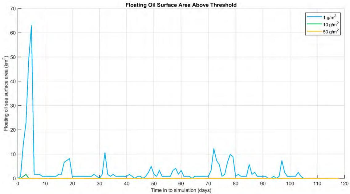
**Figure 13.20** Time series of the sea surface exposure above each threshold for the trajectory with the largest swept area of floating oil above 10 g/m<sup>2</sup>.
