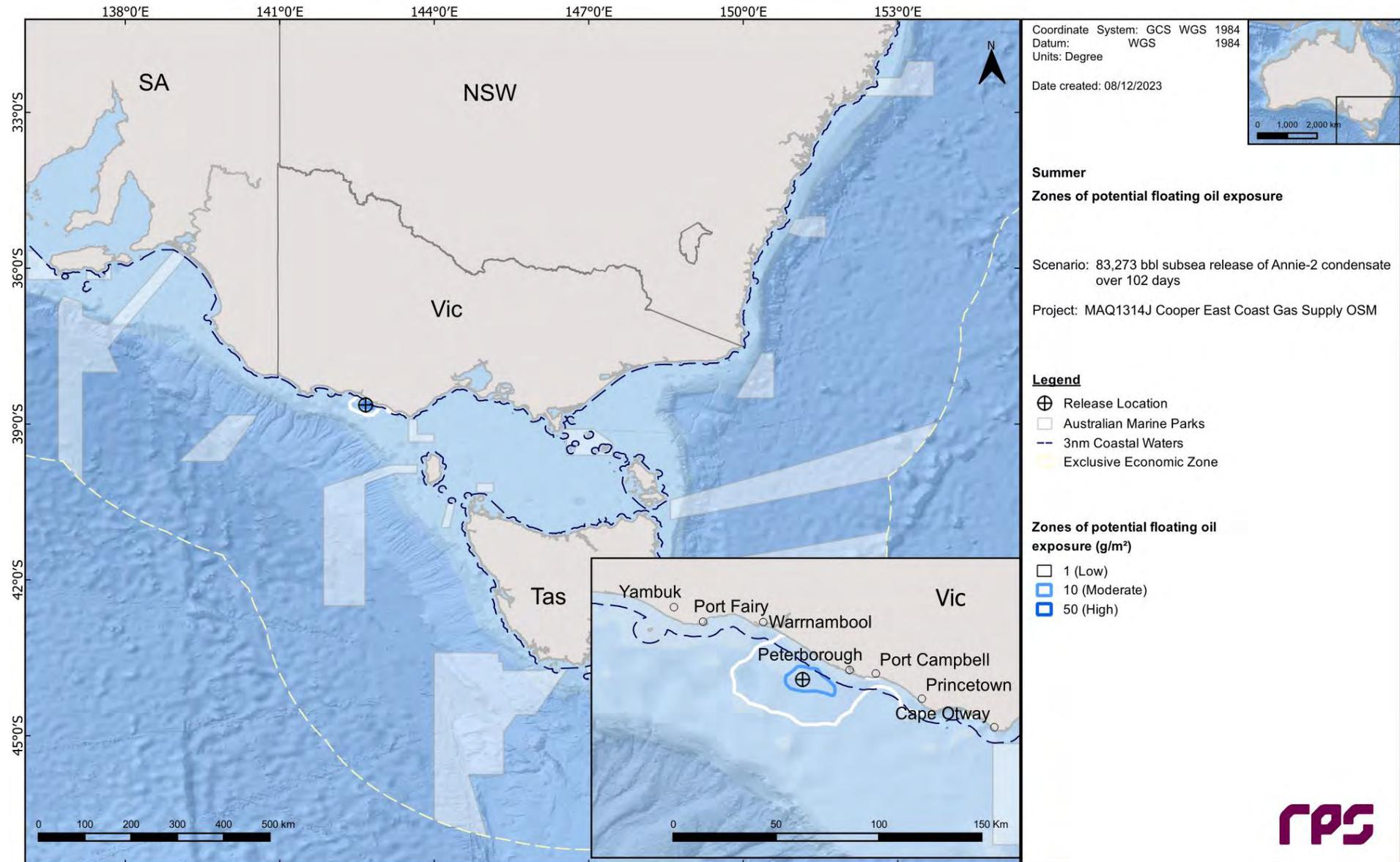
**Figure 12.1** Zones of potential floating oil exposure in the event of an 83,273 bbl subsurface release from a loss of well control at Pecten East-2 over 102 days. The results were calculated from 100 spill simulations during summer conditions.
