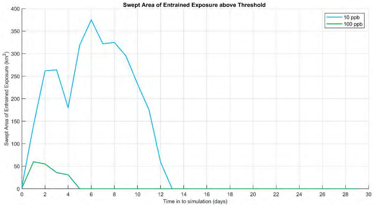
**Figure 10.24** Time series of the entrained hydrocarbon exposure area above each threshold for the trajectory with the largest area of entrained hydrocarbon exposure above 100 ppb. Results are based on a 250 m<sup>3</sup> surface release of MDO over 6 hours, tracked for 30 days.
