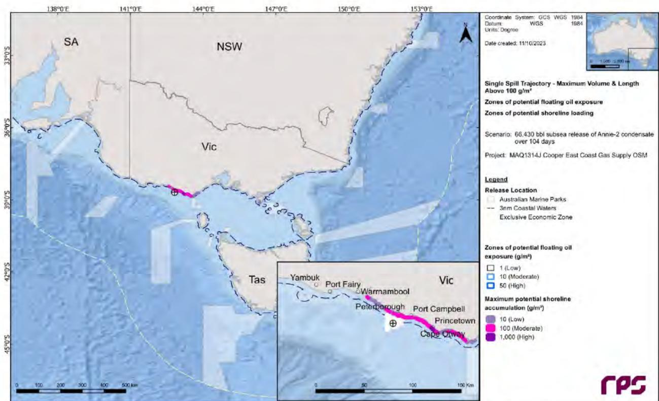
**Figure 13.22 Zones of potential floating oil exposure and shoreline accumulation, for the trajectory with the largest volume ashore and the longest length of shoreline with accumulation above 100 g/m<sup>2</sup>.**
