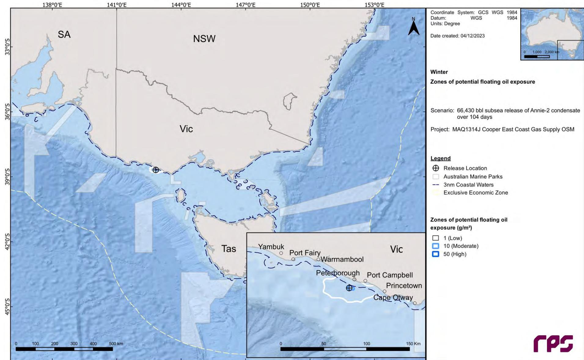
**Figure 13.2** Zones of potential floating oil exposure in the event of a 66,430 bbl subsurface release from a loss of well control at Annie-2 over 104 days. The results were calculated from 100 spill simulations during winter conditions.
