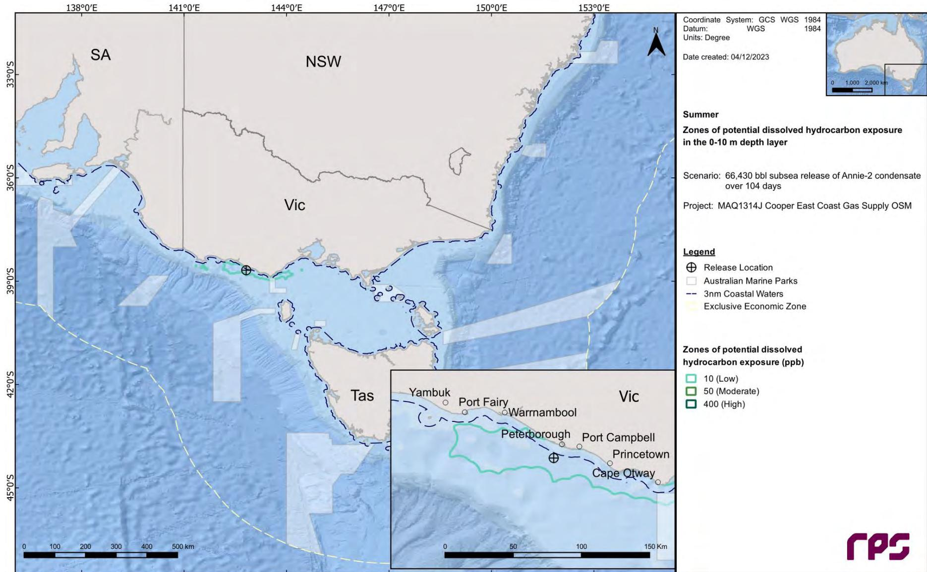
**Figure 13.9** Zones of potential dissolved hydrocarbon exposure at 0-10 m below the sea in the event of a 66,430 bbl subsurface release from a loss of well control at Annie-2 over 104 days. The results were calculated from 100 spill simulations during summer conditions.
