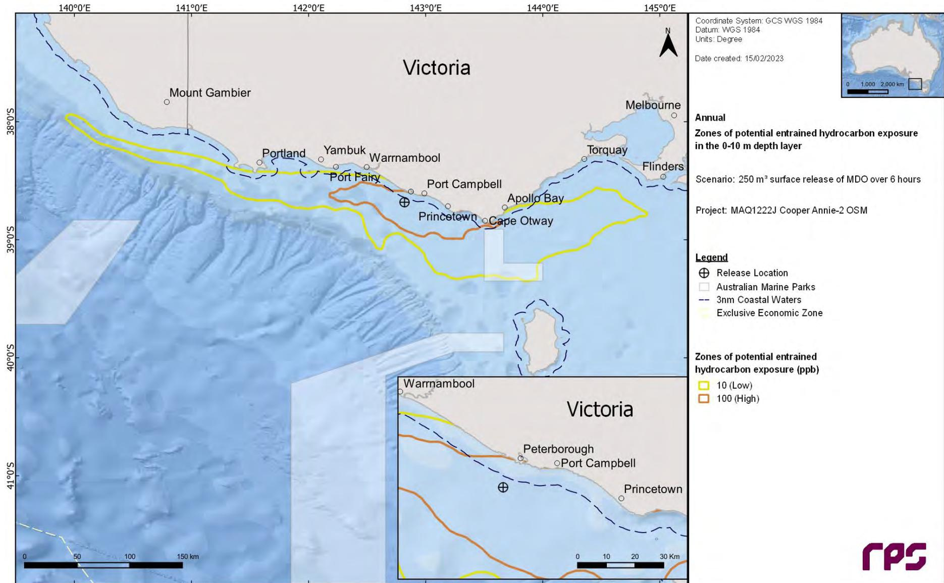
Figure 10.10 Zones of potential entrained hydrocarbon exposure at 0-10 m below the sea surface in the event of a 250 m<sup>3</sup> of MDO containment loss over 6 hours tracked for 30 days. The results were calculated from 100 spill simulations.
