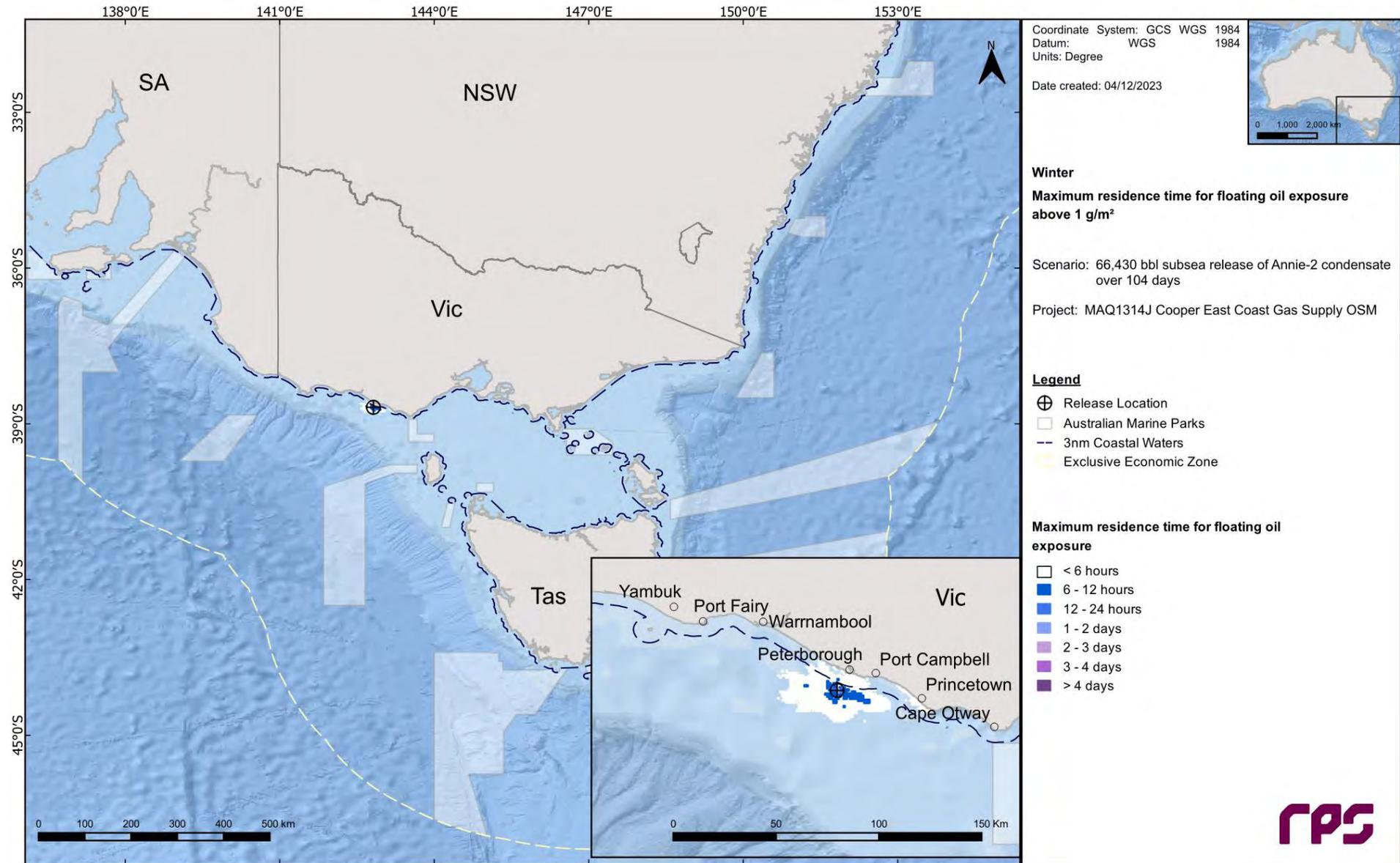
Figure 13.4 Maximum residence time of floating oil exposure above 1 g/m<sup>2</sup>, in the event of a 66,430 bbl subsurface release from a loss of well control at Annie-2 over 104 days. The results were calculated from 100 spill simulations during winter conditions.
