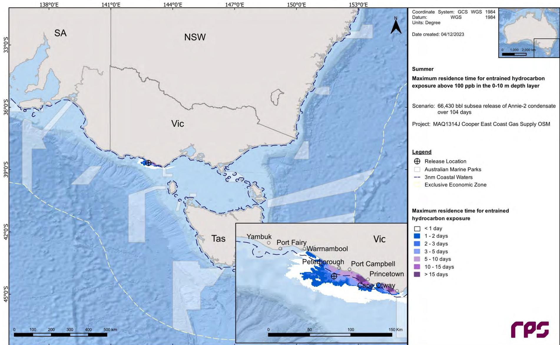
**Figure 13.17 Maximum residence time for entrained hydrocarbon exposure above 100 ppb, at 0-10 m below the sea in the event of a 66,430 bbl (10,562 m<sup>3</sup>) subsurface release from a loss of well control at Annie-2 over 104 days. The results were calculated from 100 spill simulations during summer conditions.**
