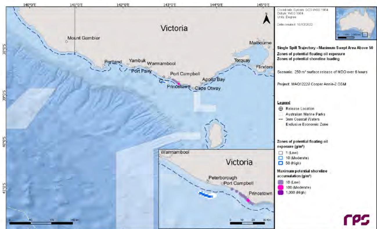
**Figure 10.16 Zones of potential floating oil exposure and shoreline accumulation, for the trajectory with the largest swept area of floating oil above 50 g/m<sup>2</sup>. Results are based on a 250 m<sup>3</sup> surface release of MDO over 6 hours, tracked for 30 days.**
