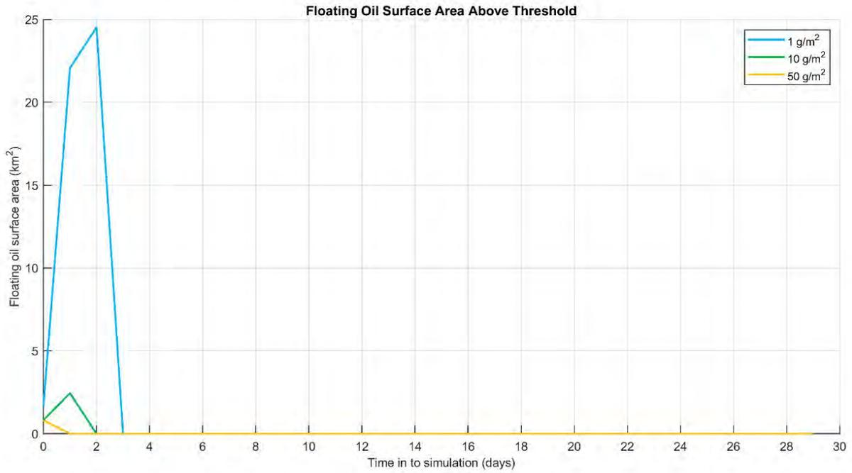
**Figure 10.14** Time series of the sea surface exposure above each threshold for the trajectory with the largest swept area of floating oil above 10 g/m<sup>2</sup>. Results are based on a 250 m<sup>3</sup> surface release of MDO over 6 hours, tracked for 30 days.
