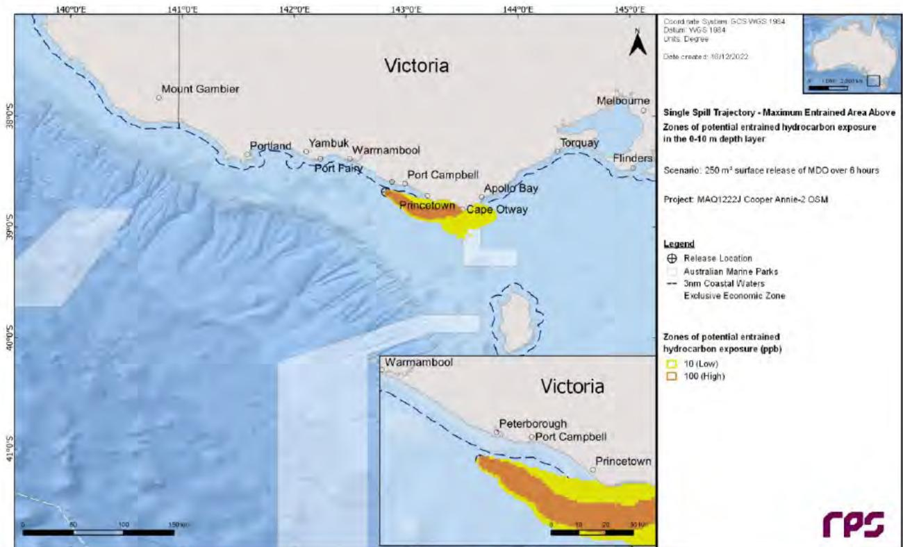
**Figure 10.23** Zones of potential entrained hydrocarbon exposure, for the trajectory with the largest area of entrained hydrocarbon exposure above 100 ppb. Results are based on a 250 m<sup>3</sup> surface release of MDO over 6 hours, tracked for 30 days.
