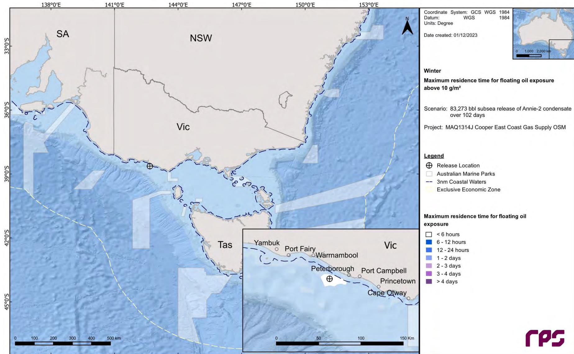
**Figure 12.6 Maximum residence time of floating oil exposure above 10 g/m<sup>2</sup>, in the event of an 83,273 bbl subsurface release from a loss of well control at Pecten East-2 over 102 days. The results were calculated from 100 spill simulations during winter conditions.**
