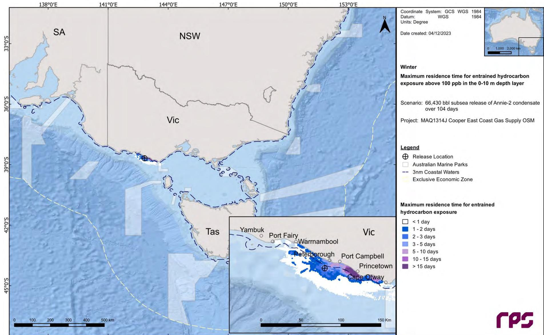
**Figure 13.18 Maximum residence time for entrained hydrocarbon exposure above 100 ppb, at 0-10 m below the sea in the event of a 66,430 bbl (10,562 m<sup>3</sup>) subsurface release from a loss of well control at Annie-2 over 104 days. The results were calculated from 100 spill simulations during winter conditions.**
