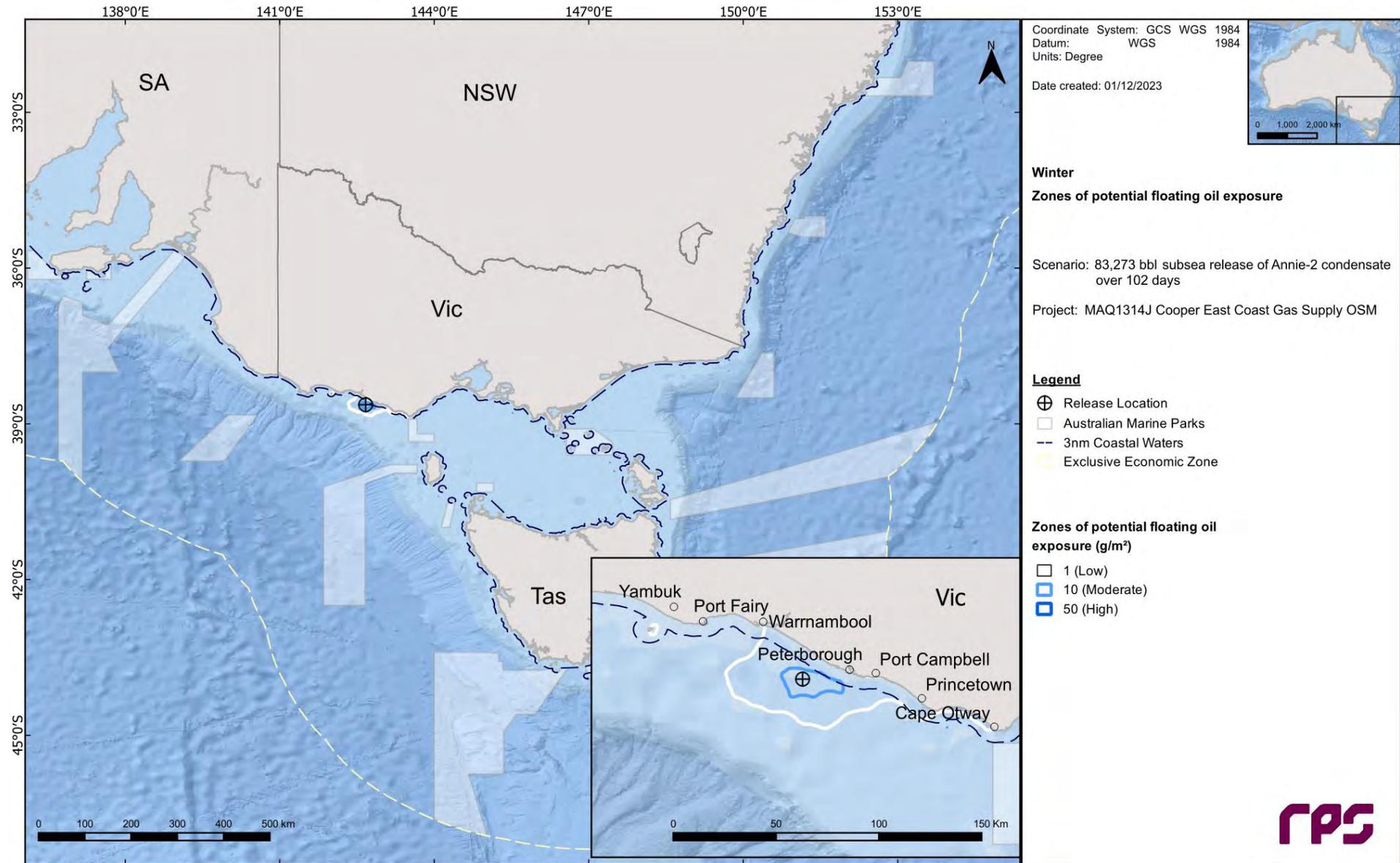
**Figure 12.2** Zones of potential floating oil exposure in the event of an 83,273 bbl subsurface release from a loss of well control at Pecten East-2 over 102 days. The results were calculated from 100 spill simulations during winter conditions.
