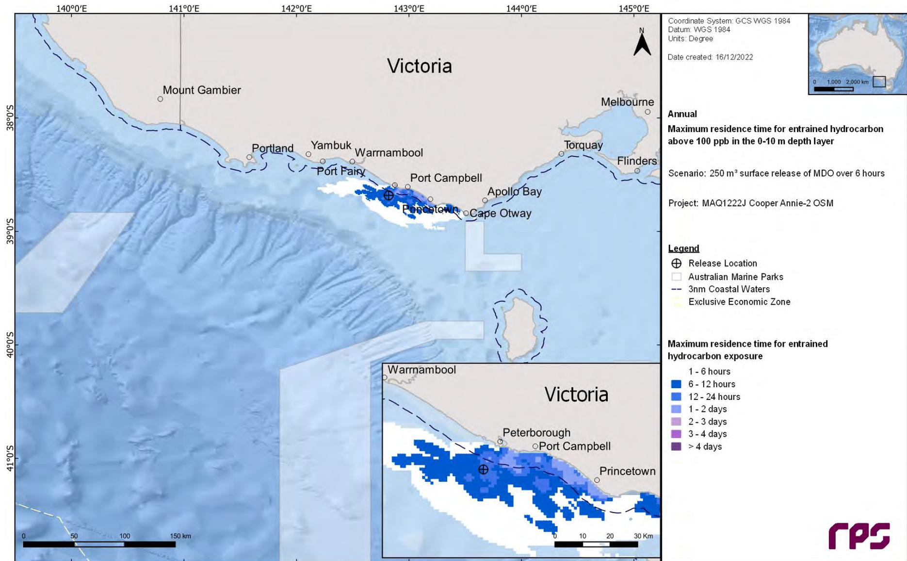
Figure 10.12 Maximum residence time for entrained hydrocarbon exposure above 100 ppb, at 0-10 m below the sea in the event of a 250 m<sup>3</sup> of MDO containment loss over 6 hours tracked for 30 days. The results were calculated from 100 spill simulations.
