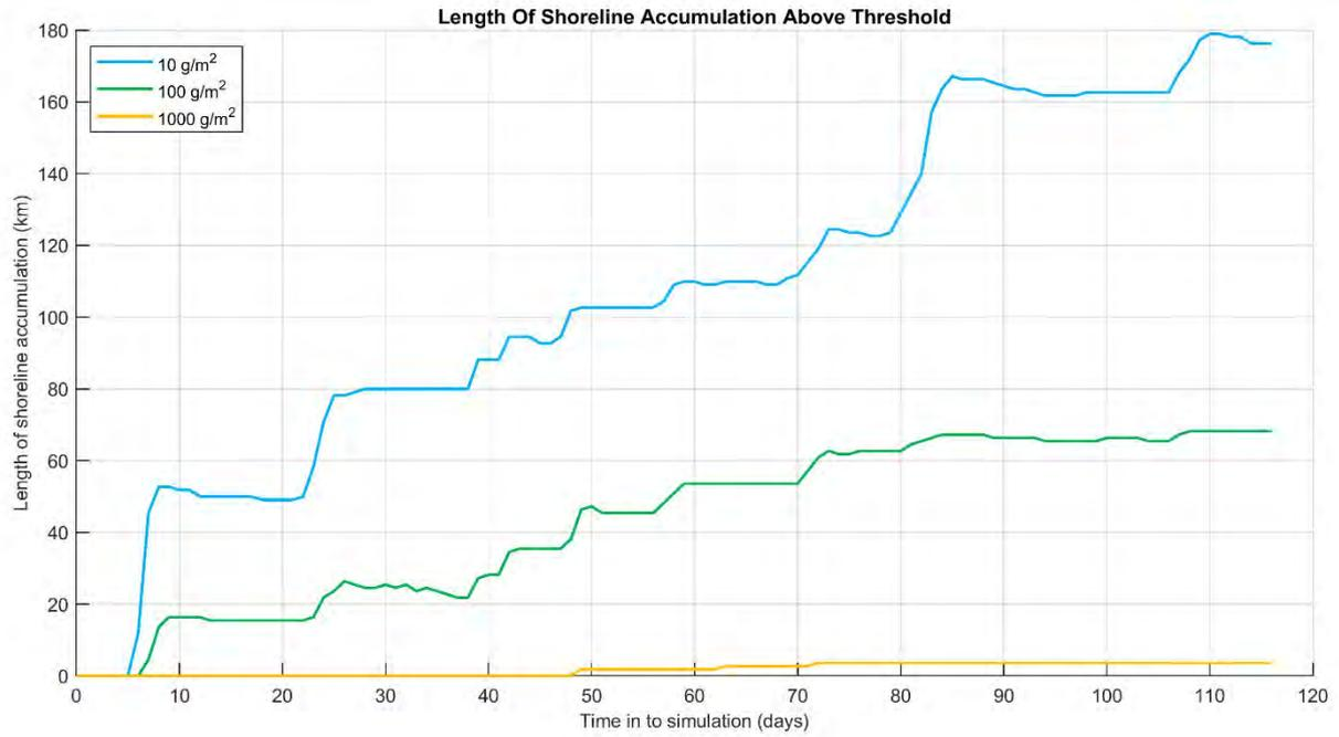
Figure 12.26 Time series of the length of shoreline with accumulation above each threshold for the trajectory with the longest length of shoreline with accumulation above 100 g/m<sup>2</sup>.
