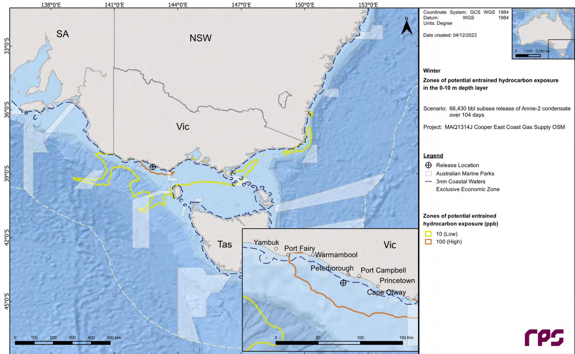
**Figure 13.14** Zones of potential entrained hydrocarbon exposure at 0-10 m below the sea surface in the event of a 66,430 bbl subsurface release from a loss of well control at Annie-2 over 104 days. The results were calculated from 100 spill simulations during winter conditions.
