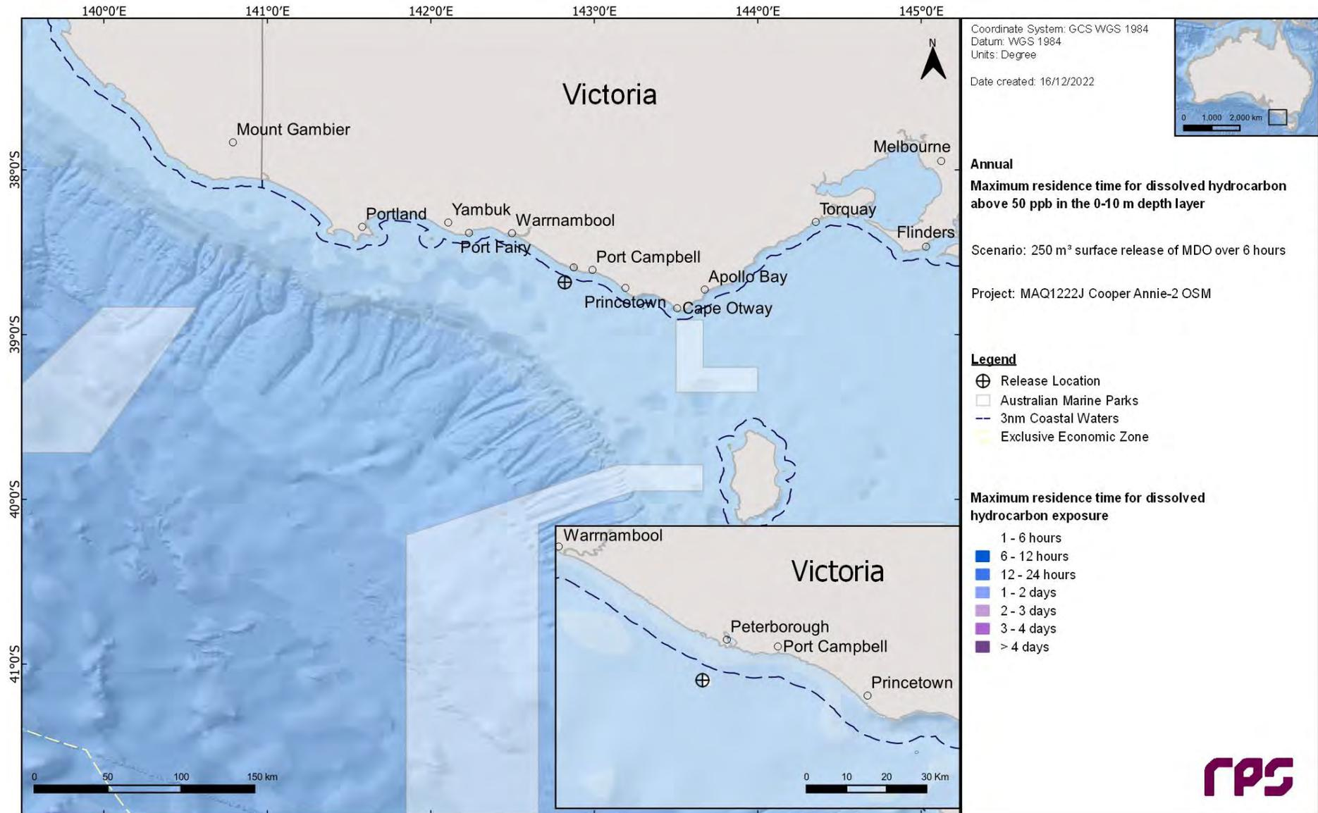
**Figure 10.9** Maximum residence time for dissolved hydrocarbon exposure above 50 ppb, at 0-10 m below the sea surface in the event of a 250 m<sup>3</sup> of MDO containment loss over 6 hours tracked for 30 days. The results were calculated from 100 spill simulations.
