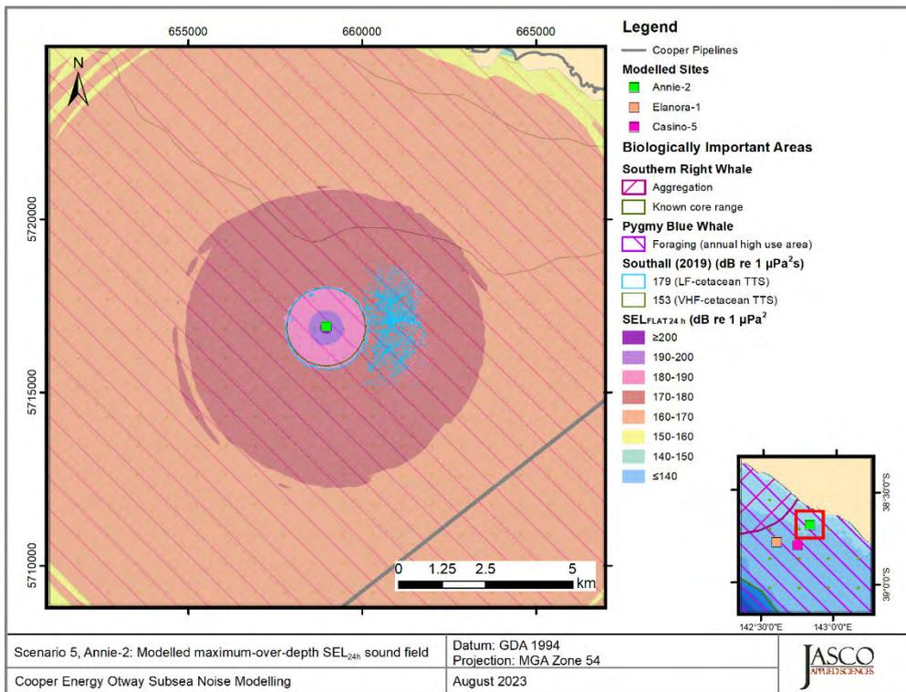
Figure 32. Scenario 5, Drilling and standby OSV during resupply, Annie-2, accumulated  $SEL_{24h}$ : Sound level contour map showing weighted maximum-over-depth  $SEL_{24h}$  results, along with isopleths for TTS in low and very-high-frequency cetaceans. Thresholds omitted here were not reached or not long enough to display graphically.
