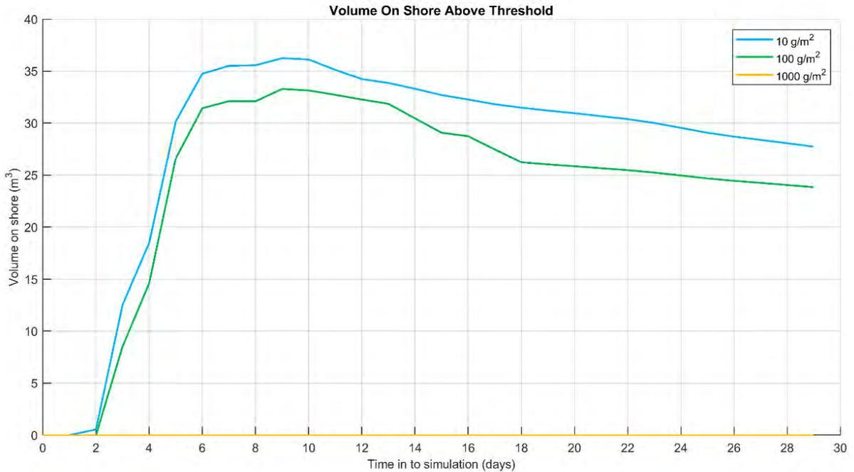
**Figure 10.21** Time series of oil accumulation on the shoreline above each threshold for the trajectory with the largest volume ashore and longest length of shoreline with accumulation above 100 g/m<sup>2</sup>. Results are based on a 250 m<sup>3</sup> surface release of MDO over 6 hours, tracked for 30 days.
