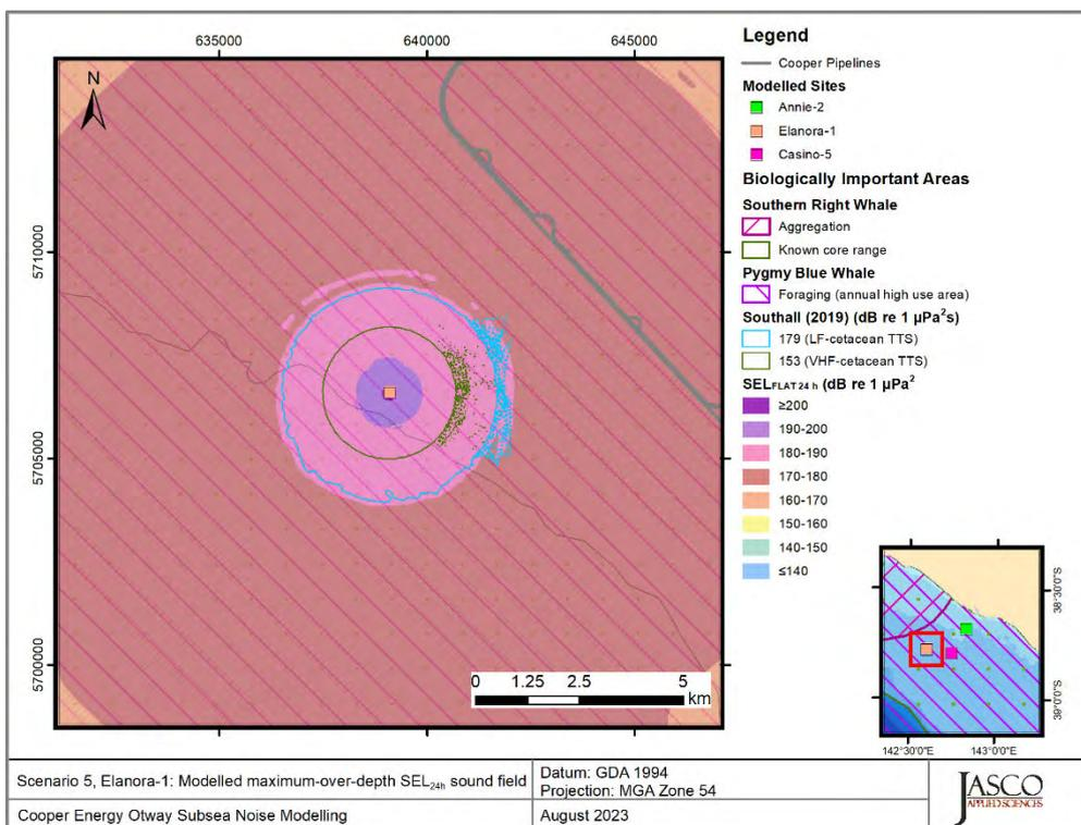
Figure 33. Scenario 5, Drilling and standby OSV during resupply, Elanora-1, accumulated  $SEL_{24h}$ : Sound level contour map showing weighted maximum-over-depth  $SEL_{24h}$  results, along with isopleths for TTS in low and very-high-frequency cetaceans. Thresholds omitted here were not reached or not long enough to display graphically.
