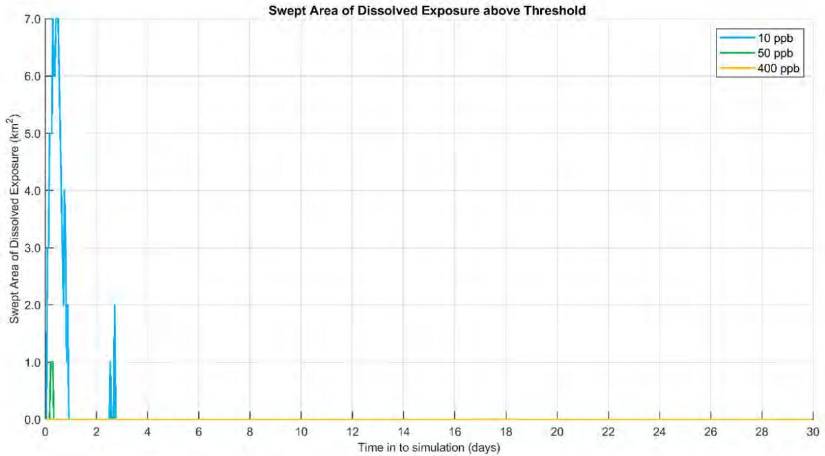
**Figure 10.27** Time series of the dissolved hydrocarbon exposure area above each threshold for the trajectory with the largest area of dissolved hydrocarbon exposure above 50 ppb. Results are based on a 250 m<sup>3</sup> surface release of MDO over 6 hours, tracked for 30 days.
