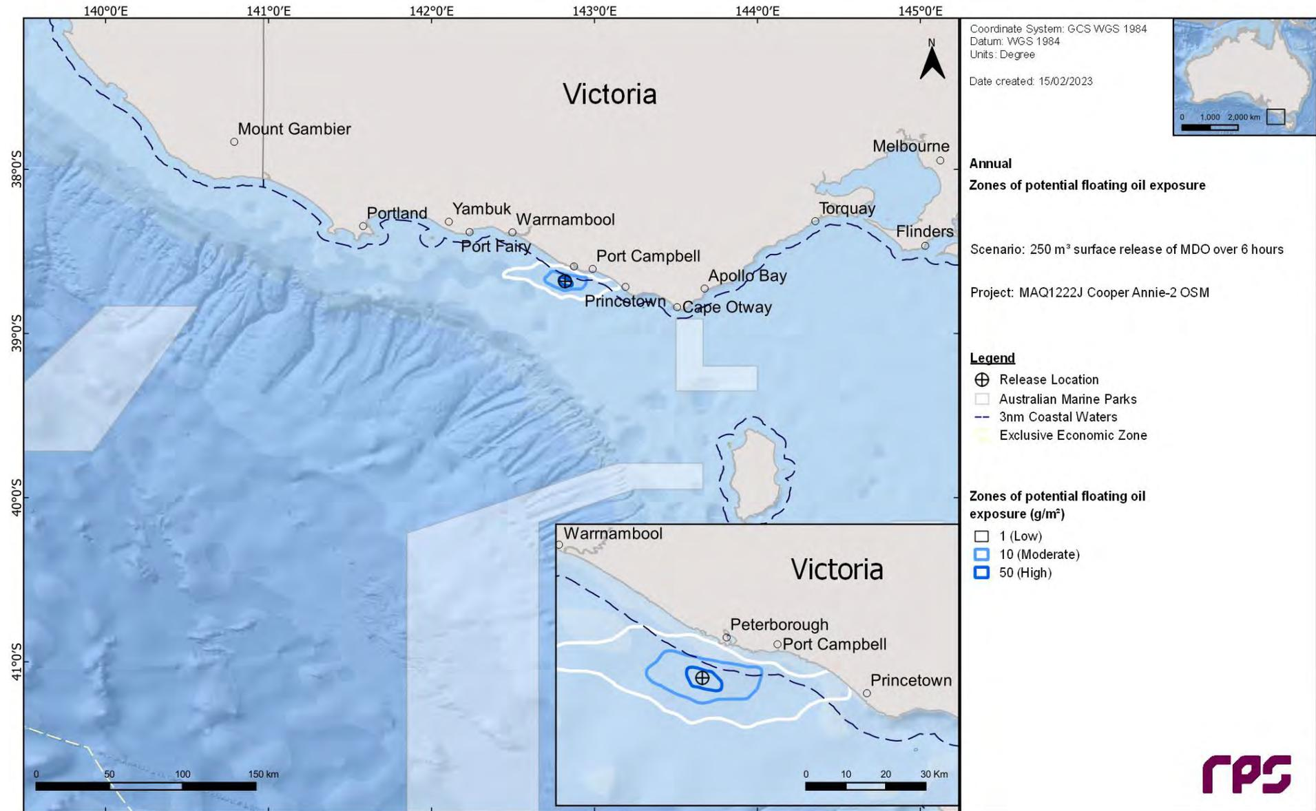
**Figure 10.2** Zones of potential floating oil exposure in the event of a 250 m<sup>3</sup> of MDO containment loss over 6 hours tracked for 30 days. The results were calculated from 100 spill simulations.
