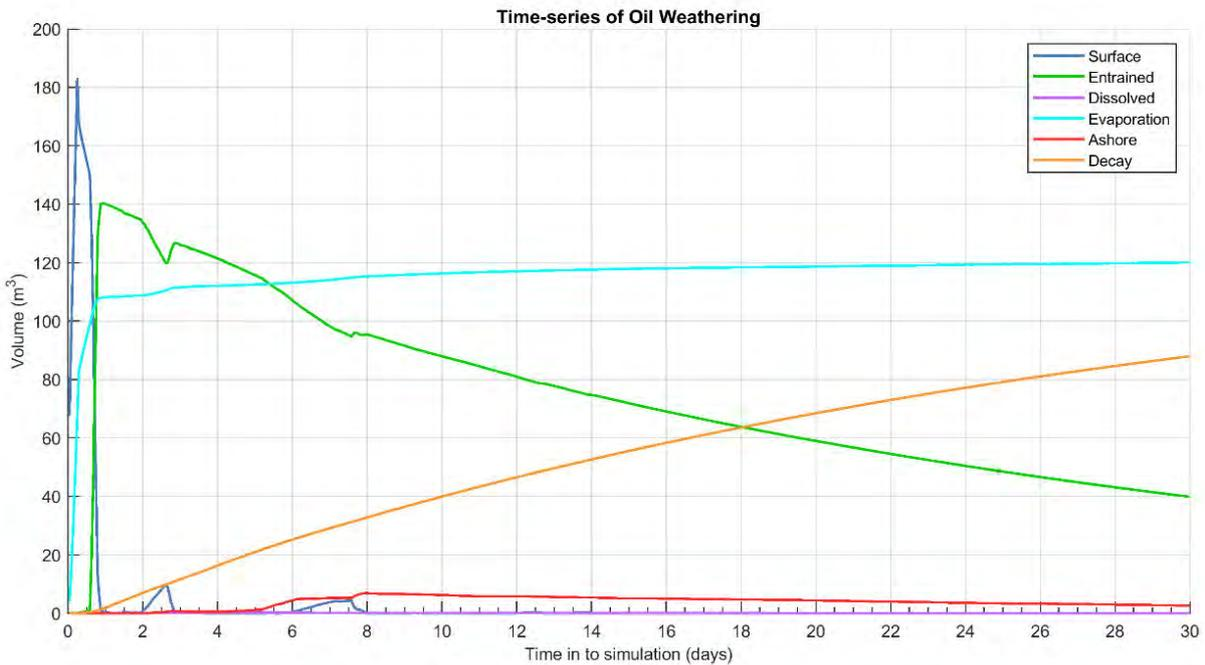
**Figure 10.18** Predicted weathering and fates graph for the trajectory with the largest swept area of floating oil above 50 g/m<sup>2</sup>. Results are based on a 250 m<sup>3</sup> surface release of MDO over 6 hours, tracked for 30 days.
