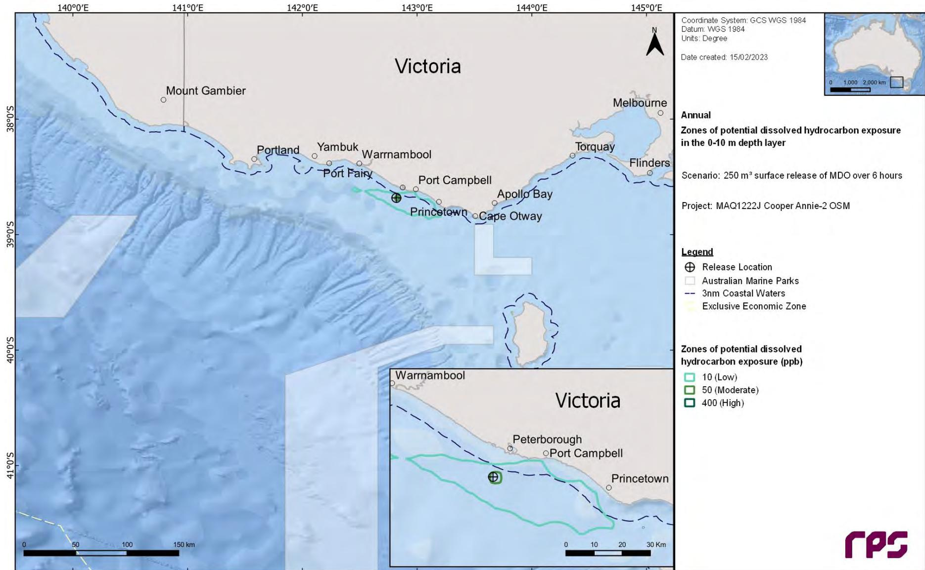
**Figure 10.7** Zones of potential dissolved hydrocarbon exposure at 0-10 m below the sea in the event of a 250 m<sup>3</sup> of MDO containment loss over 6 hours tracked for 30 days. The results were calculated from 100 spill simulations.
