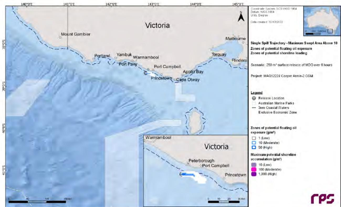
**Figure 10.13 Zones of potential floating oil exposure and shoreline accumulation, for the trajectory with the largest swept area of floating oil above 10 g/m<sup>2</sup>. Results are based on a 250 m<sup>3</sup> surface release of MDO over 6 hours, tracked for 30 days.**
