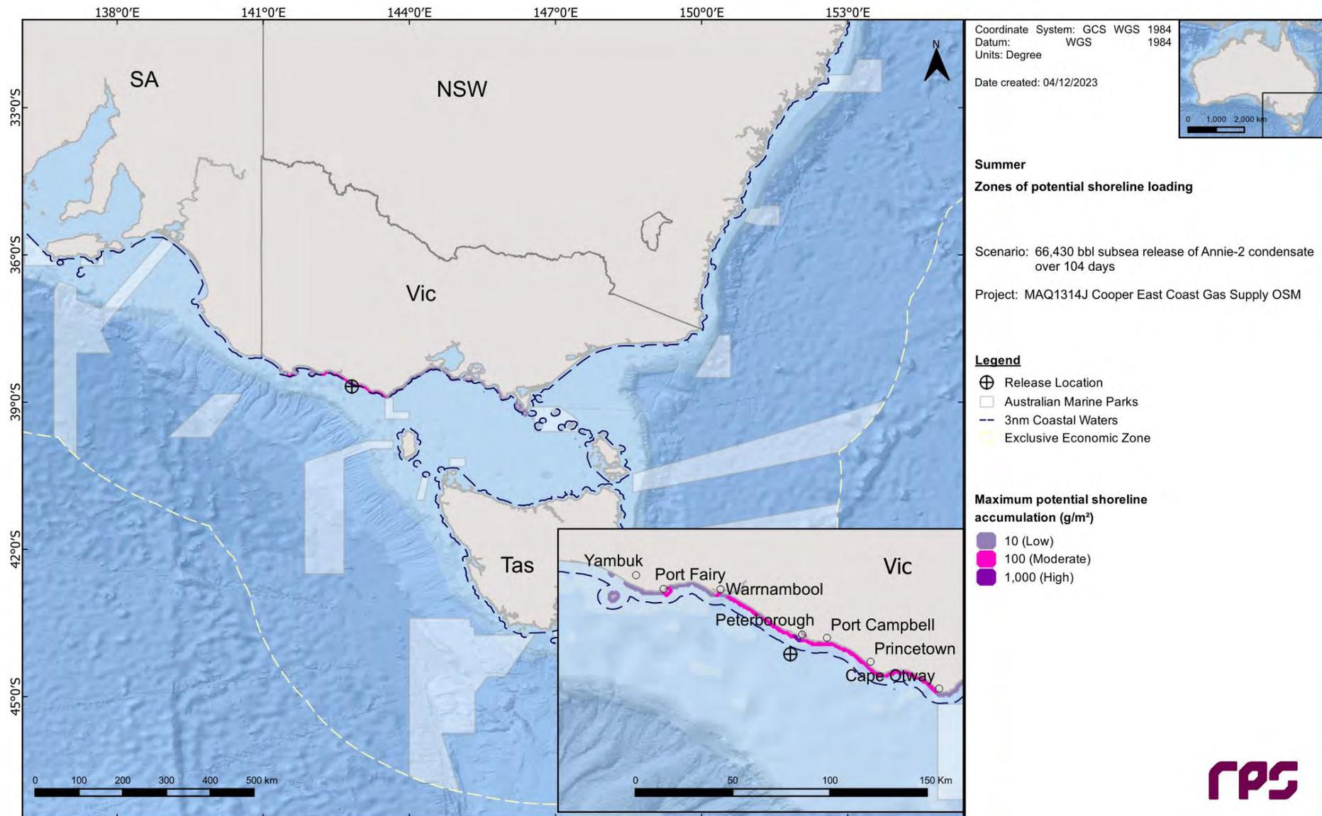
**Figure 13.7** Maximum potential shoreline accumulation in the event of a 66,430 bbl subsurface release from a loss of well control at Annie-2 over 104 days. The results were calculated from 100 spill simulations during summer conditions.
