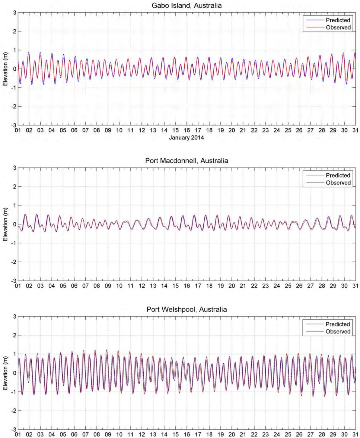
**Figure 3.5 Comparison between HYDROMAP predicted (blue line) and observed (red line) surface elevation at tidal stations Gabo Island (upper image), Port MacDonnell (middle image) and Port Welshpool (lower image).**
