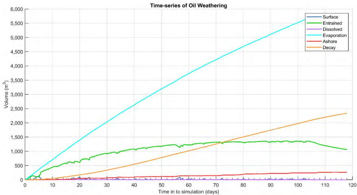
**Figure 13.24** Predicted weathering and fates graph for the trajectory with the largest volume ashore and the longest length of shoreline with accumulation above 100 g/m<sup>2</sup>.
