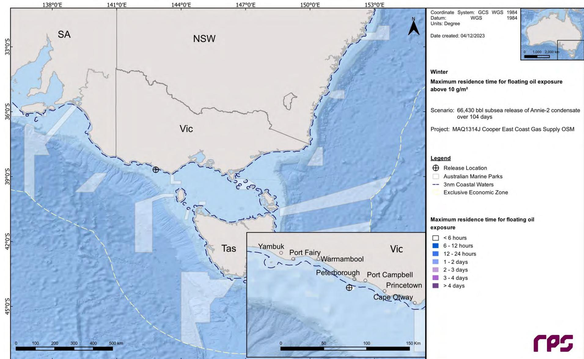
Figure 13.6 Maximum residence time of floating oil exposure above 10 g/m<sup>2</sup>, in the event of a 66,430 bbl subsurface release from a loss of well control at Annie-2 over 104 days. The results were calculated from 100 spill simulations during winter conditions.
