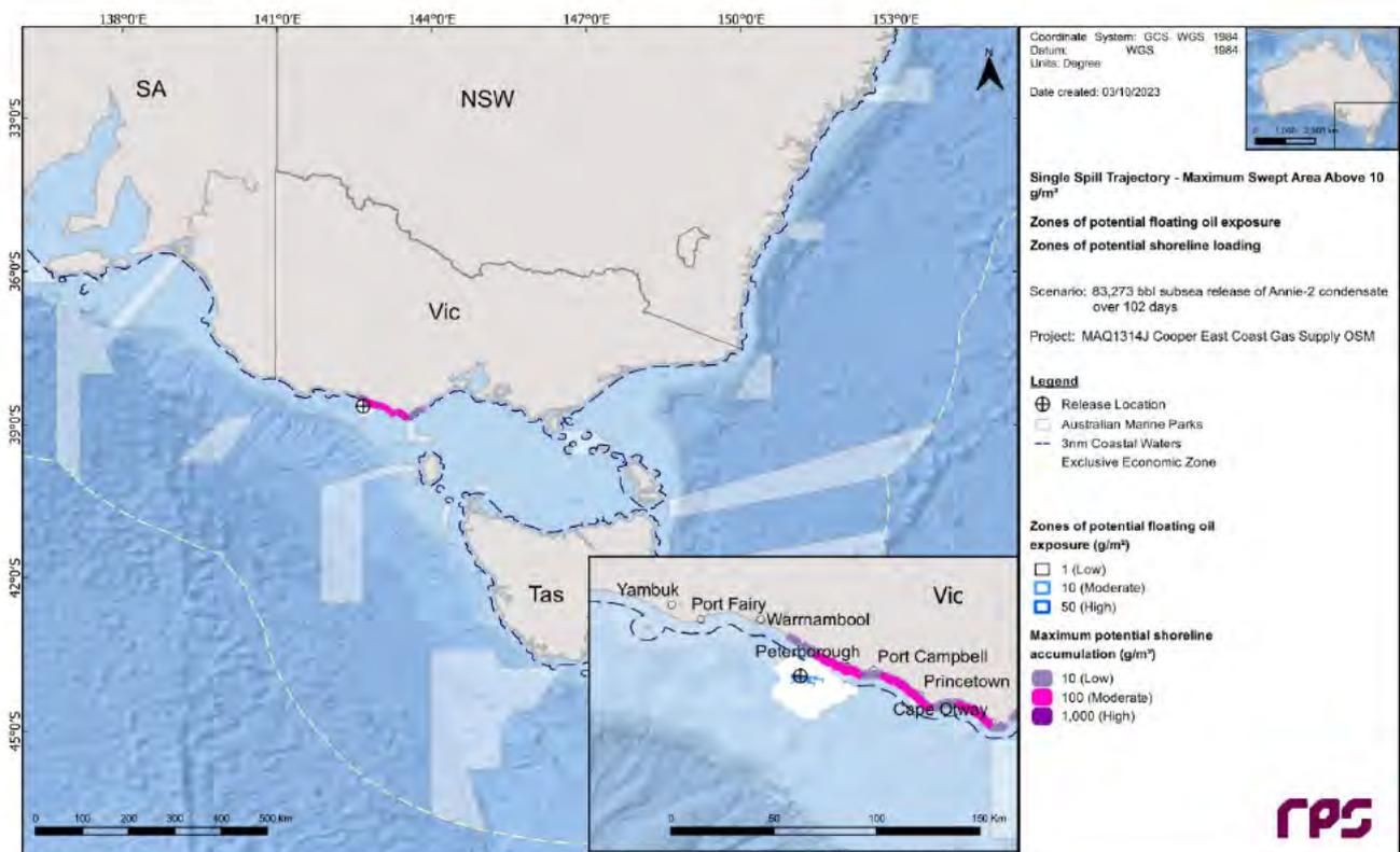
**Figure 12.19 Zones of potential floating oil exposure and shoreline accumulation, for the trajectory with the largest swept area of floating oil above 10 g/m<sup>2</sup>.**
