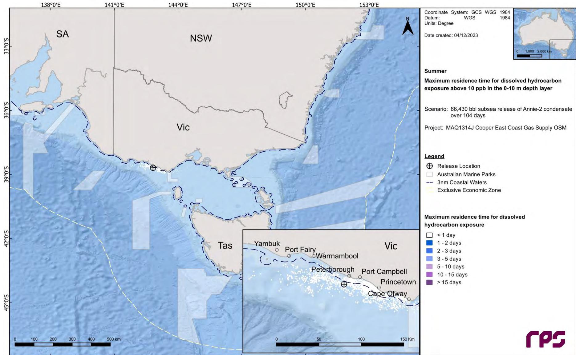
**Figure 13.11 Maximum residence time for dissolved hydrocarbon exposure above 10 ppb, at 0-10 m below the sea surface in the event of a 66,430 bbl (10,562 m<sup>3</sup>) subsurface release from a loss of well control at Annie-2 over 104 days. The results were calculated from 100 spill simulations during summer conditions.**
