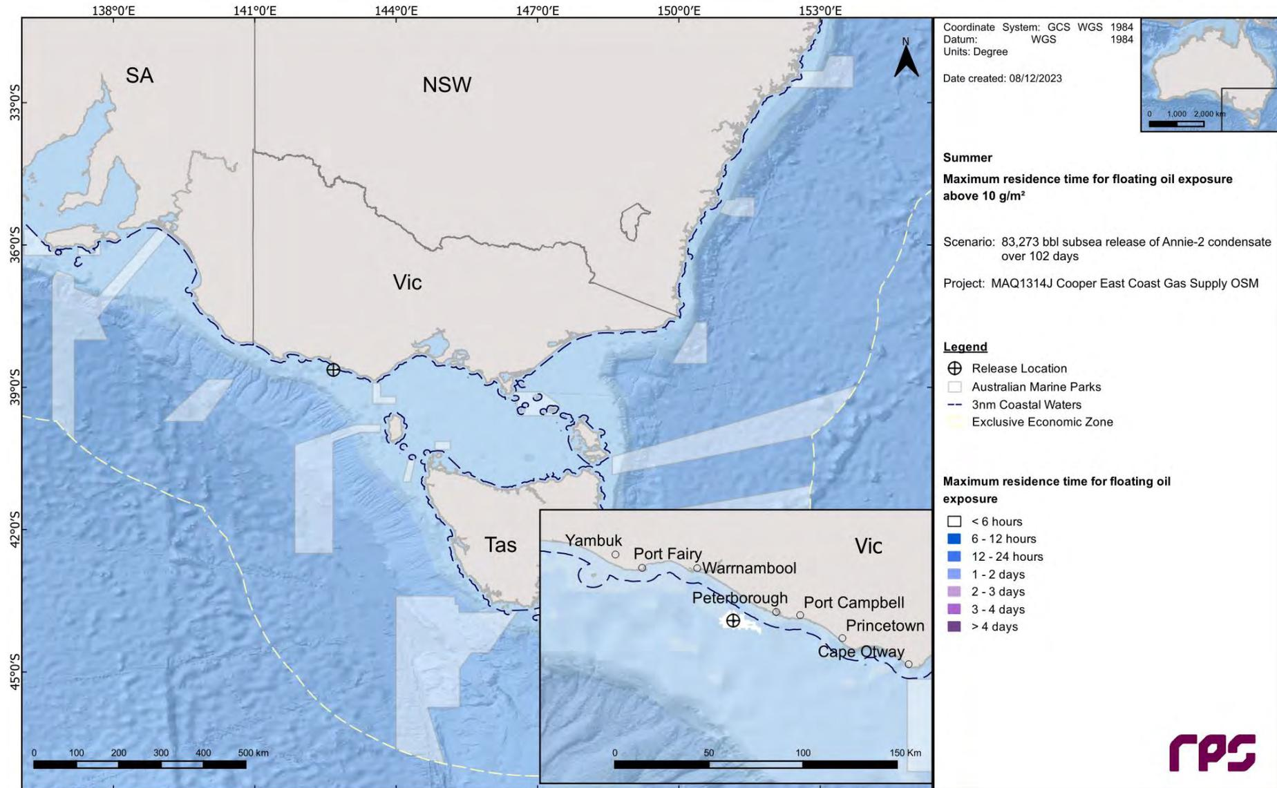
**Figure 12.5 Maximum residence time of floating oil exposure above 10 g/m<sup>2</sup>, in the event of an 83,273 bbl subsurface release from a loss of well control at Pecten East-2 over 102 days. The results were calculated from 100 spill simulations during summer conditions.**
