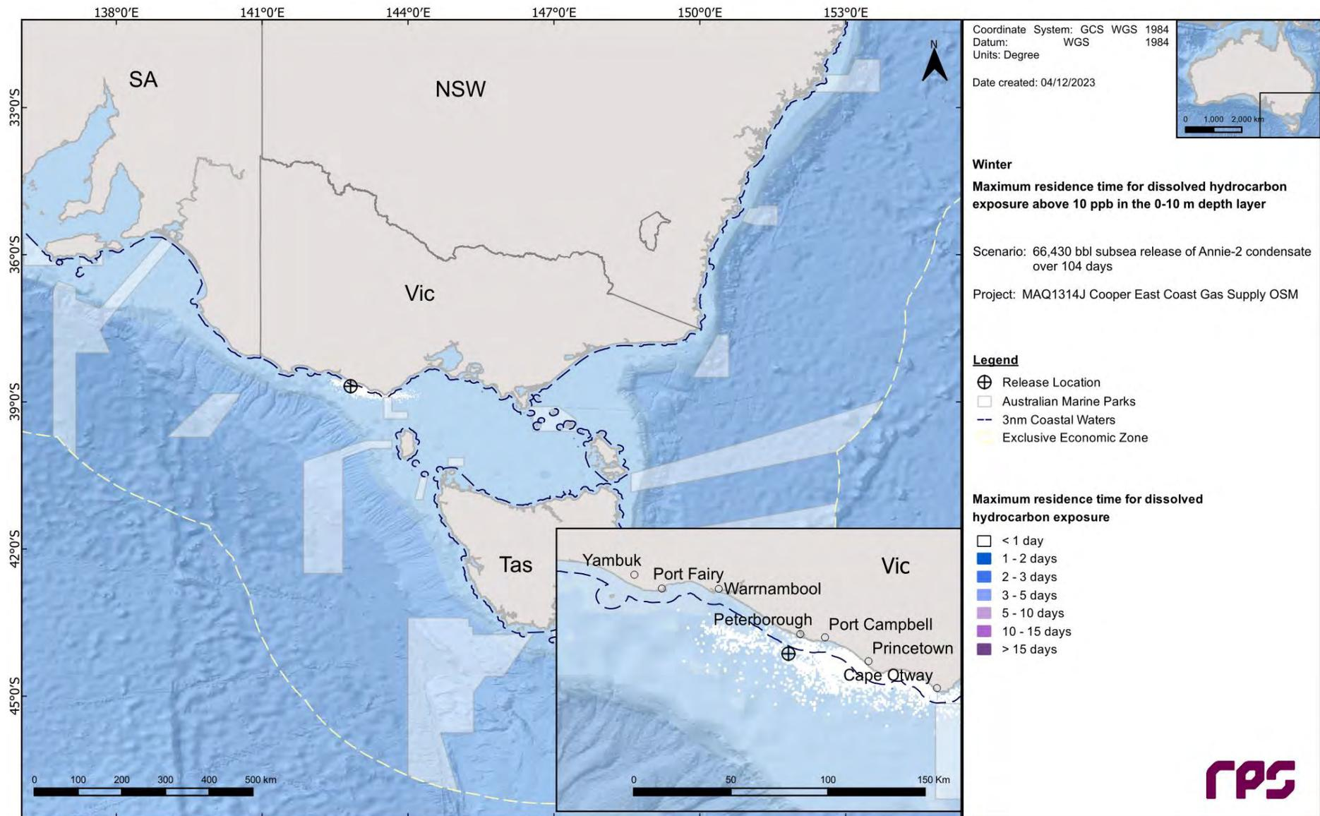
**Figure 13.12 Maximum residence time for dissolved hydrocarbon exposure above 10 ppb, at 0-10 m below the sea surface in the event of a 66,430 bbl (10,562 m<sup>3</sup>) subsurface release from a loss of well control at Annie-2 over 104 days. The results were calculated from 100 spill simulations during winter conditions.**
