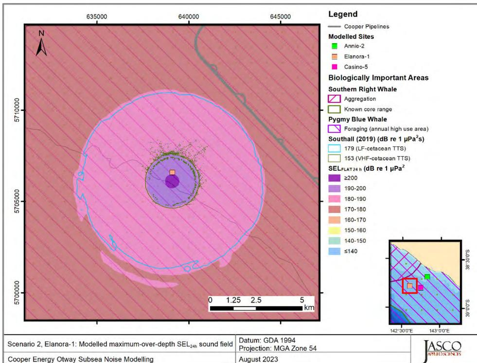
Figure 27. Scenario 2, Mooring, Elanora-1, accumulated  $SEL_{24h}$ : Sound level contour map showing weighted maximum-over-depth  $SEL_{24h}$  results, along with isopleths for TTS in low and very-high-frequency cetaceans. Thresholds omitted here were not reached or not long enough to display graphically.
