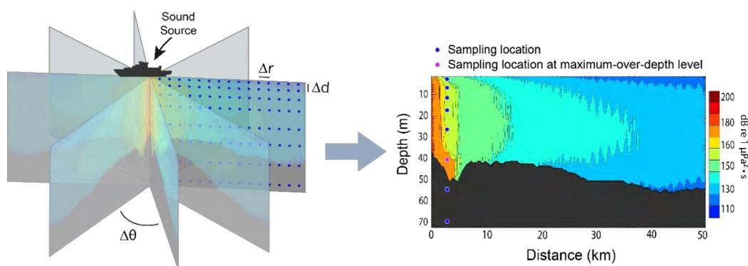
Figure B-4. The  $N \times 2$ -D and maximum-over-depth modelling approach used by MONM.
