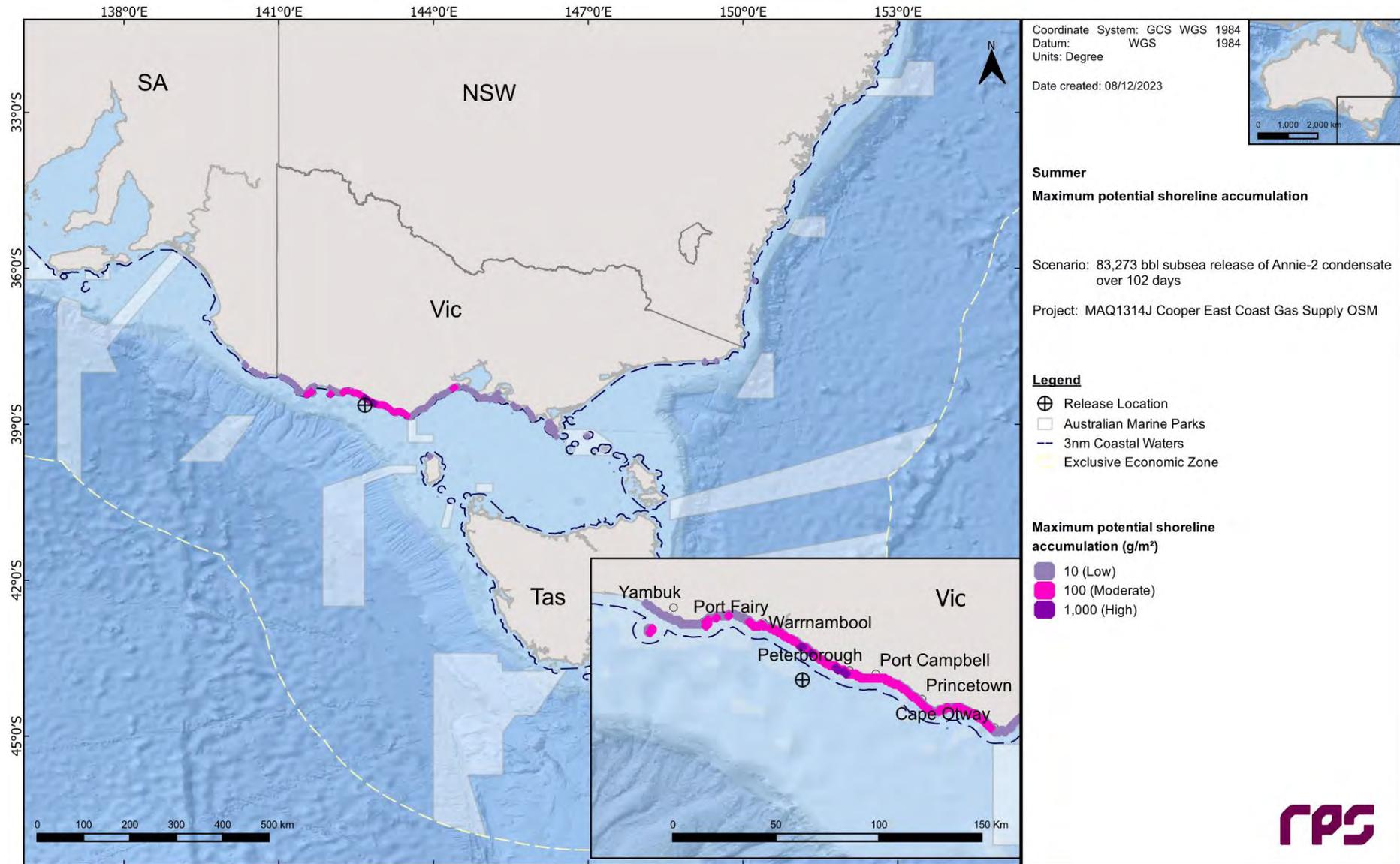
**Figure 12.7** Maximum potential shoreline accumulation in the event of an 83,273 bbl subsurface release from a loss of well control at Pecten East-2 over 102 days. The results were calculated from 100 spill simulations during summer conditions.
