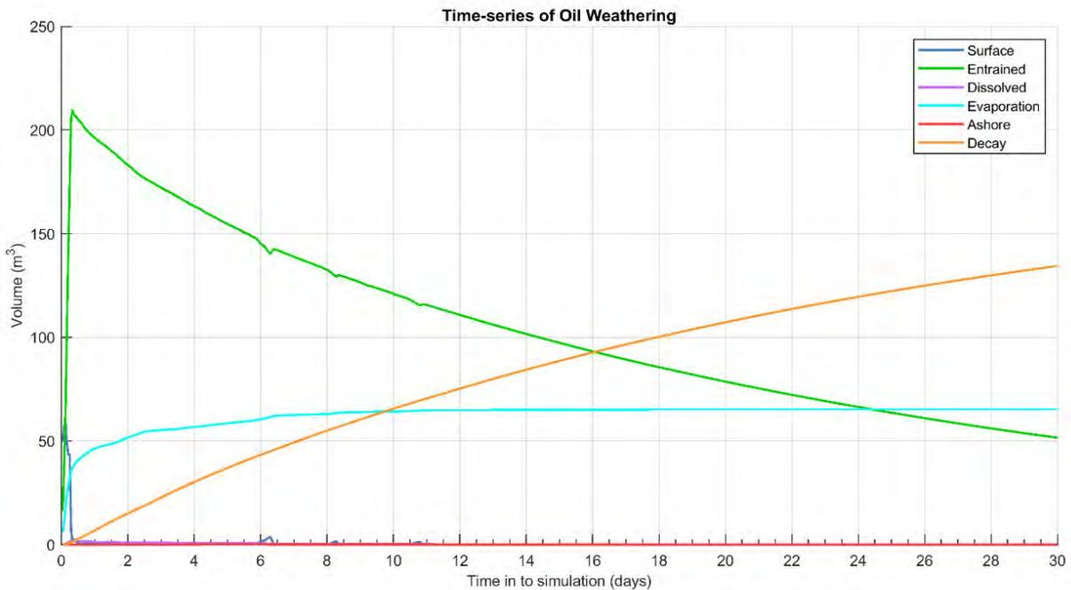
**Figure 10.25** Predicted weathering and fates graph for the trajectory with the largest area of entrained hydrocarbon exposure above 100 ppb. Results are based on a 250 m<sup>3</sup> surface release of MDO over 6 hours, tracked for 30 days.
