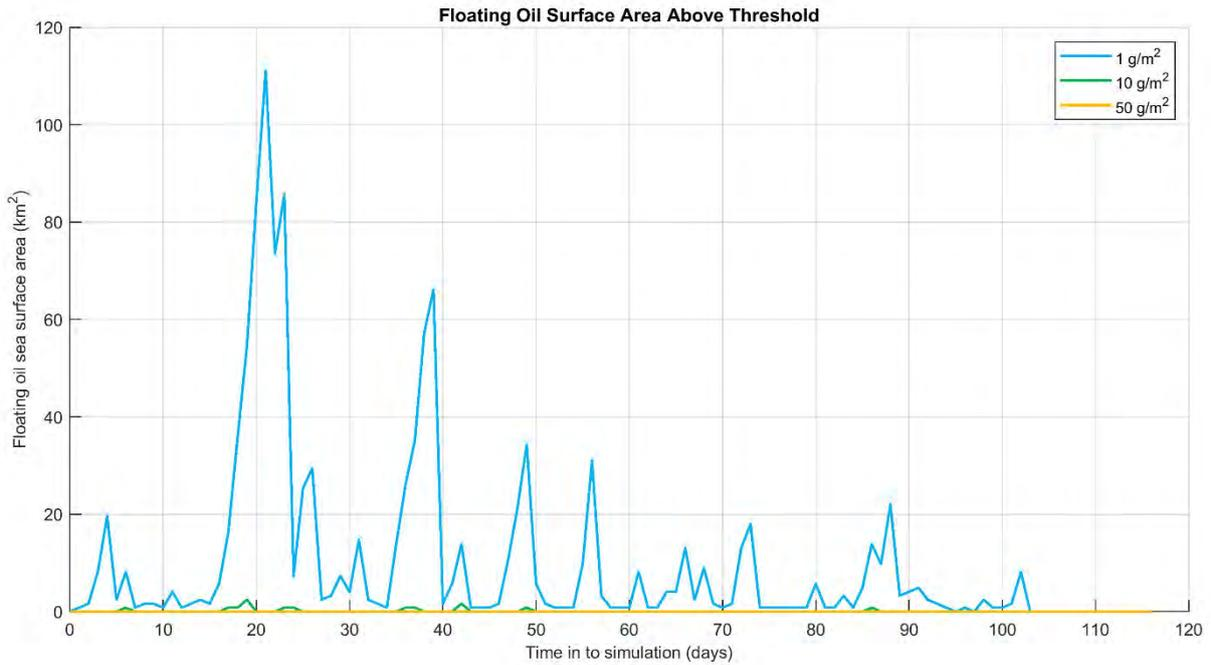
**Figure 12.20** Time series of the sea surface exposure above each threshold for the trajectory with the largest swept area of floating oil above 10 g/m<sup>2</sup>.
