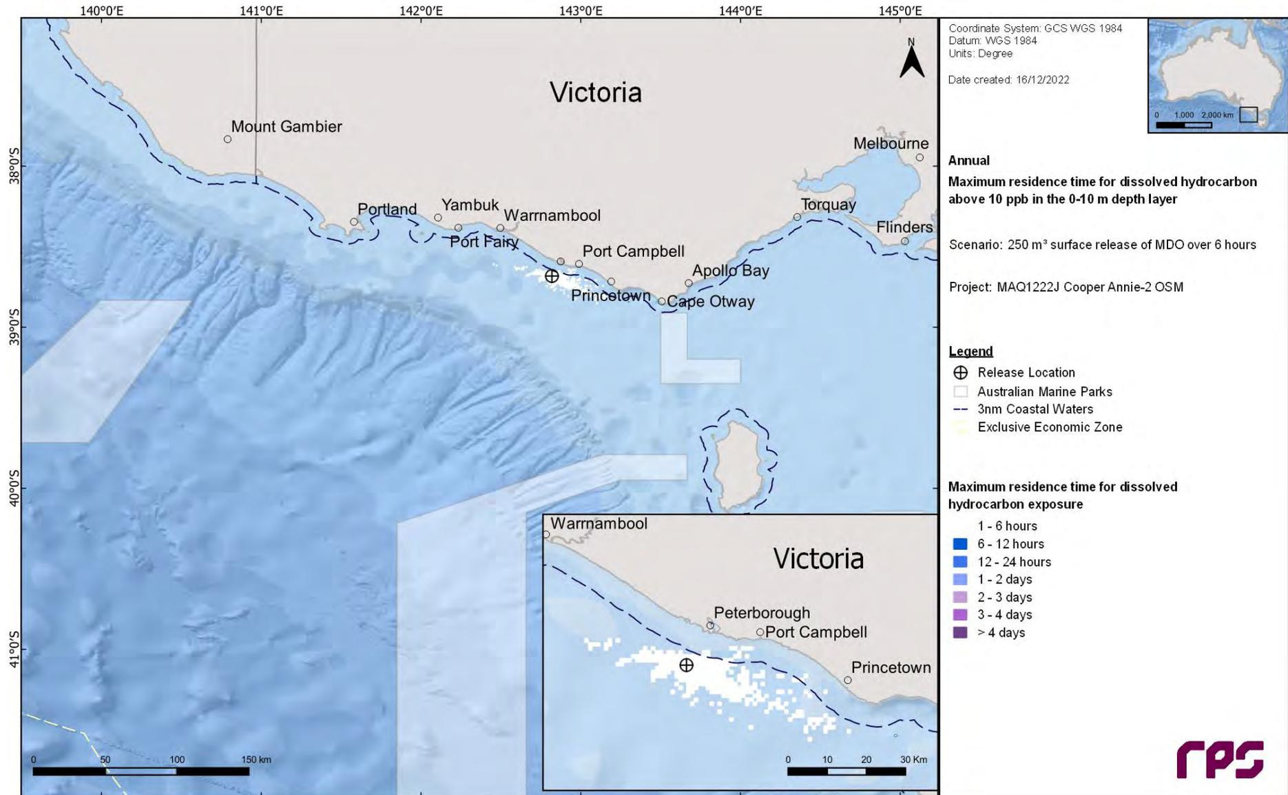
**Figure 10.8** Maximum residence time for dissolved hydrocarbon exposure above 10 ppb, at 0-10 m below the sea surface in the event of a 250 m<sup>3</sup> of MDO containment loss over 6 hours tracked for 30 days. The results were calculated from 100 spill simulations.
