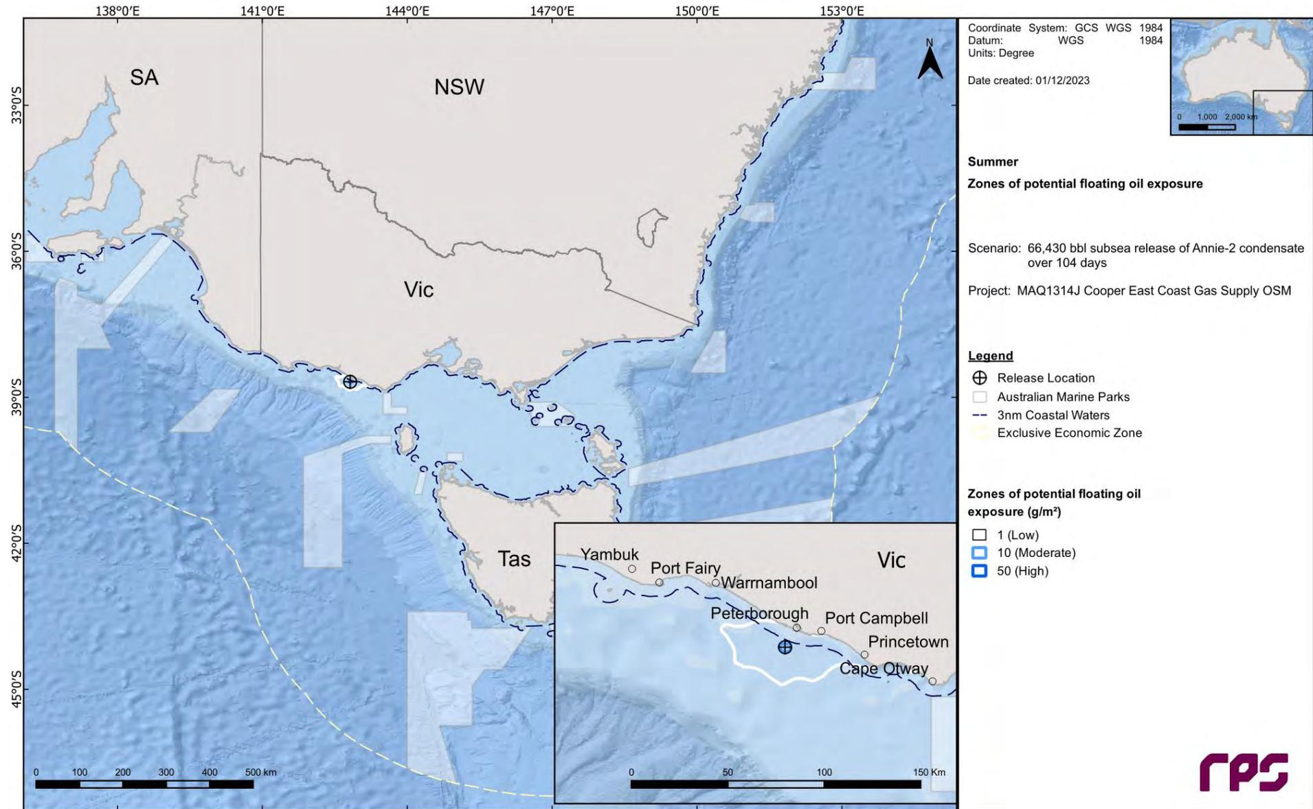
**Figure 13.1** Zones of potential floating oil exposure in the event of a 66,430 bbl subsurface release from a loss of well control at Annie-2 over 104 days. The results were calculated from 100 spill simulations during summer conditions.
