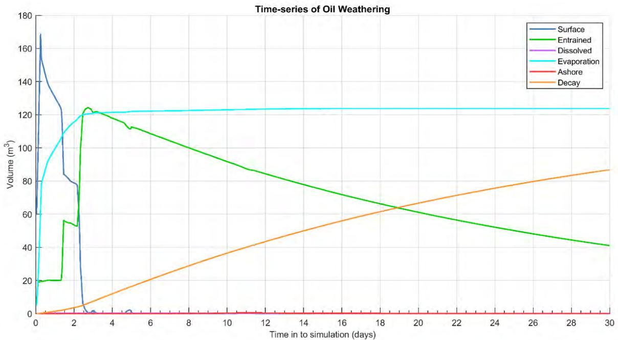
**Figure 10.15** Predicted weathering and fates graph for the trajectory with the largest swept area of floating oil above 10 g/m<sup>2</sup>. Results are based on a 250 m<sup>3</sup> surface release of MDO over 6 hours, tracked for 30 days.
