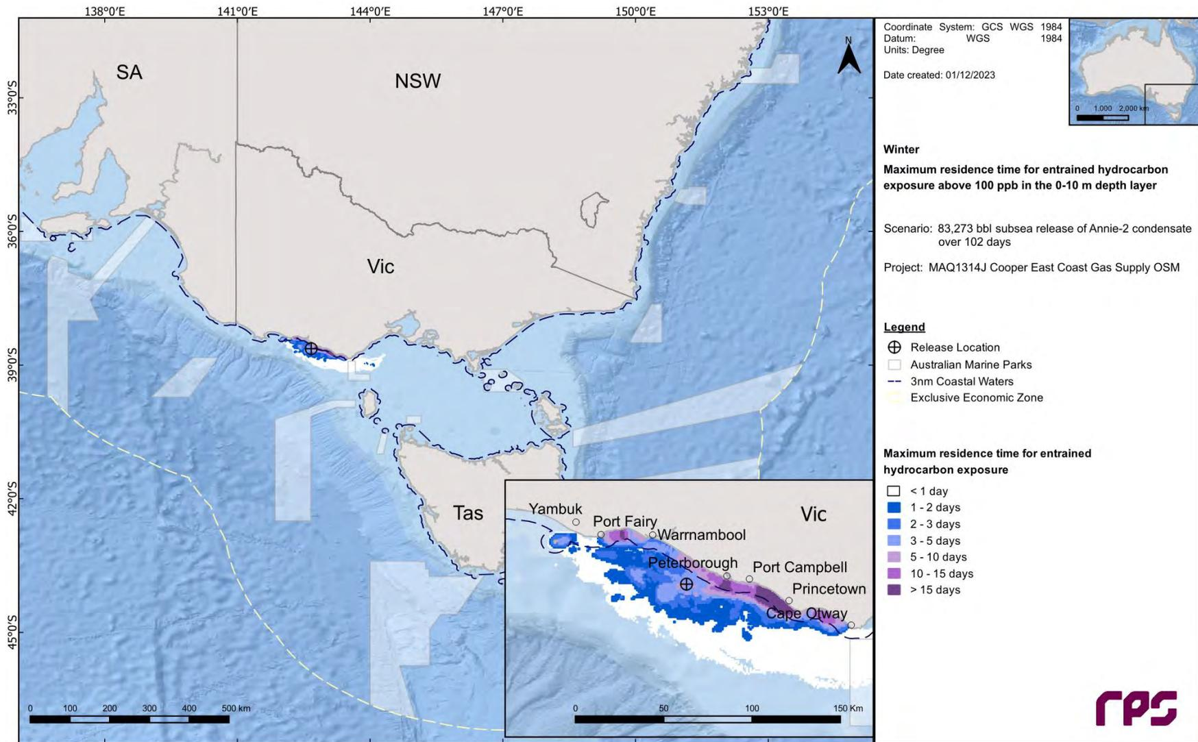
**Figure 12.18 Maximum residence time for entrained hydrocarbon exposure above 100 ppb, at 0-10 m below the sea in the event of an 83,273 bbl subsurface release from a loss of well control at Pecten East-2 over 102 days. The results were calculated from 100 spill simulations during winter conditions.**
