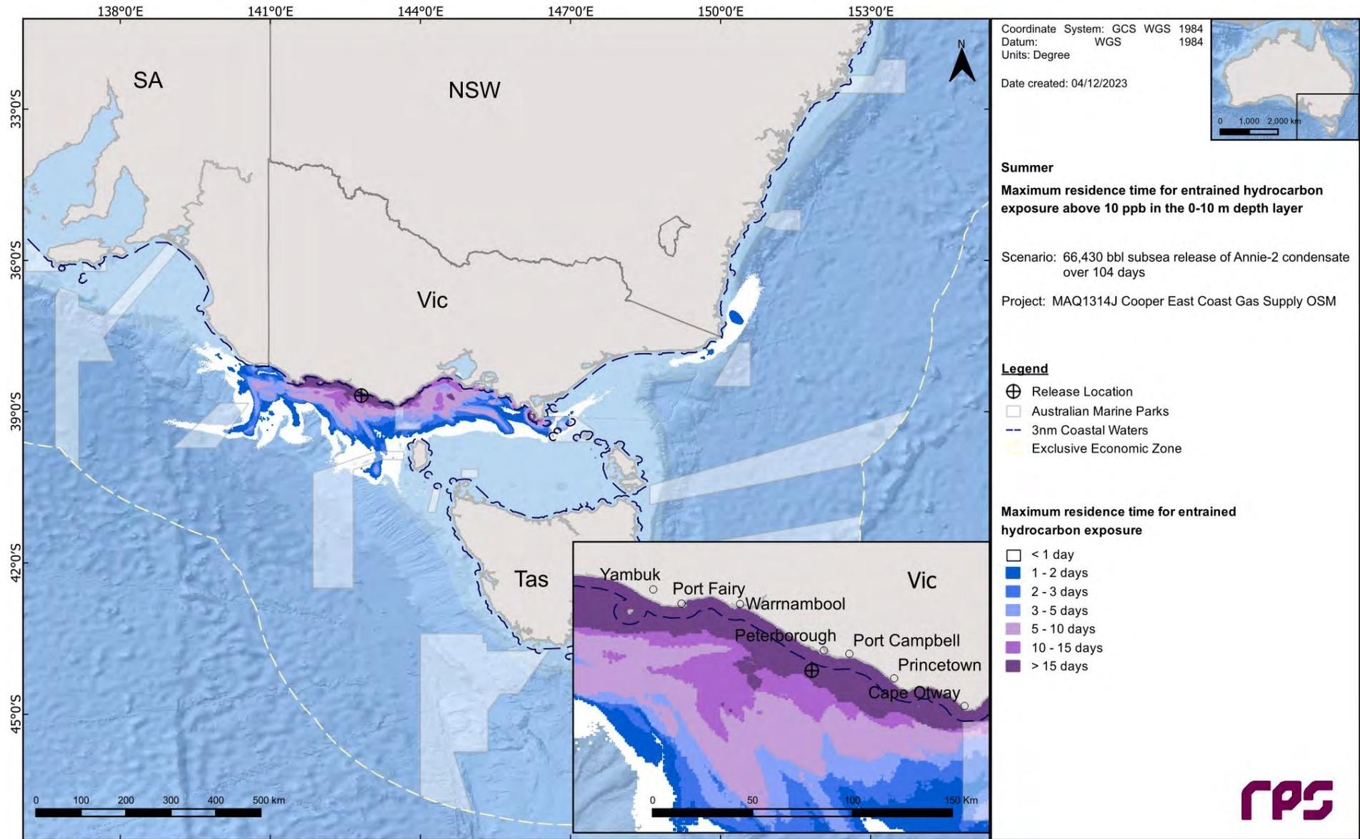
**Figure 13.15** Maximum residence time for entrained hydrocarbon exposure above 10 ppb, at 0-10 m below the sea in the event of a 66,430 bbl subsurface release from a loss of well control at Annie-2 over 104 days. The results were calculated from 100 spill simulations during summer conditions.
