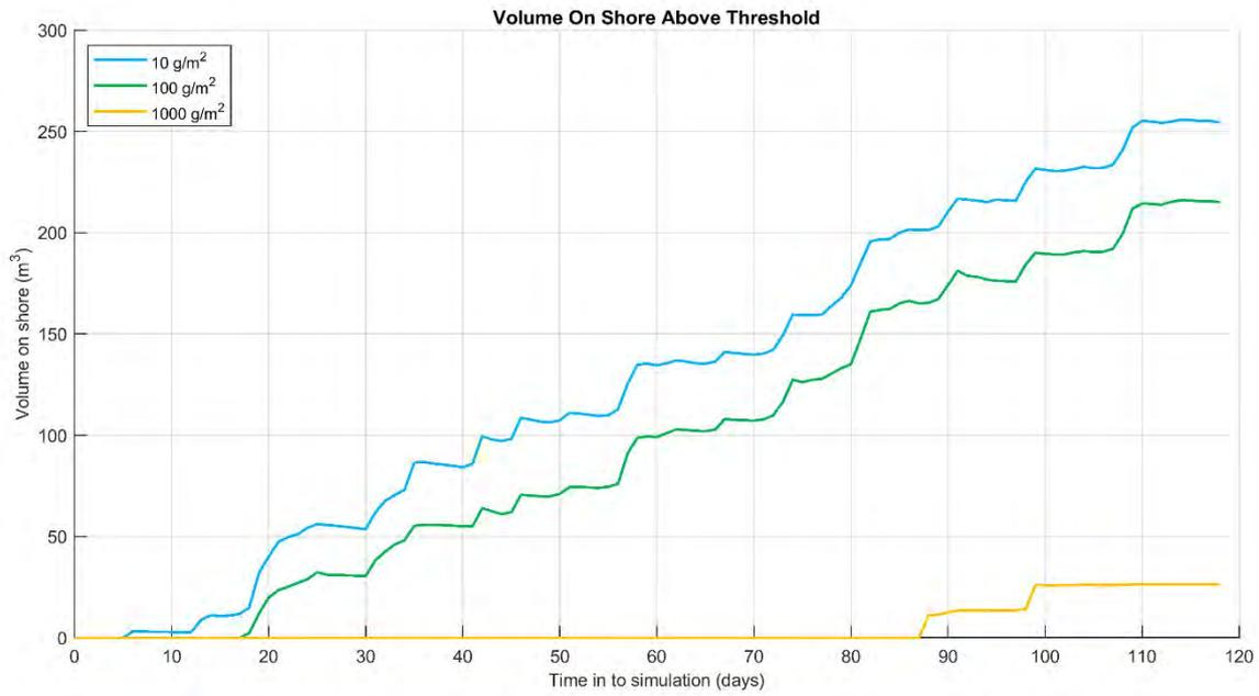
**Figure 13.23** Time series of oil accumulation on the shoreline above each threshold for the trajectory with the largest volume ashore and the longest length of shoreline with accumulation above 100 g/m<sup>2</sup>.
