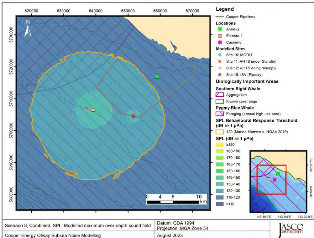
Figure 23. Scenario 8, Drilling and standby OSV during resupply and pipelay – end, Elanora-1 and Casino-5, SPL: Sound level contour map showing the unweighted maximum-over-depth sound field in 10 dB steps, and the isopleths for behavioural response threshold for marine mammals.
