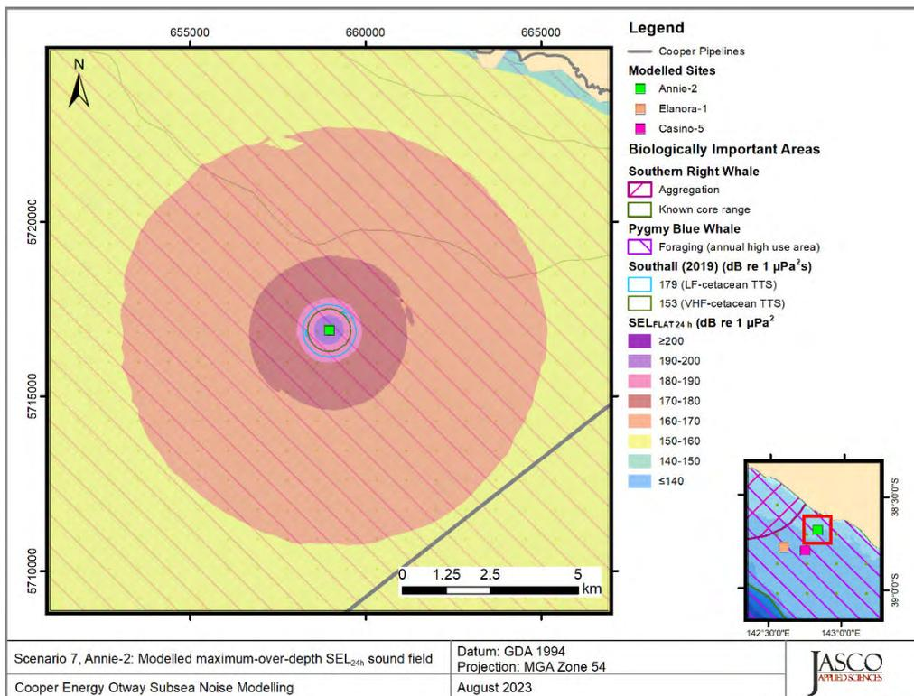
Figure 35. Scenario 7, Installation, Annie-2, accumulated  $SEL_{24h}$ : Sound level contour map showing weighted maximum-over-depth  $SEL_{24h}$  results, along with isopleths for TTS in low and very-high-frequency cetaceans. Thresholds omitted here were not reached or not long enough to display graphically.
