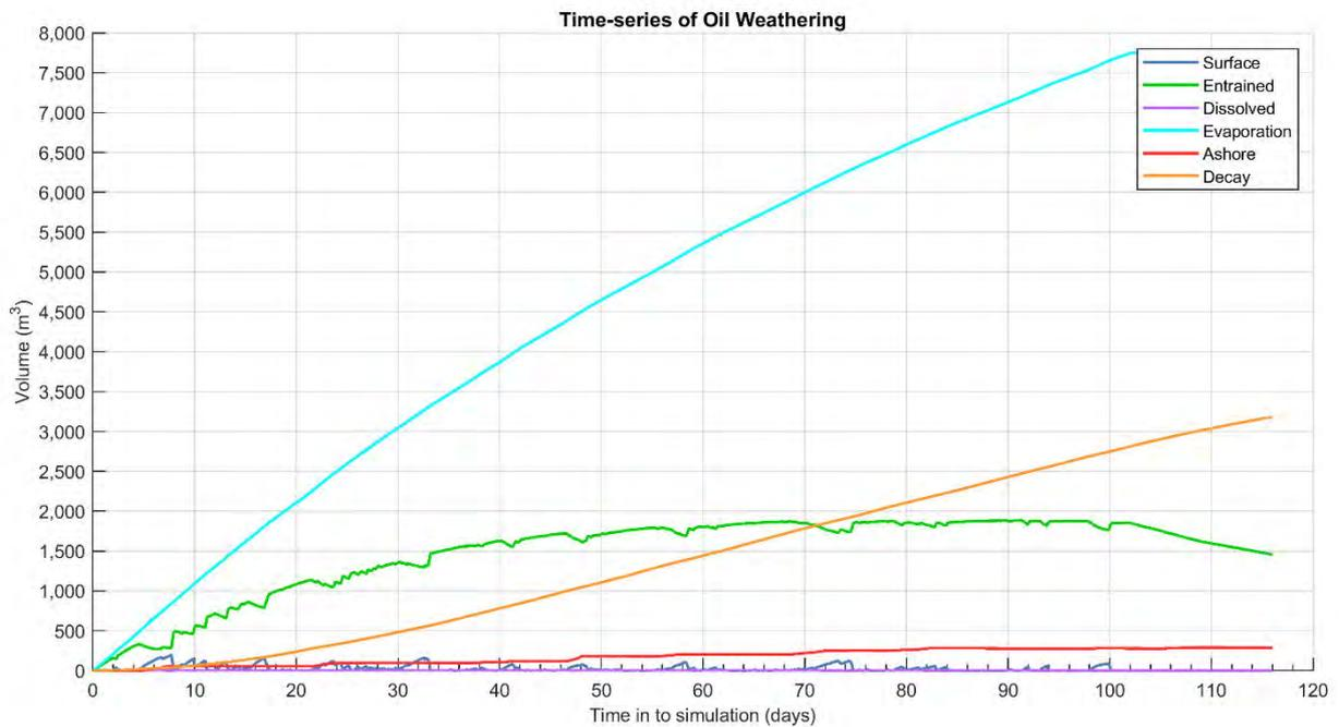
Figure 12.27 Predicted weathering and fates graph for the trajectory with the longest length of shoreline with accumulation above 100 g/m<sup>2</sup>.
