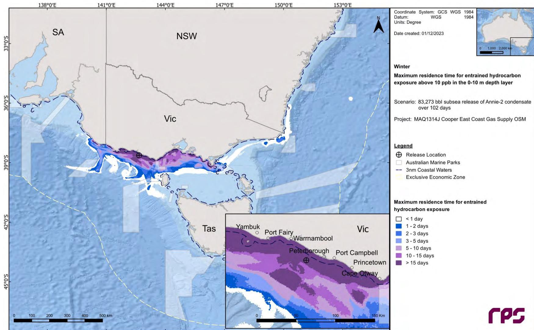
**Figure 12.16** Maximum residence time for entrained hydrocarbon exposure above 10 ppb, at 0-10 m below the sea in the event of an 83,273 bbl subsurface release from a loss of well control at Pecten East-2 over 102 days. The results were calculated from 100 spill simulations during winter conditions.
