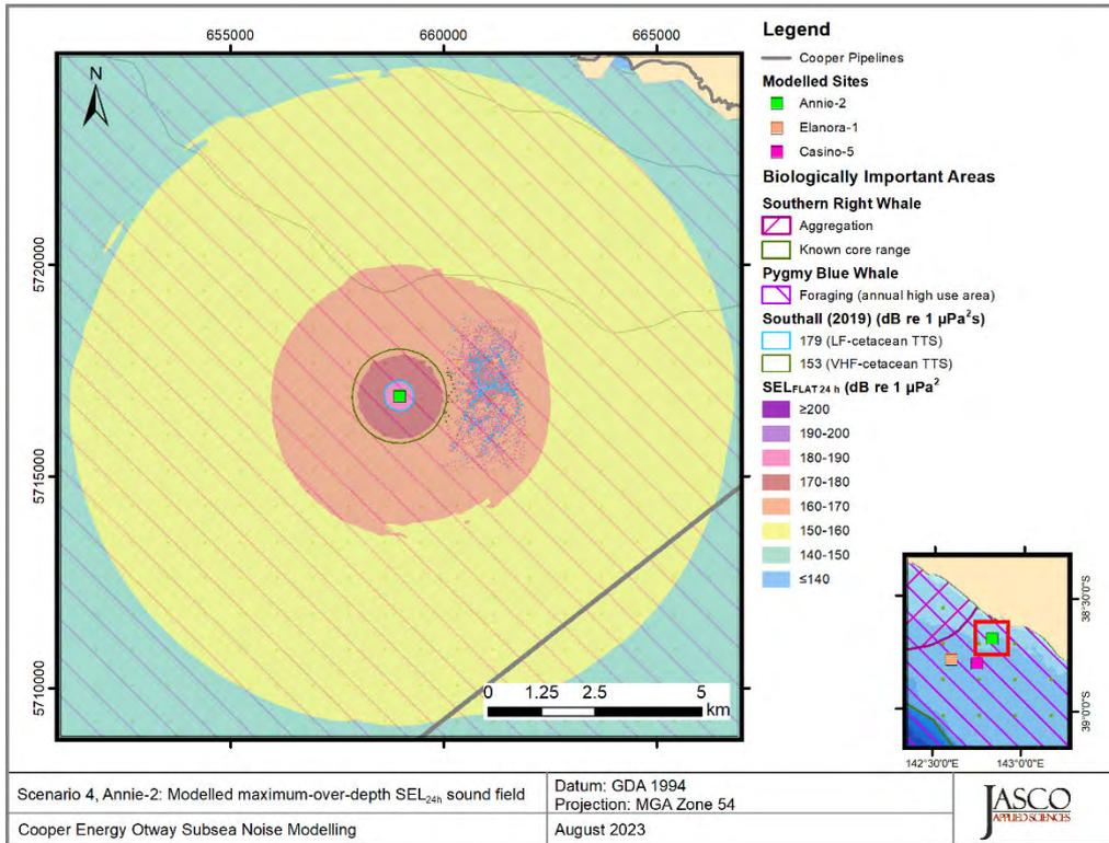
Figure 30. Scenario 4, Drilling and standby OSV, Annie-2, accumulated SEL<sub>24h</sub>: Sound level contour map showing weighted maximum-over-depth SEL<sub>24h</sub> results, along with isopleths for TTS in low and very-high-frequency cetaceans. Thresholds omitted here were not reached or not long enough to display graphically.
