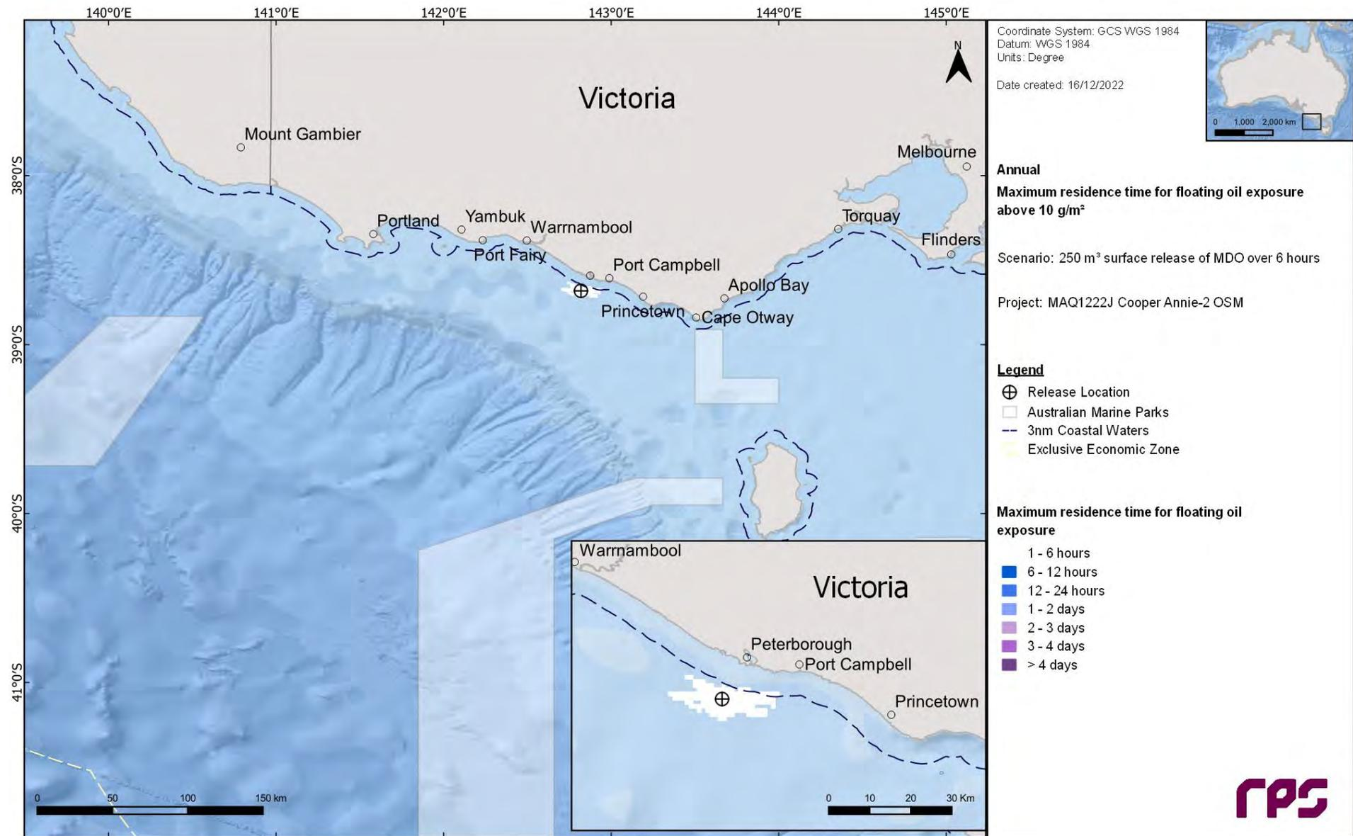
Figure 10.4 Maximum residence time of floating oil exposure above 10 g/m<sup>2</sup>, in the event of a 250 m<sup>3</sup> of MDO containment loss over 6 hours tracked for 30 days. The results were calculated from 100 spill simulations.
