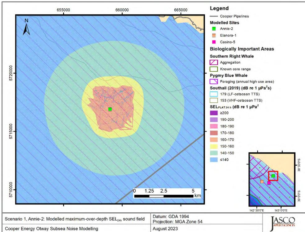
Figure 24. Scenario 1, Drilling prelays, Annie-2, accumulated SEL<sub>24h</sub>: Sound level contour map showing weighted maximum-over-depth SEL<sub>24h</sub> results, along with isopleths for TTS in low and very-high-frequency cetaceans. Thresholds omitted here were not reached or not long enough to display graphically.
