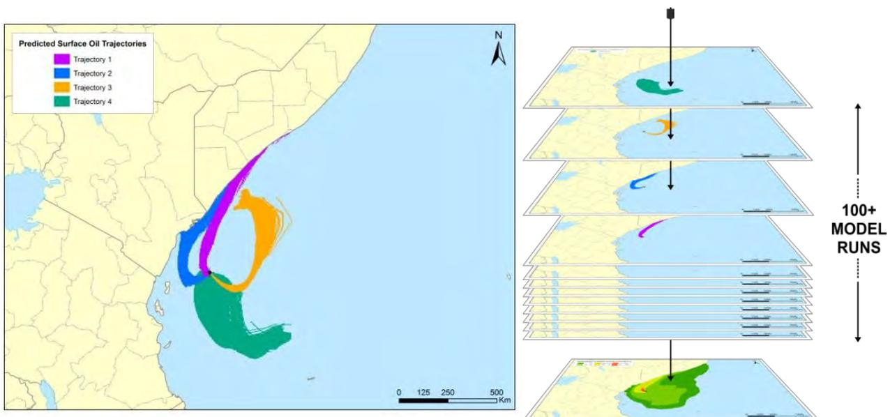
**Figure 1.2** Examples of four individual spill trajectories (four replicate simulations) predicted by SIMAP for a spill scenario. The frequency of contact with given locations is used to calculate the probability of impacts during a spill. Essentially, all model runs are overlain (shown as the stacked runs on the right) and the number of times that trajectories contact a given location at a concentration is used to calculate the probability.
