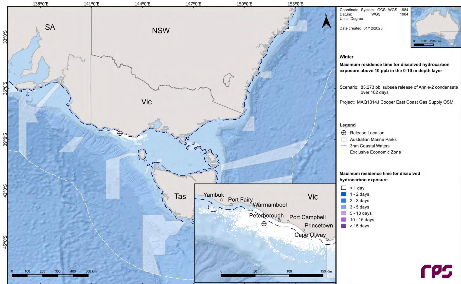
**Figure 12.12 Maximum residence time for dissolved hydrocarbon exposure above 10 ppb, at 0-10 m below the sea surface in the event of an 83,273 bbl subsurface release from a loss of well control at Pecten East-2 over 102 days. The results were calculated from 100 spill simulations during winter conditions.**
