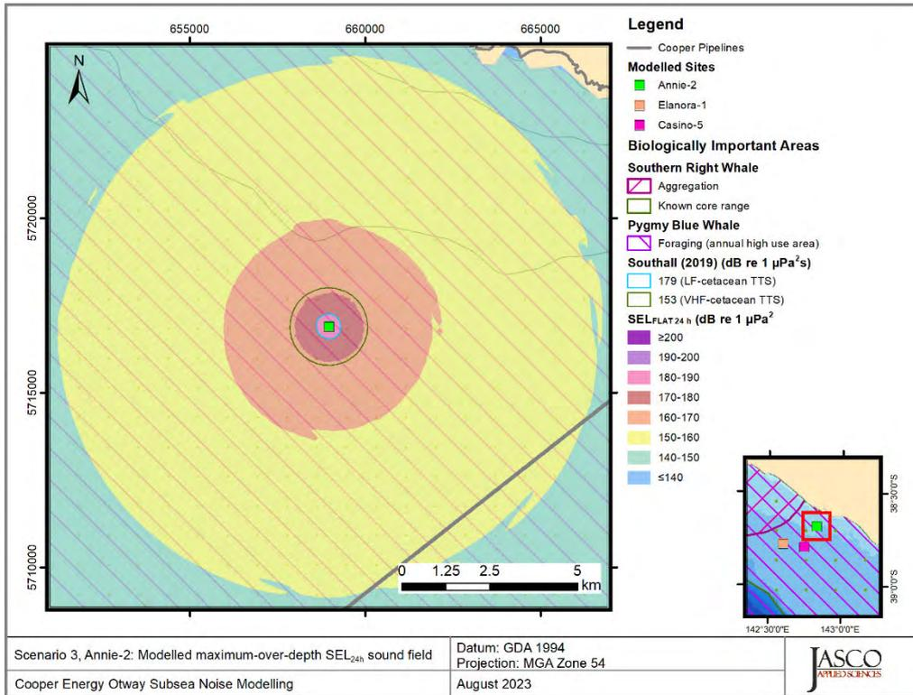
Figure 28. Scenario 3, MODU Drilling, Annie-2, accumulated SEL<sub>24h</sub>: Sound level contour map showing weighted maximum-over-depth SEL<sub>24h</sub> results, along with isopleths for TTS in low and very-high-frequency cetaceans. Thresholds omitted here were not reached or not long enough to display graphically.
