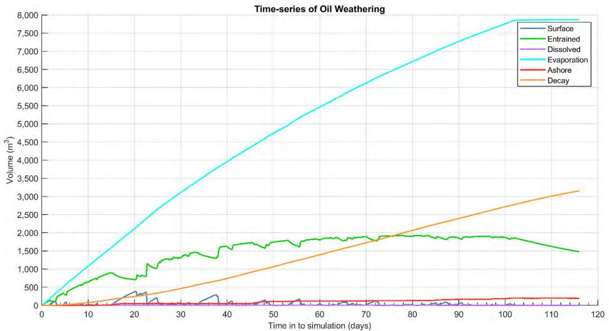
**Figure 12.21** Predicted weathering and fates graph for the trajectory with the largest swept area of floating oil above 10 g/m<sup>2</sup>.
