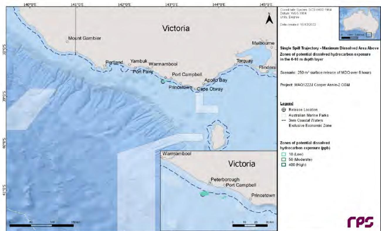
**Figure 10.26 Zones of potential dissolved hydrocarbon exposure, for the trajectory with the largest area of dissolved hydrocarbon exposure above 50 ppb. Results are based on a 250 m<sup>3</sup> surface release of MDO over 6 hours, tracked for 30 days.**
