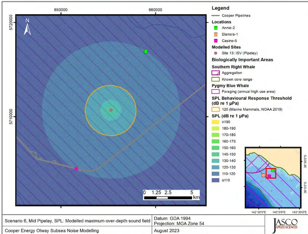
Figure 18. Scenario 6, Pipelay installation – mid, Casino-5, SPL: Sound level contour map showing the unweighted maximum-over-depth sound field in 10 dB steps, and the isopleths for behavioural response threshold for marine mammals.
