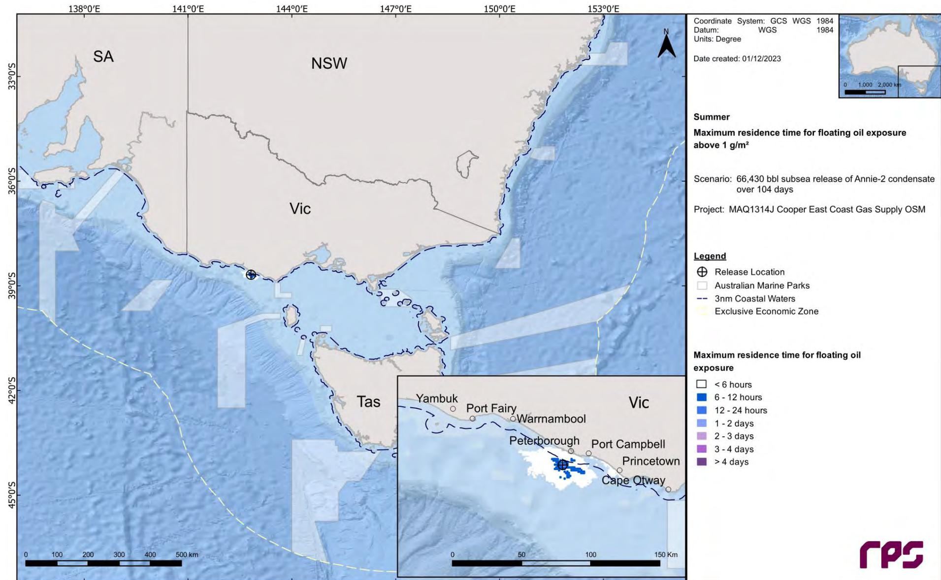
Figure 13.3 Maximum residence time of floating oil exposure above 1 g/m<sup>2</sup>, in the event of a 66,430 bbl subsurface release from a loss of well control at Annie-2 over 104 days. The results were calculated from 100 spill simulations during summer conditions.
