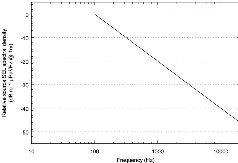
Figure B-3. Estimated sound spectrum from cavitating propeller (Leggat et al. 1981).
