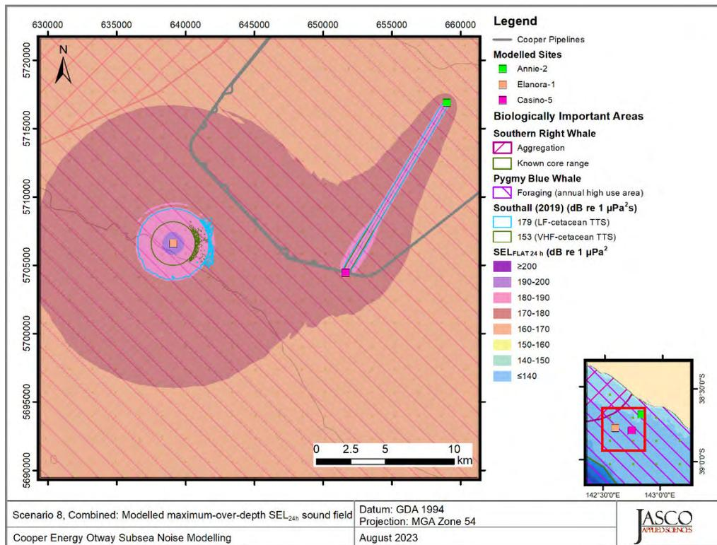
Figure 36. Scenario 8, Drilling and standby OSV during resupply and pipelay, Elanora-1 and between Annie-2 and Casino-5, accumulated SEL<sub>24h</sub>: Sound level contour map showing weighted maximum-over-depth SEL<sub>24h</sub> results, along with isopleths for TTS in low and very-high-frequency cetaceans. Thresholds omitted here were not reached or not long enough to display graphically.
