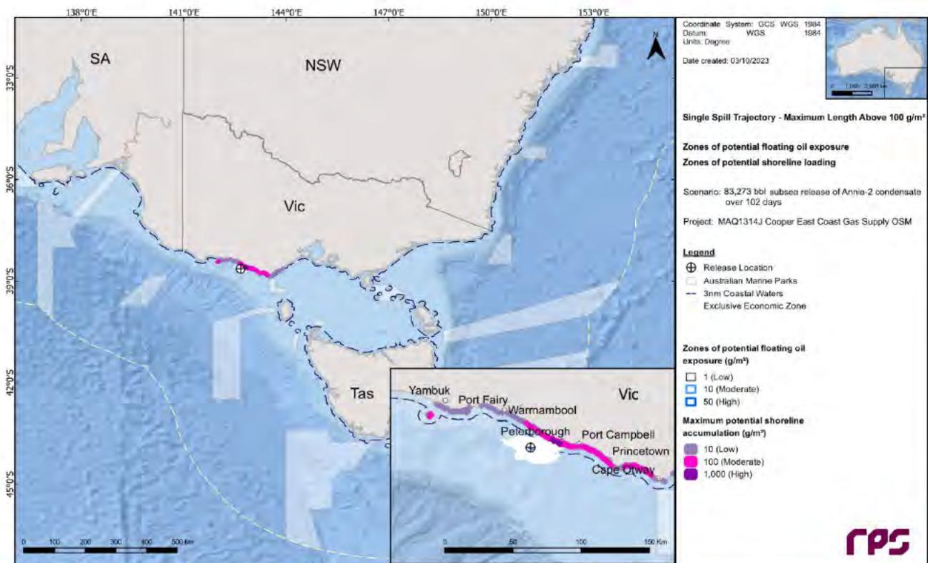
**Figure 12.25 Zones of potential floating oil exposure and shoreline accumulation, for the trajectory with the longest length of shoreline with accumulation above 100 g/m<sup>2</sup>.**
