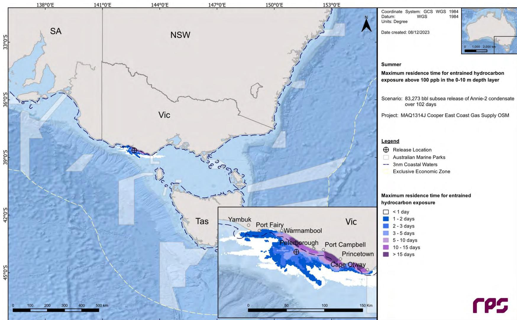
**Figure 12.17 Maximum residence time for entrained hydrocarbon exposure above 100 ppb, at 0-10 m below the sea in the event of an 83,273 bbl subsurface release from a loss of well control at Pecten East-2 over 102 days. The results were calculated from 100 spill simulations during summer conditions.**
