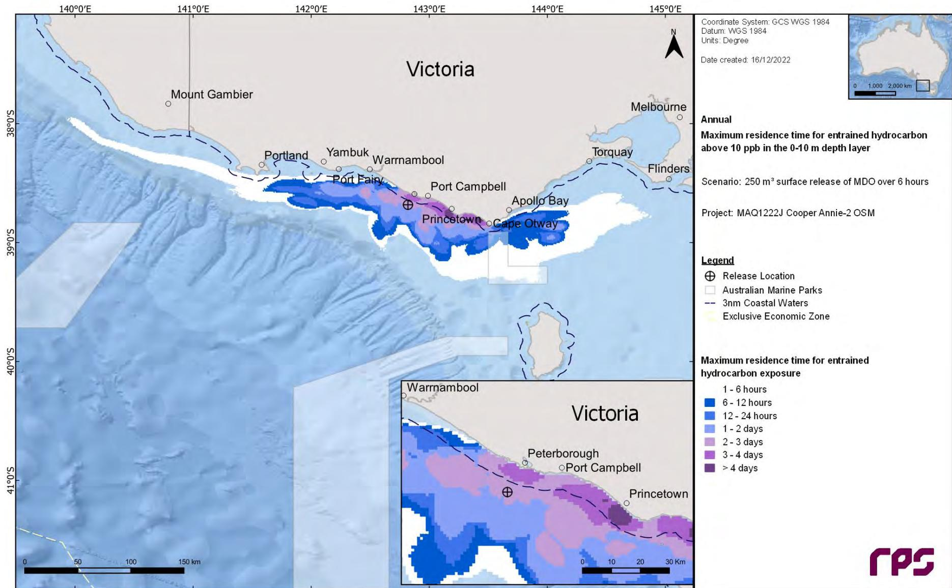
Figure 10.11 Maximum residence time for entrained hydrocarbon exposure above 10 ppb, at 0-10 m below the sea in the event of a 250 m<sup>3</sup> of MDO containment loss over 6 hours tracked for 30 days. The results were calculated from 100 spill simulations.
