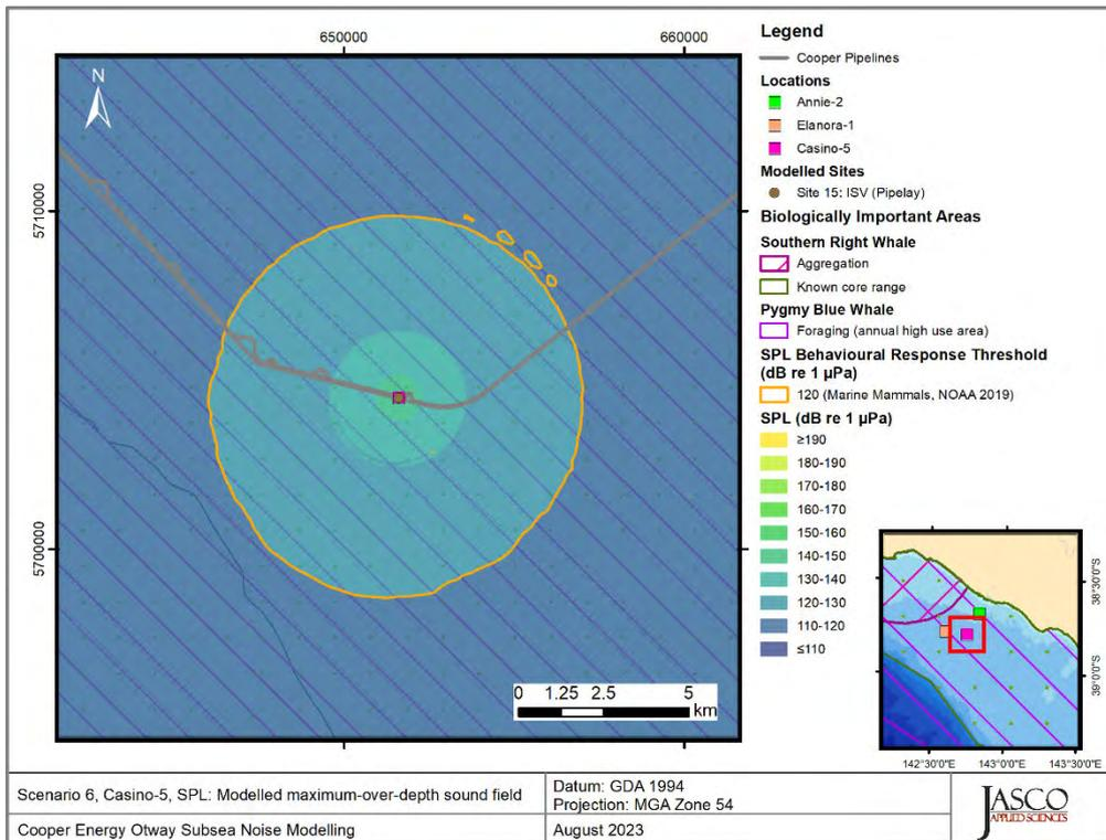
Figure 19. Scenario 6, Pipelay installation – end, Casino-5, SPL: Sound level contour map showing the unweighted maximum-over-depth sound field in 10 dB steps, and the isopleths for behavioural response threshold for marine mammals.
