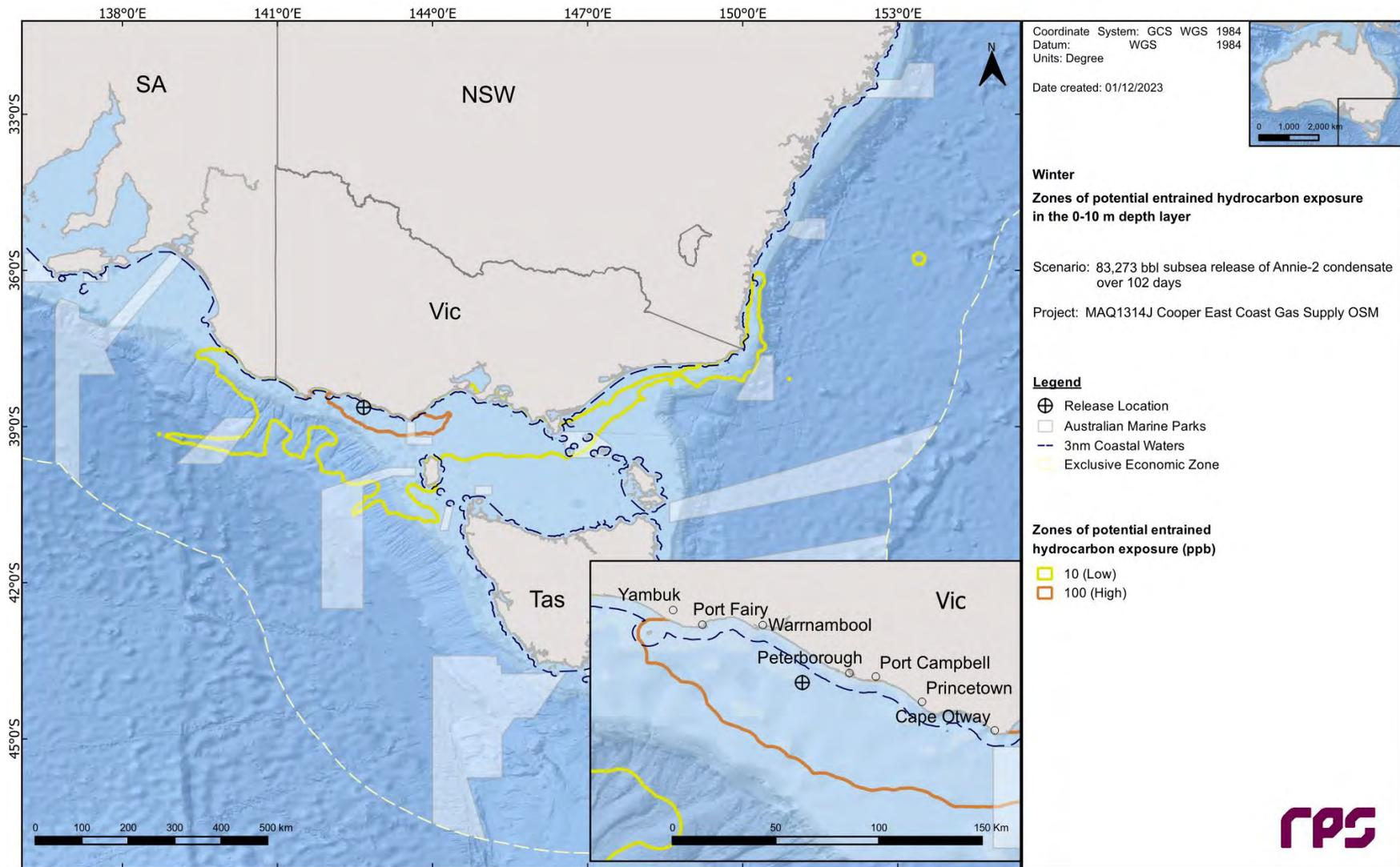
**Figure 12.14** Zones of potential entrained hydrocarbon exposure at 0-10 m below the sea surface in the event of an 83,273 bbl subsurface release from a loss of well control at Pecten East-2 over 102 days. The results were calculated from 100 spill simulations during winter conditions.
