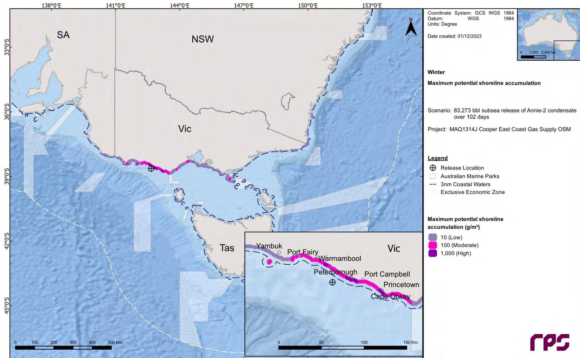
**Figure 12.8** Maximum potential shoreline accumulation in the event of an 83,273 bbl subsurface release from a loss of well control at Pecten East-2 over 102 days. The results were calculated from 100 spill simulations during winter conditions.
