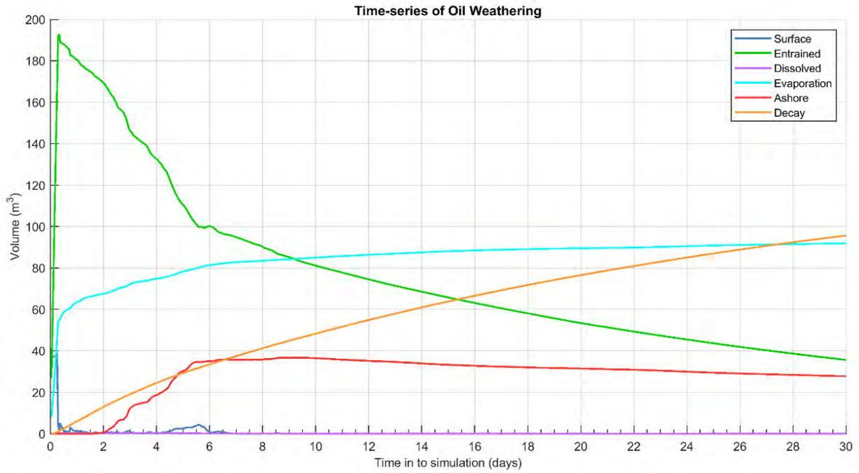
**Figure 10.22 Predicted weathering and fates graph for the trajectory with the largest volume ashore and longest length of shoreline with accumulation above 100 g/m<sup>2</sup>. Results are based on a 250 m<sup>3</sup> surface release of MDO over 6 hours, tracked for 30 days.**
