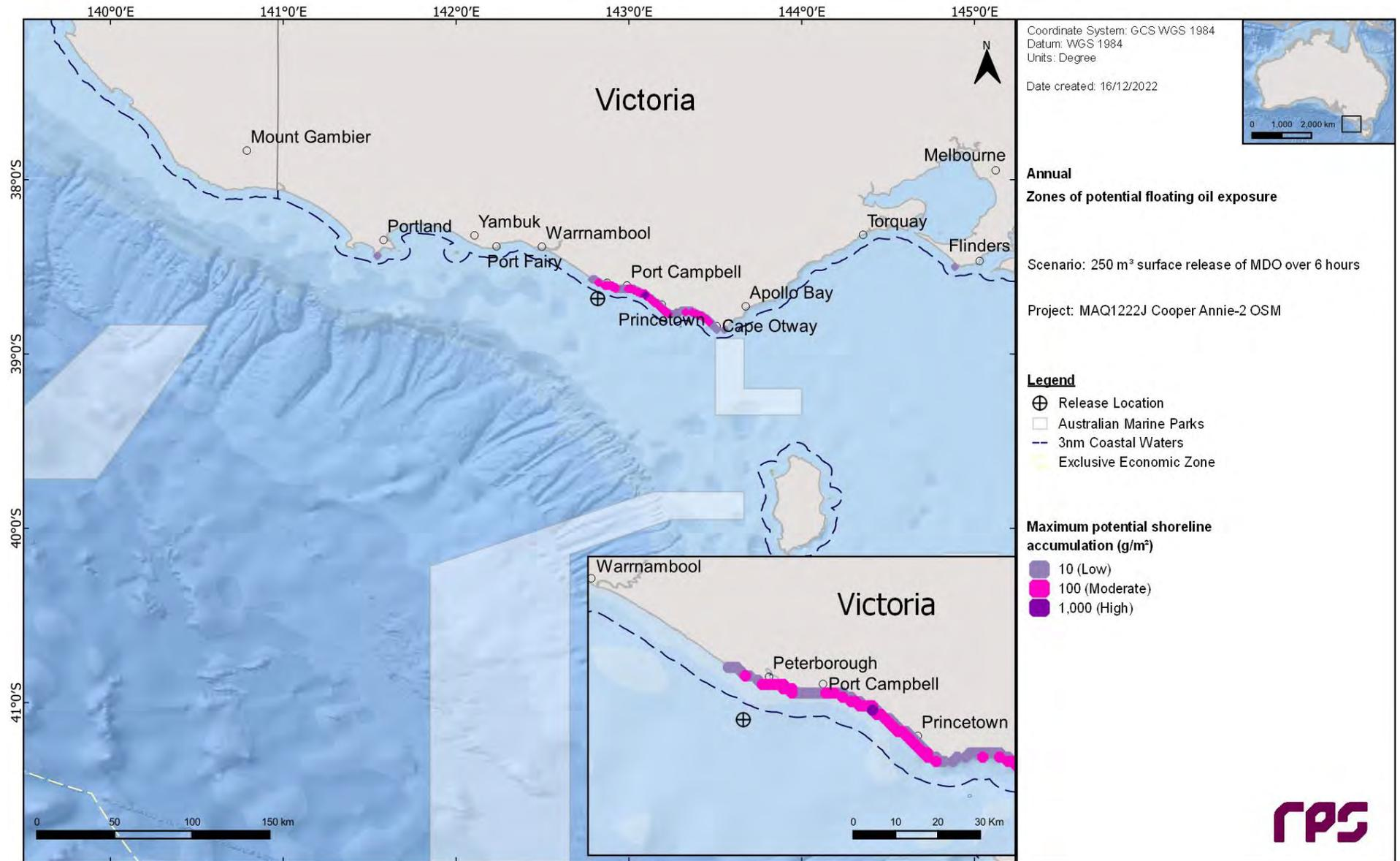
**Figure 10.6** Maximum potential shoreline loading in the event of a 250 m<sup>3</sup> of MDO containment loss over 6 hours tracked for 30 days. The results were calculated from 100 spill simulations.
