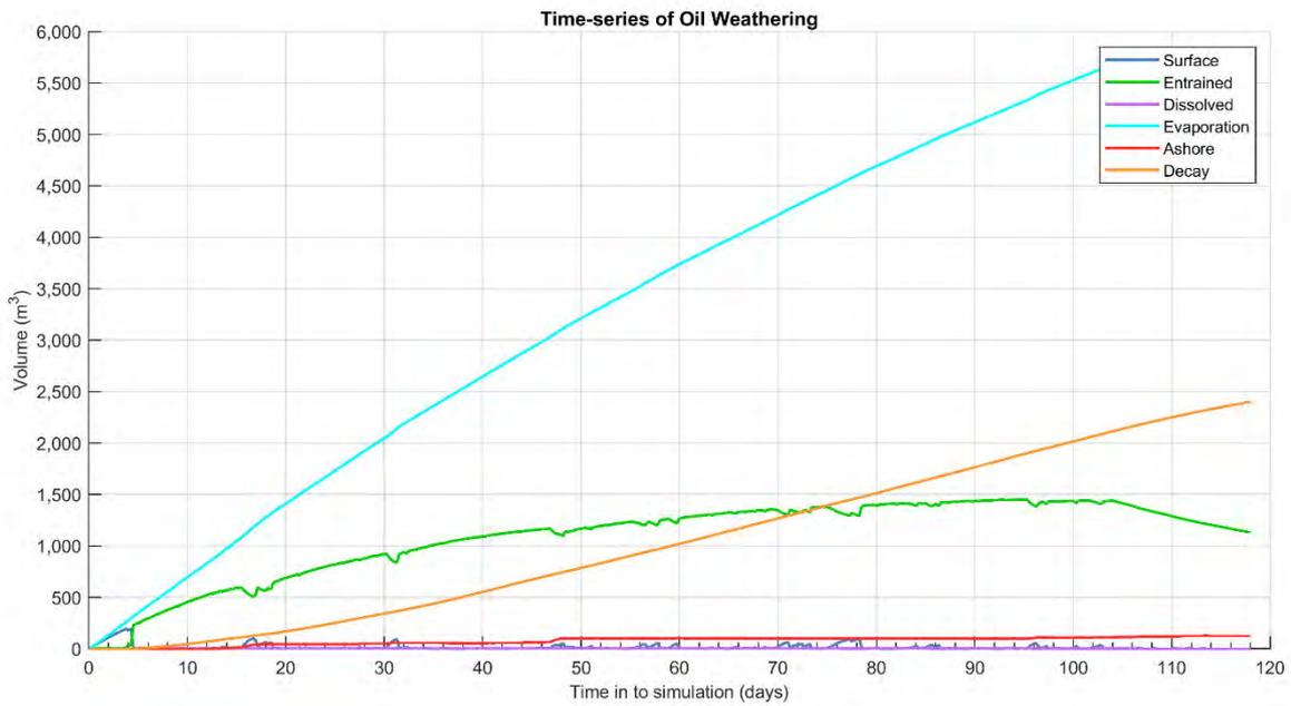
**Figure 13.21** Predicted weathering and fates graph for the trajectory with the largest swept area of floating oil above 10 g/m<sup>2</sup>.
