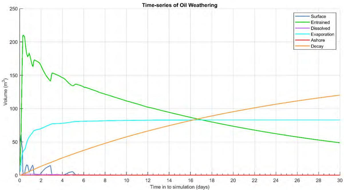
**Figure 10.28** Predicted weathering and fates graph for the trajectory with the largest area of dissolved hydrocarbon exposure above 50 ppb. Results are based on a 250 m<sup>3</sup> surface release of MDO over 6 hours, tracked for 30 days.
