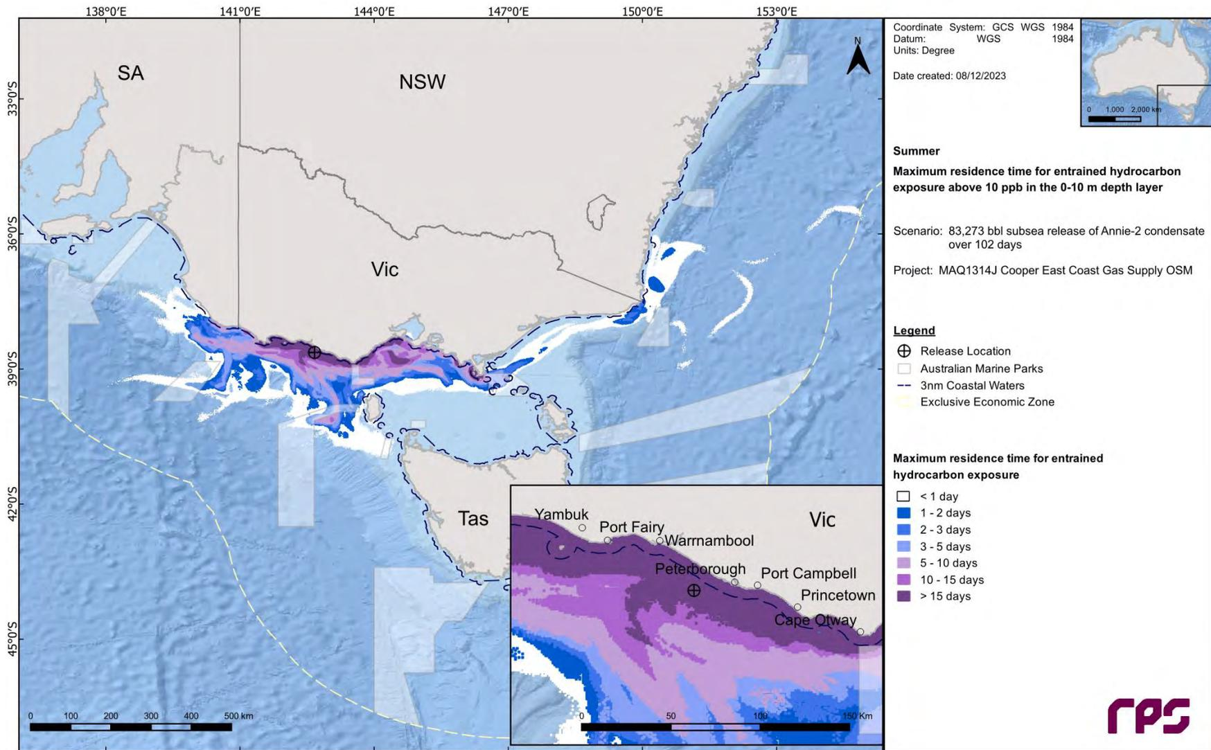
**Figure 12.15** Maximum residence time for entrained hydrocarbon exposure above 10 ppb, at 0-10 m below the sea in the event of an 83,273 bbl subsurface release from a loss of well control at Pecten East-2 over 102 days. The results were calculated from 100 spill simulations during summer conditions.
