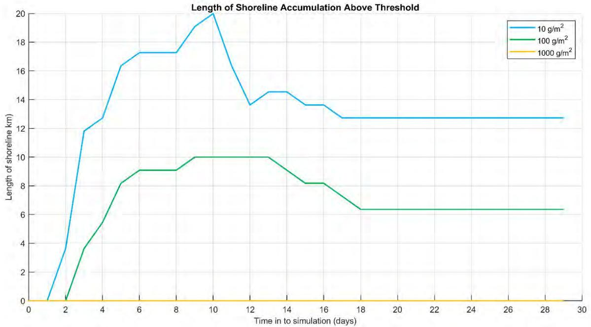
**Figure 10.20** Time series of the length of shoreline with accumulation above each threshold for the trajectory with the largest volume ashore and longest length of shoreline with accumulation above 100 g/m<sup>2</sup>. Results are based on a 250 m<sup>3</sup> surface release of MDO over 6 hours, tracked for 30 days.
