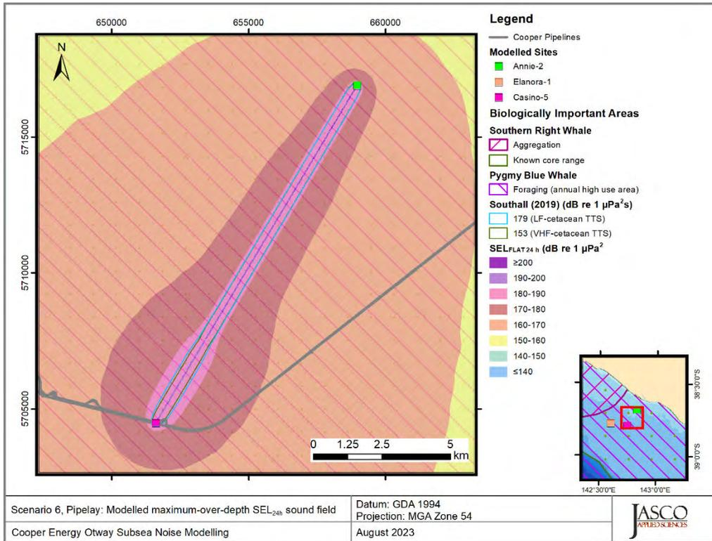
Figure 34. Scenario 6, Pipeline/Umbilical installation, Annie-2 & Casino-5, accumulated  $SEL_{24h}$ : Sound level contour map showing weighted maximum-over-depth  $SEL_{24h}$  results, along with isopleths for TTS in low and very-high-frequency cetaceans. Thresholds omitted here were not reached or not long enough to display graphically.
