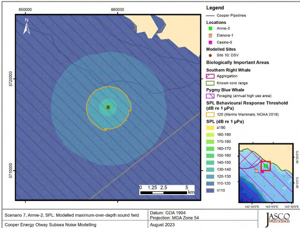
Figure 20. Scenario 7, Installation, Annie-2, SPL: Sound level contour map showing the unweighted maximum-over-depth sound field in 10 dB steps, and the isopleths for behavioural response threshold for marine mammals.
