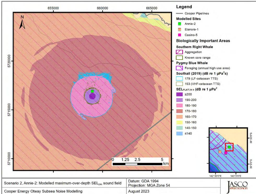
Figure 26. Scenario 2, Mooring, Annie-2, accumulated  $SEL_{24h}$ : Sound level contour map showing weighted maximum-over-depth  $SEL_{24h}$  results, along with isopleths for TTS in low and very-high-frequency cetaceans. Thresholds omitted here were not reached or not long enough to display graphically.
