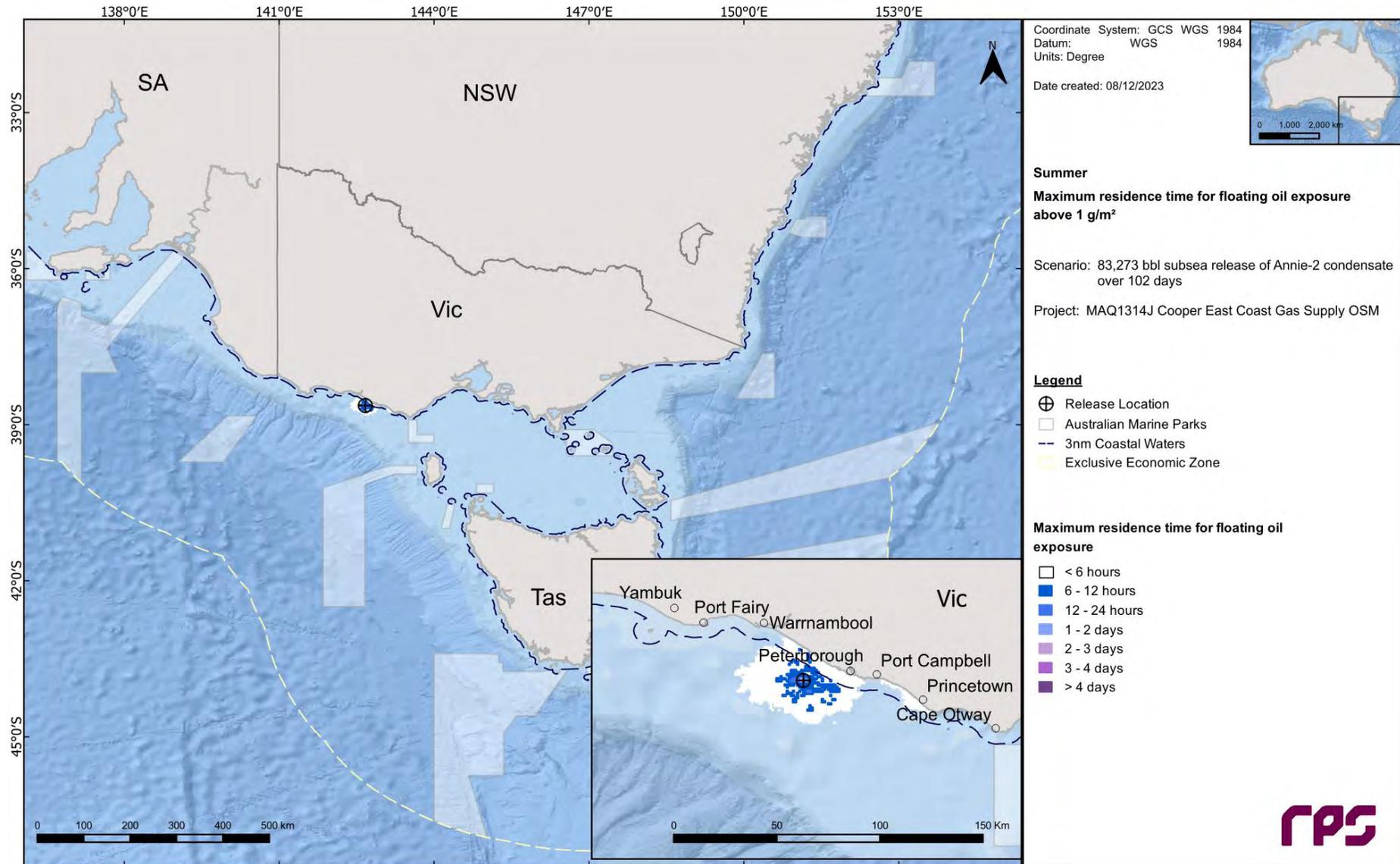
Figure 12.3 Maximum residence time of floating oil exposure above 1 g/m<sup>2</sup>, in the event of an 83,273 bbl subsurface release from a loss of well control at Pecten East-2 over 102 days. The results were calculated from 100 spill simulations during summer conditions.
