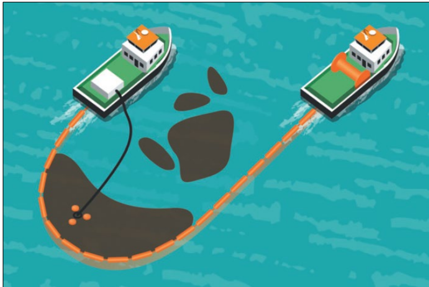
Figure 13-1: ‘J’ Configuration for Containment and Recovery Operations
