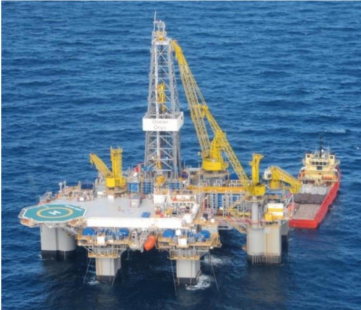
Figure 3. *Ocean Onyx* semi-submersible platform.
