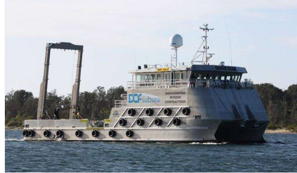
Figure 2-4: The "Silver Star" - typical vessel for pipeline surveys
