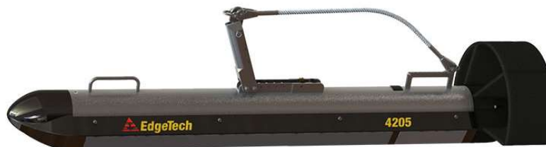
Figure 2-6: An example 'towfish' retained for Offshore Oil & Gas Pipeline route surveys
