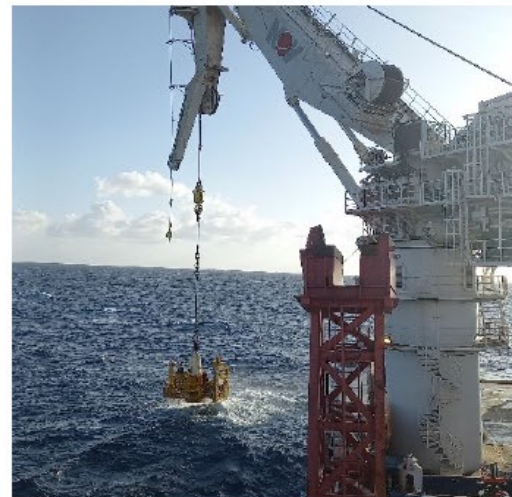
Figure 4. Typical Subsea Equipment Recovery Activity
