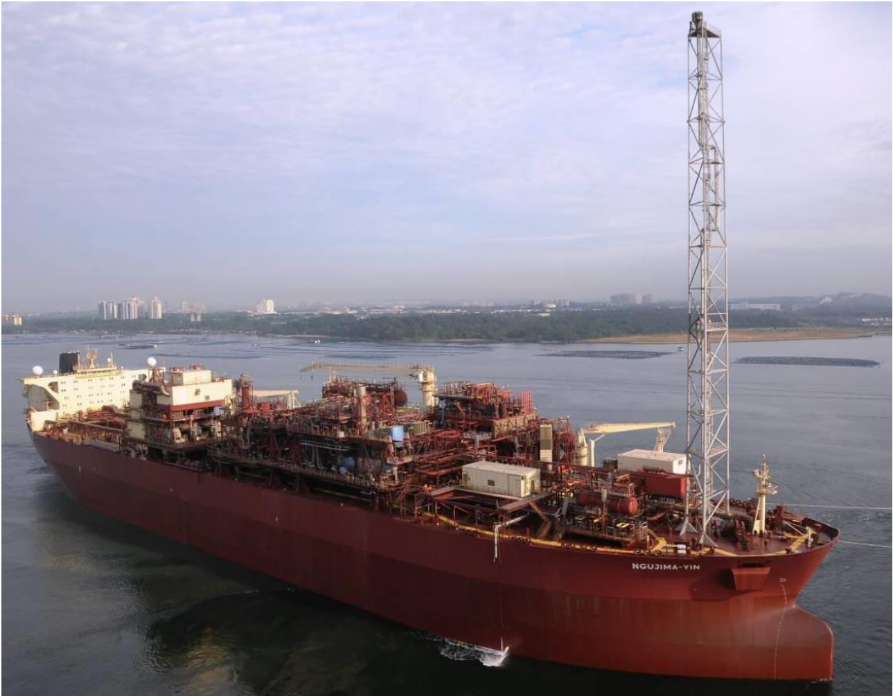
Figure 3-1: Ngujima-Yin floating production, storage and offloading facility
