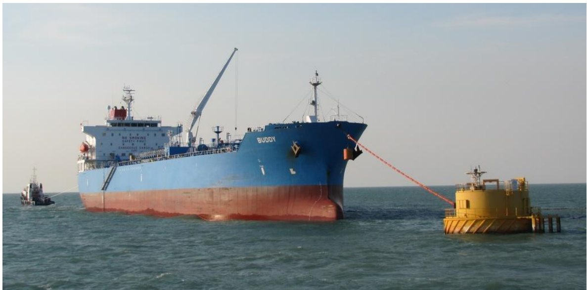
Figure 3.10: Tanker moored to single point mooring for condensate offtake
