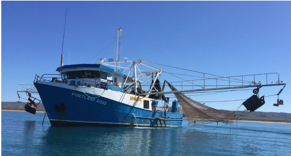
Figure 7. FV Portland Road. A 24m steel trawler that works full-time as a prawn trawler, and opportunistically fishes part-time in the PFT.
