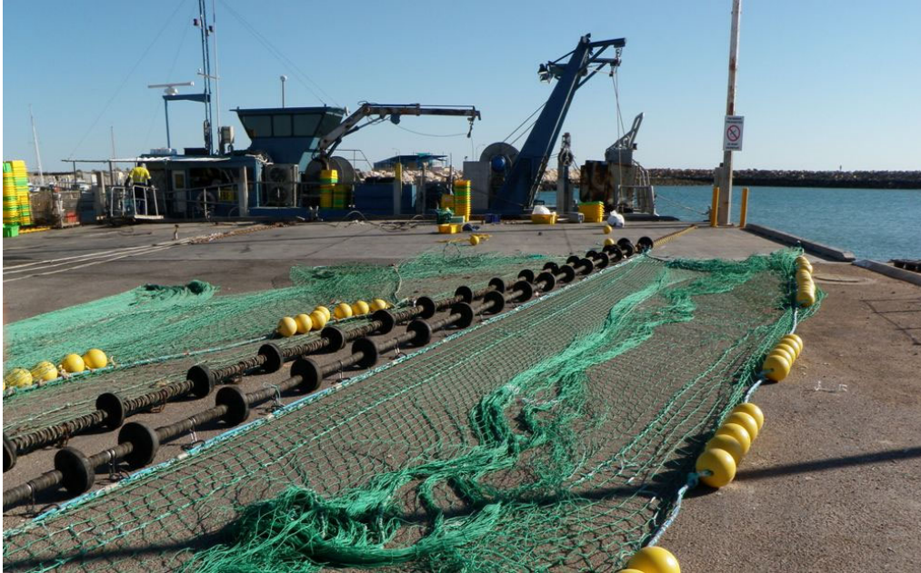
Figure 9. A PFT trawl net stretched out for repairs, showing 10-inch rubber disc ground-gear and clusters of 8-inch pneumatic floats attached to the lower (footrope) and upper (headrope) framelines respectively. (Source: Fishing Untangled Pty Ltd. )
