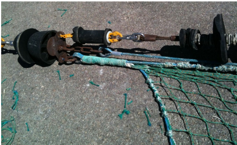
Figure 10. The lower wingtip of a PFT trawl net showing the rubber half bobbin (extreme left) that serves to protect the connection tackle and "hard eyes" located at the terminal end of the ground-wire (upper wire), bolsch-line (middle blue combo rope) and footrope (lower wrapped combo rope) from interactions with seabed obstacles.
