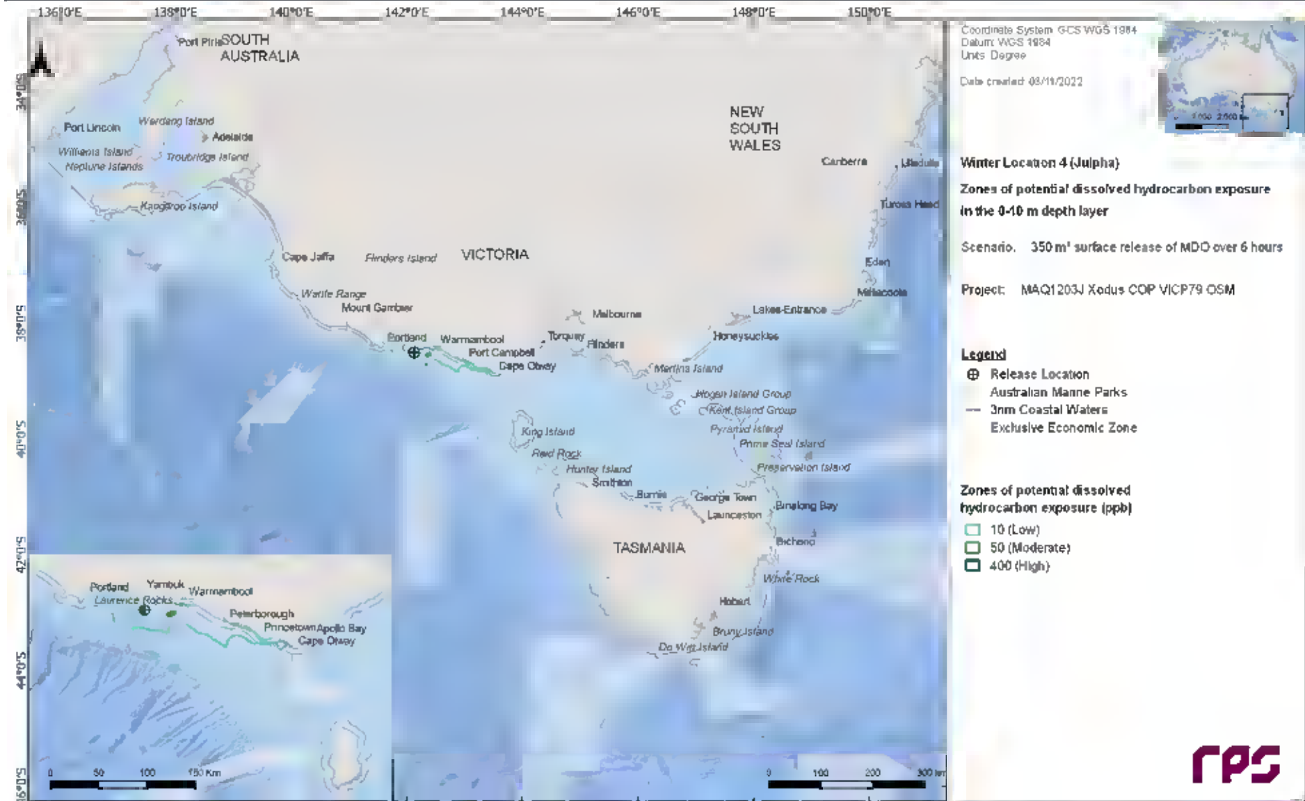
Figure 20.7 Zones of potential dissolved hydrocarbon exposure at 0-10 m below the sea surface from a vessel collision at Location 4 during winter conditions. The results were calculated from 100 spill simulations.
