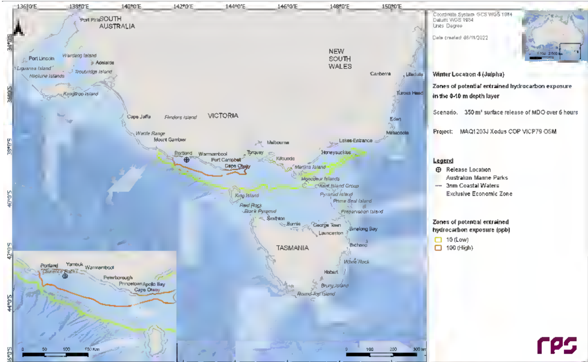
Figure 20.9 Zones of potential entrained hydrocarbon exposure at 0-10 m below the sea surface from a vessel collision at Location 4 during winter conditions. The results were calculated from 100 spill simulations.
