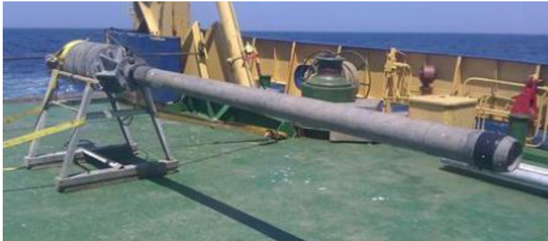
Photo 2-12 Typical gravity corer
