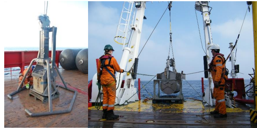
Photo 2-9 Box corer deployment
