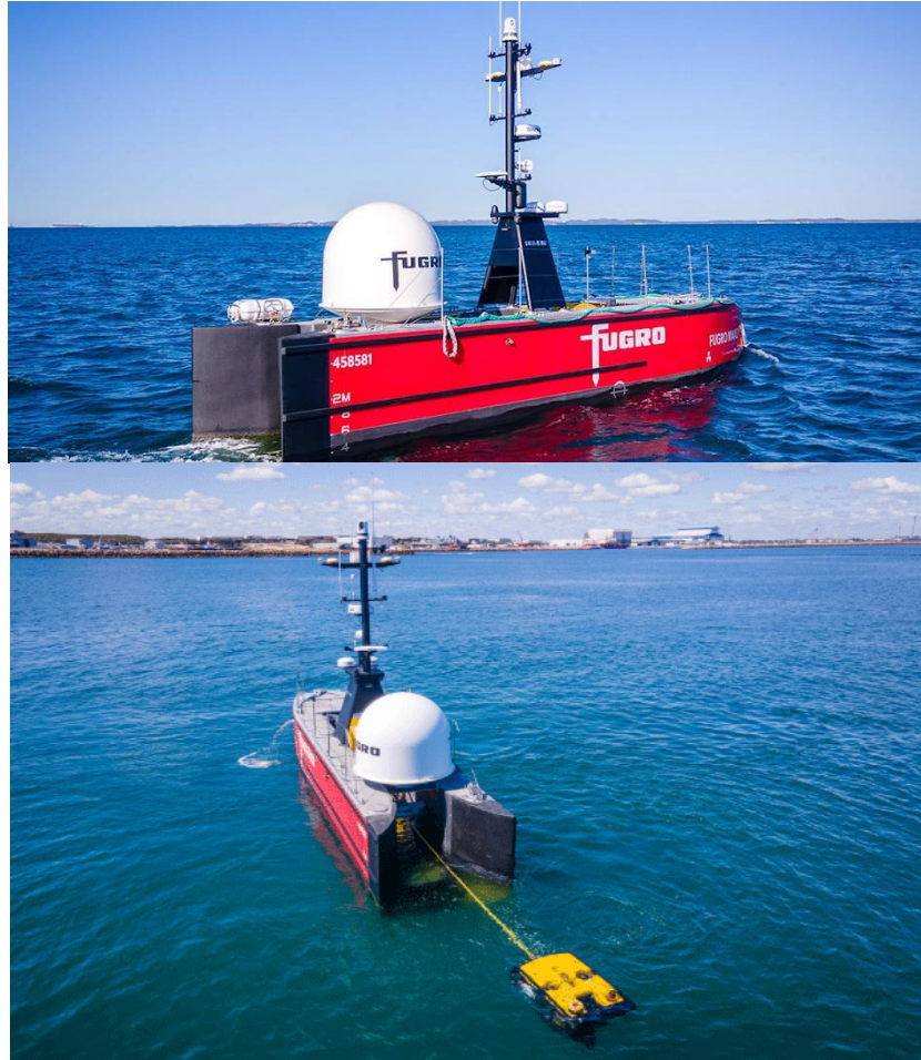
Figure 3-5: Example uncrewed survey vessel (above) and with ROV in tow (bottom).
