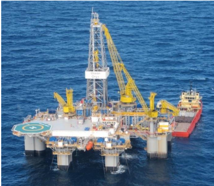
Figure 2. Ocean Onyx semi-submersible platform.
