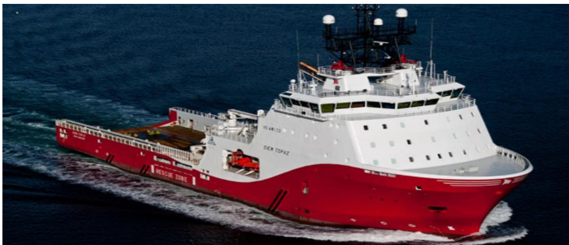
Figure 3-6: Example of an Anchor Handling Tug
