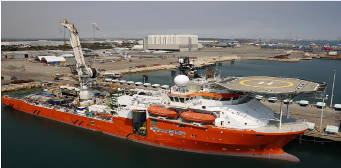
Figure 3-10: Example of an Inspection, Maintenance, Repair Vessel
