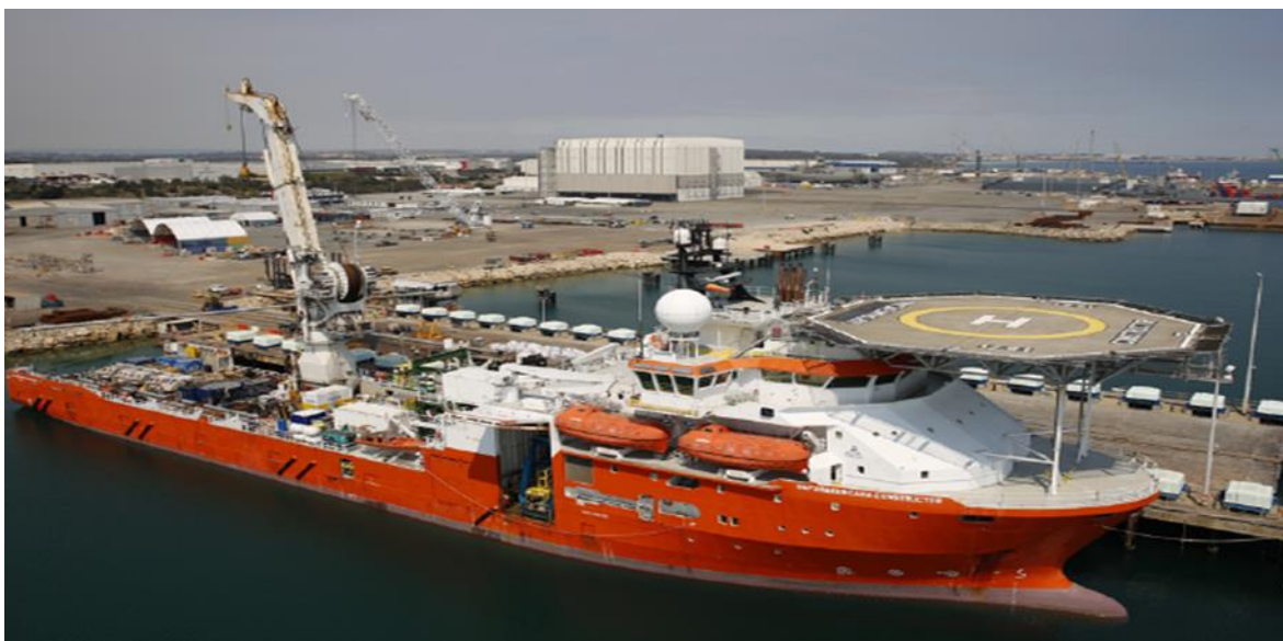
Figure 3-8: Example of a Pipelay/Multipurpose Service Vessel
