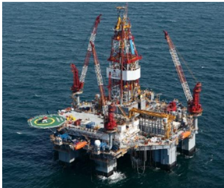
Figure 3-5: Representative Semi-submersible MODU
