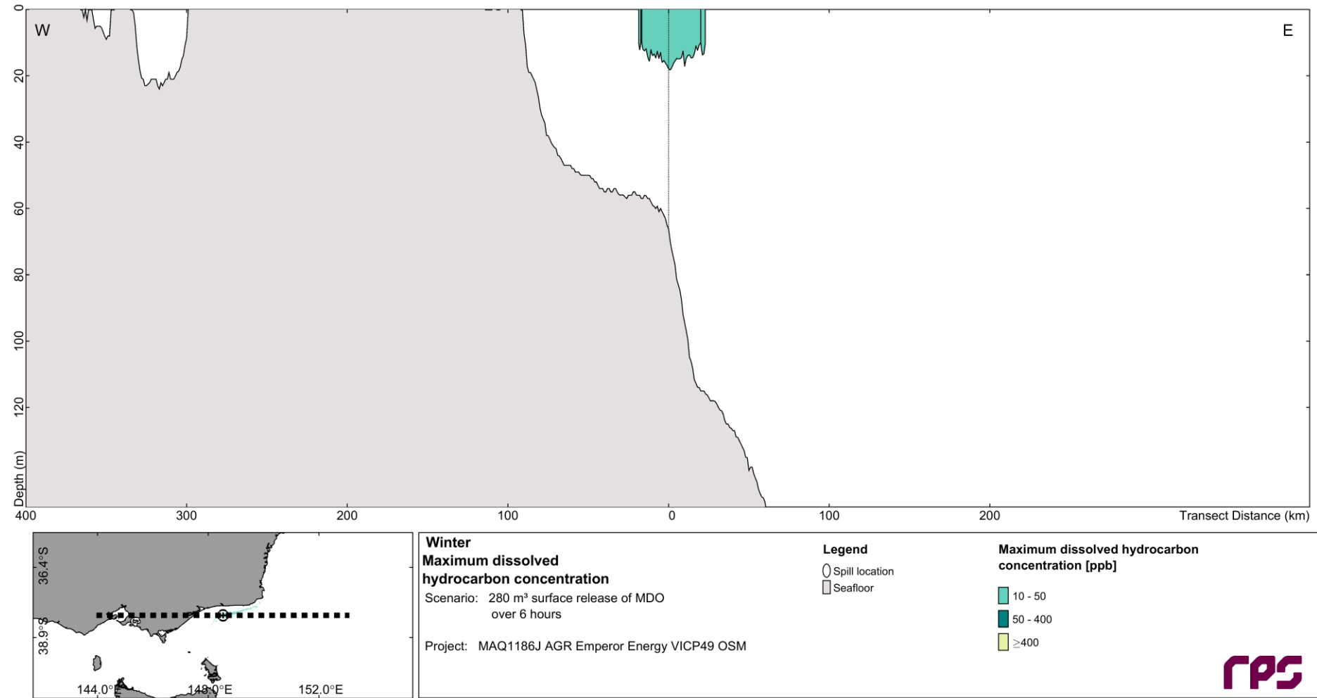
Figure 13.10 North-south cross-section transect of dissolved hydrocarbon concentrations from a vessel collision during winter conditions. The results were calculated from 100 spill simulations.
