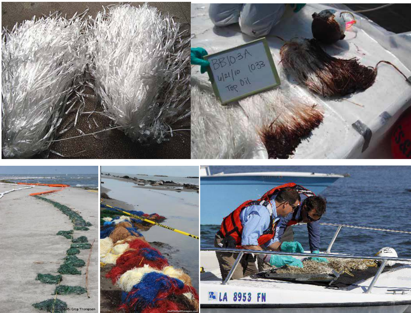
Figure-4: Examples of polypropylene snare booms and “pom-poms” used to absorb and trap oil in the near-shore zone.
