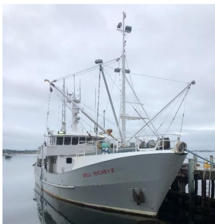
Figure 32. FV Del Richey 2, a Commonwealth Southern Squid Jig fishery vessel (20m aft wheelhouse vessel) (Source: Andrew Sullivan)
