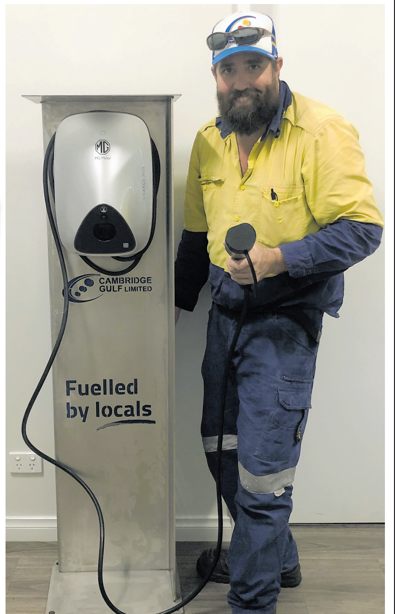
Cambridge Gulf Limited chief operating officer Mat Dear with one of their new 11kW, three-phase EV chargers.
