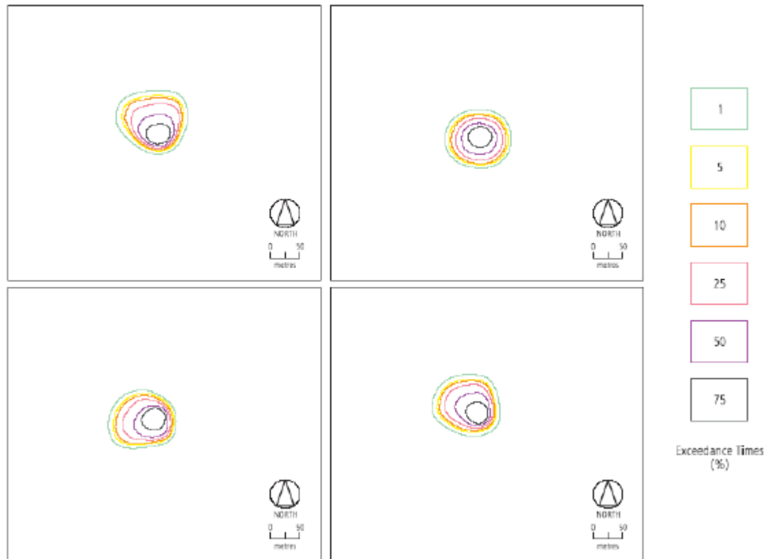
Figure 6-5: Predicted dispersion and temperature of cooling water discharge trajectory and dispersion of cooling water modelled for a nominal discharge of 100,000 m 3 at a water temperature of 25°C above surrounding seawater
