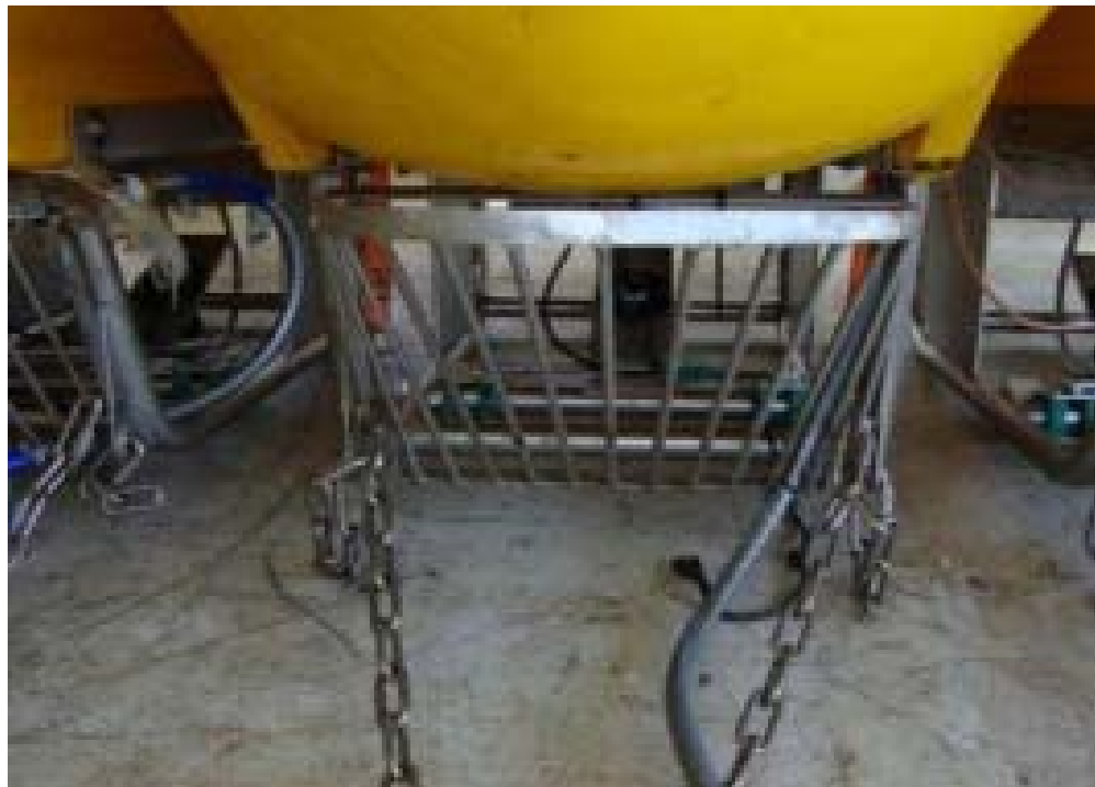
Figure 3-1: Turtle Guards Fitted to Tail Buoys
