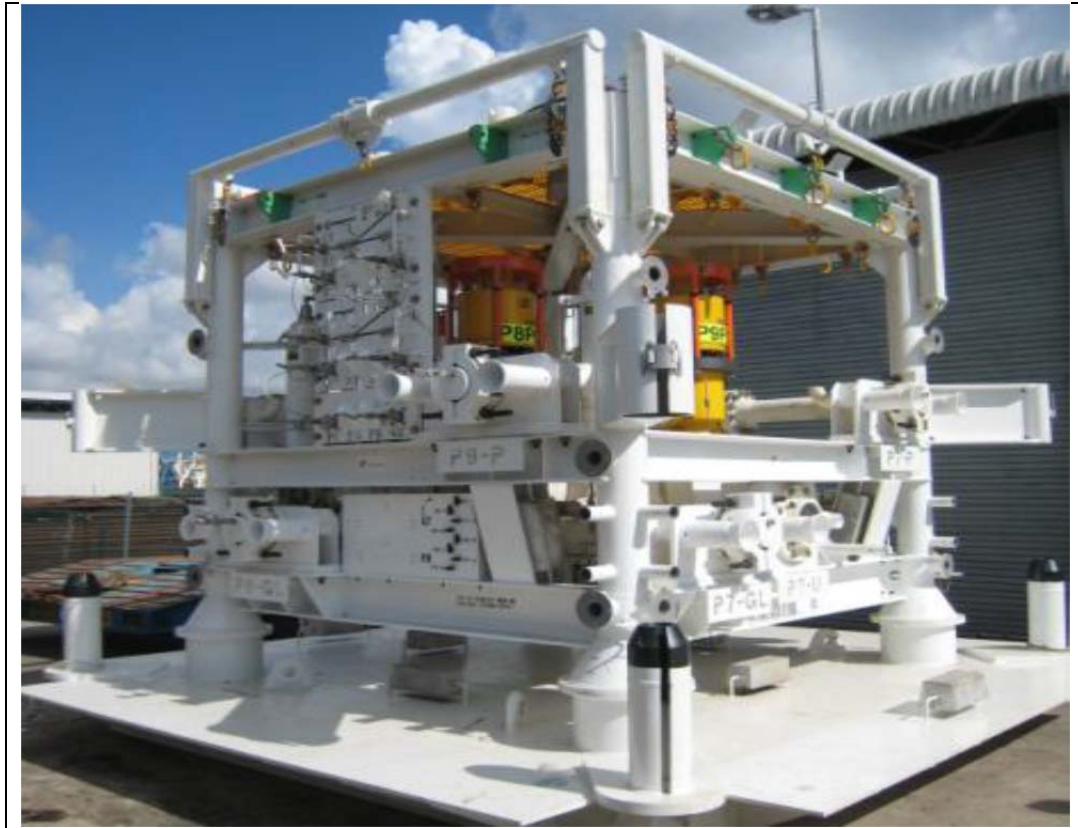
Photo 1. Puffin manifold and foundation structure
