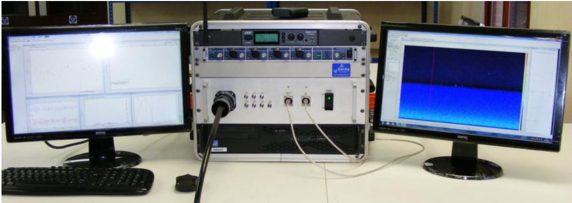
Figure 1. 8U Base unit with Rack-mounted PC and LF and HF monitors
