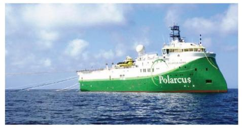
Figure 3-5: Polarcus Asima Seismic Survey Vessel
