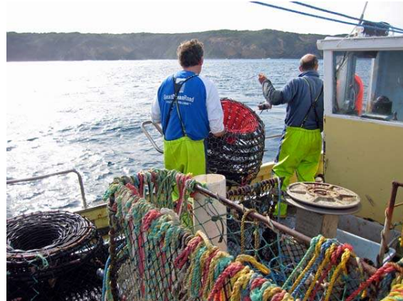
Figure 12 Photos showing (a) close up of cray pots, and (b) the retrieval of cray pots using the pot hauler.
