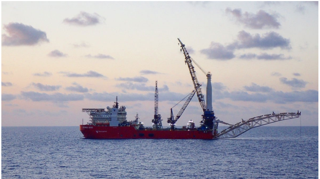
Figure 3-2: Indicative pipeline installation vessel
